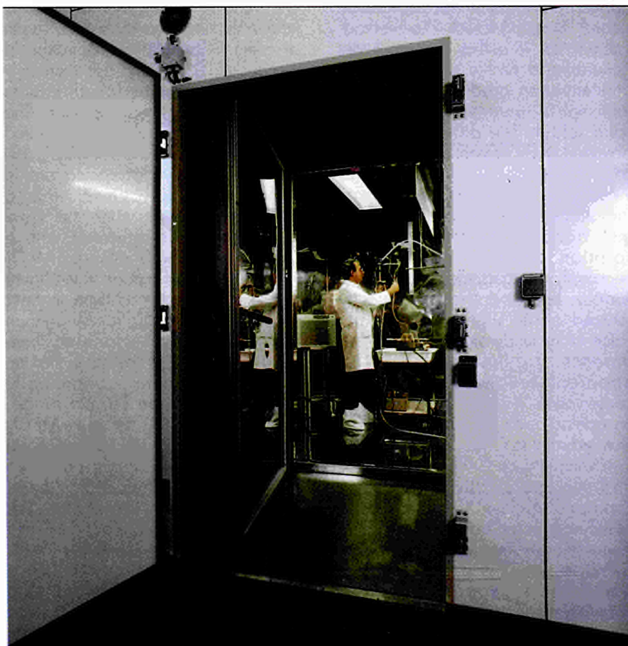
Fig.1.38 View into the interior of a double-walled walk-in type environmental chamber ("Indoortron") where the testing of an air cleaning device is under preparation.
