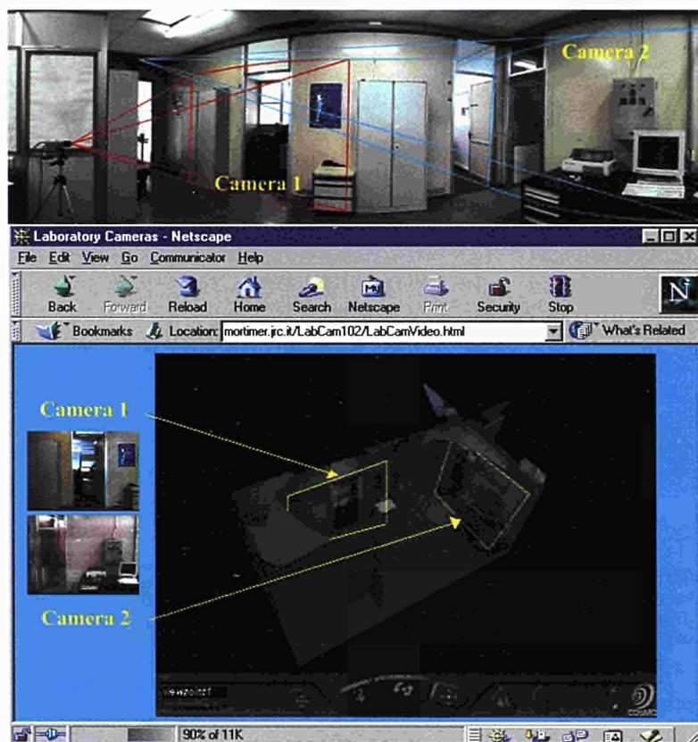
Figure 3.9: Multi-Camera Surveillance – Pilot implementation using two cameras. The 3D model of the surveyed environment is overlaid with the real-time video surveillance images. This provides spatial context for an easier interpretation.
