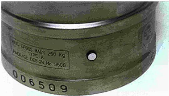
A new multipurpose passive radio-frequency transponder [3.8,3.9] seal (Figure 3.7) was developed and patented (International Patent no. 99402256.4). This new passive seal uses the same installation principle as the well-known Copper Brass (i.e. wire needed). Using a portable radio-frequency reader, it is now possible to read the two identification numbers inside the seal
