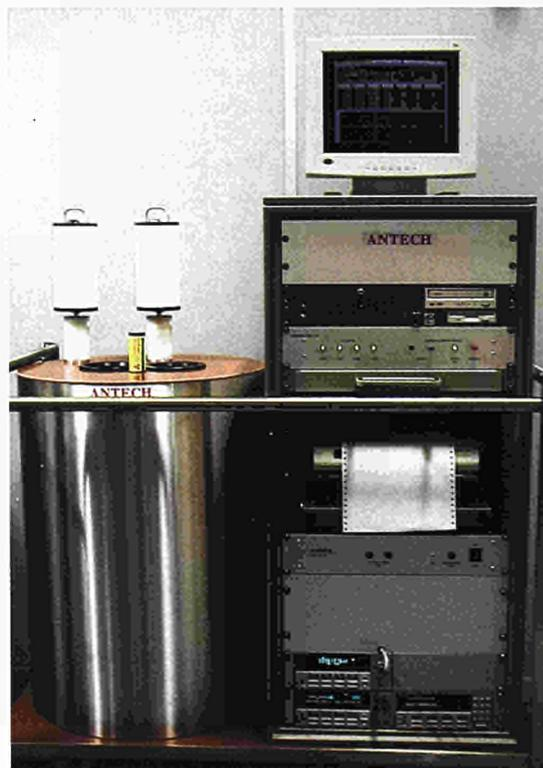
Figure 3.3: The new Small Sample Calorimeter (SSCAL) allows the characterisation of samples as small as 1g of plutonium at 0.2% precision.
