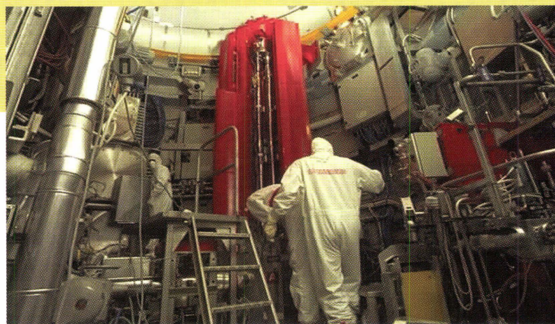
View of the interior of the caisson used in the Phébus FP programme, which contains elements simulating the cooling circuit of a damaged nuclear reactor.
