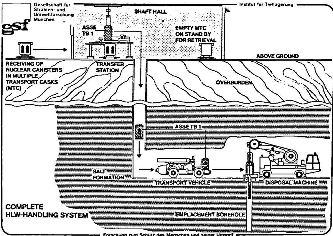
Fig. 2: HAW Handling System
