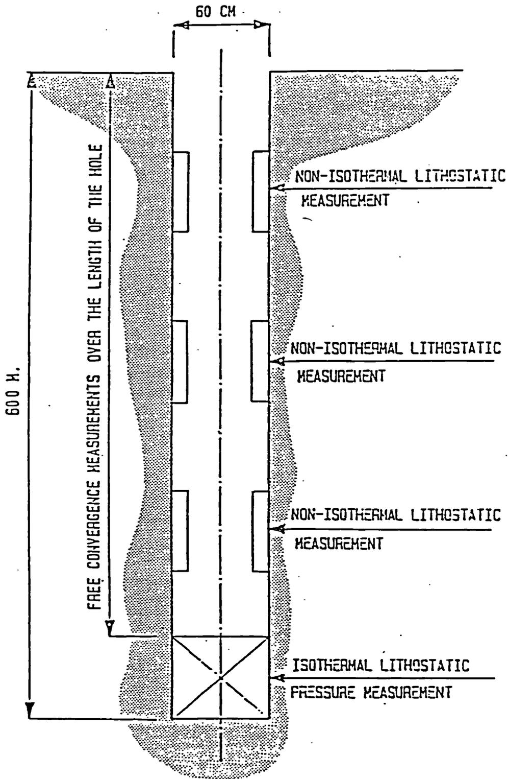
Fig. 1 : Sketch of the 600 m bore hole measurement set up.
