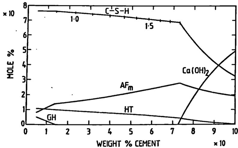
Fig. 2. Phase distribution in slag-cements
