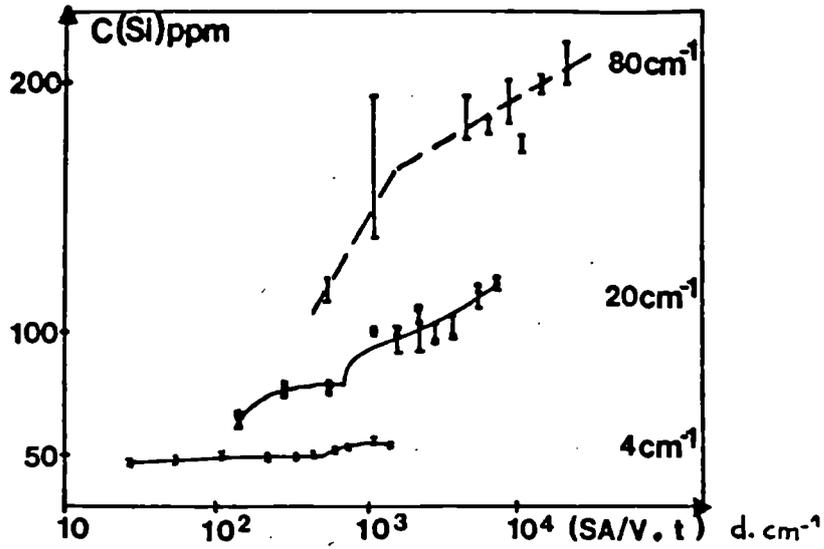
FIGURE 1 : SILICON CONCENTRATION VERSUS (SA/V.t) FOR DIFFERENT SA/V RATIOS (2nd TEST SERIES)
