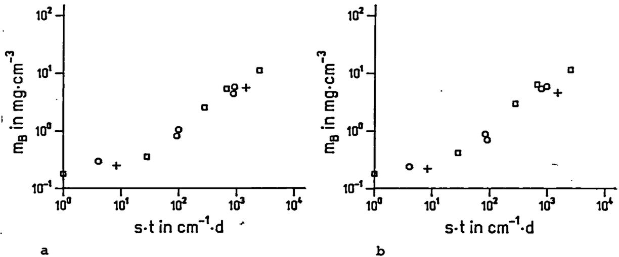
Figure 3. Amount of reacted glass per leachant volume,  $m_B$  (determined by boron analysis of leachate) as a function of  $s \cdot t$  for the corrosion of the HLW glass SON 68 in solution 1 (a) and solution 2 (b) at 190 °C;  $\square$  : 30 d;  $\circ$  : 120 d; + : HMI test
