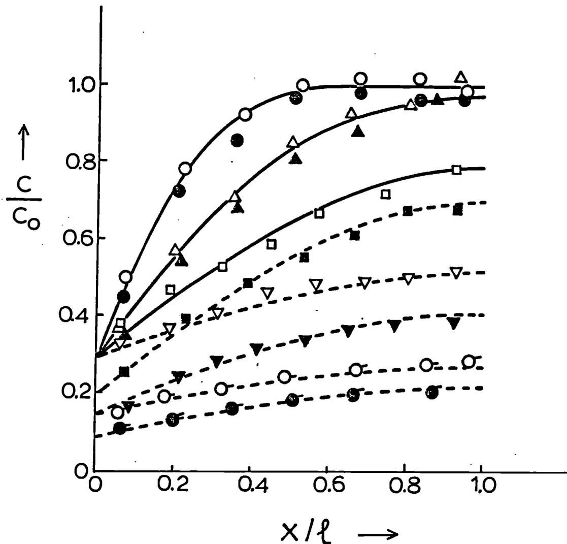
Figure 2. Distribution of Cs in cement samples after 6 (o,●), 21 (Δ,▲), 57 (□,■), 114 (▽,▼) or 174 (◇,◇) days of elution at 70°C. Amounts eluted (%): 10.2 (o), 11.5 (●), 22.1 (Δ), 24.0 (▲), 37.1 (□), 45.0 (■), 54.5 (▽), 65.0 (▼), 76.0 (◇) or 82.0 (◇). The theoretical concentration profiles correspond to  $D=7.5 \times 10^{-7} \text{ cm}^2 \text{ s}^{-1}$  (—) or  $8.9 \times 10^{-7} \text{ cm}^2 \text{ s}^{-1}$  (---) and  $C_1/C_0=0.30$  (o,●,Δ,▲,□,▽), 0.20 (■), 0.15 (▼,◇), 0.09 (◇).
