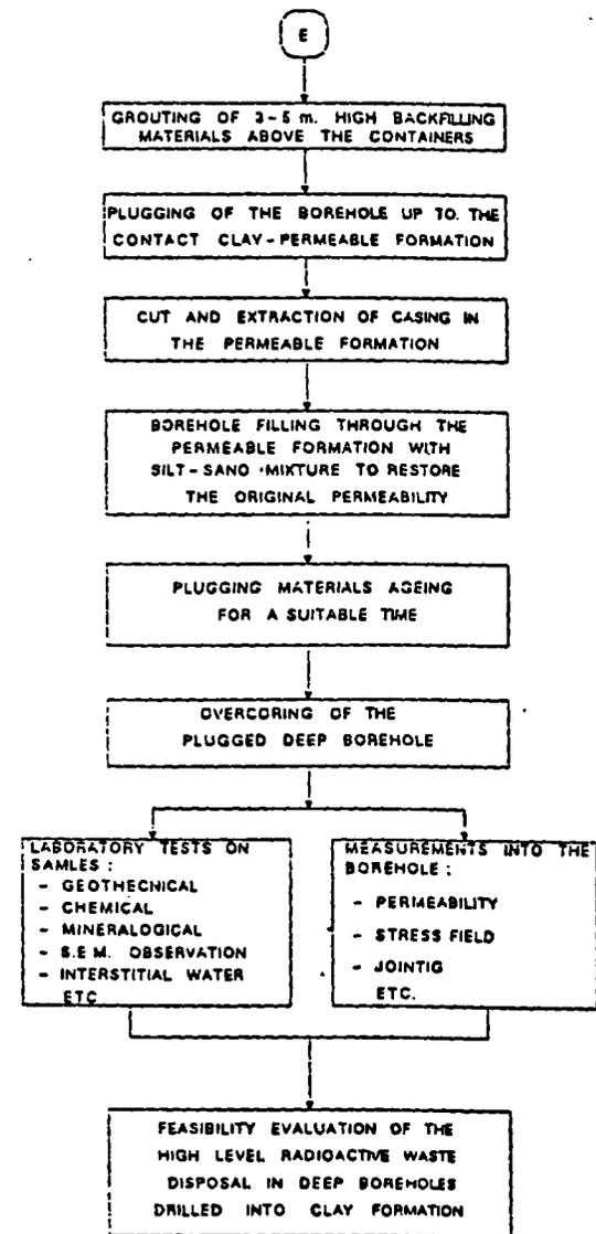
TRIALS AND CONTROL OF PLACING FILLING AND SEALING MATERIALS
