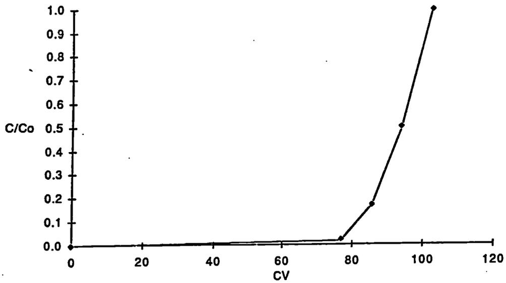
Fig.3 IE-96 Zeolite break-through curve
