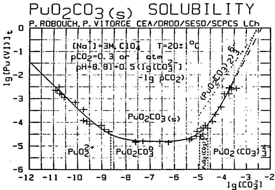
Fig. 2 : Solubility of plutonium ( $NaClO_4$  3M,  $t = 25^\circ C$ ) ; note the potential existence of a trimer specie at high free carbonate concentration (dashed line)
