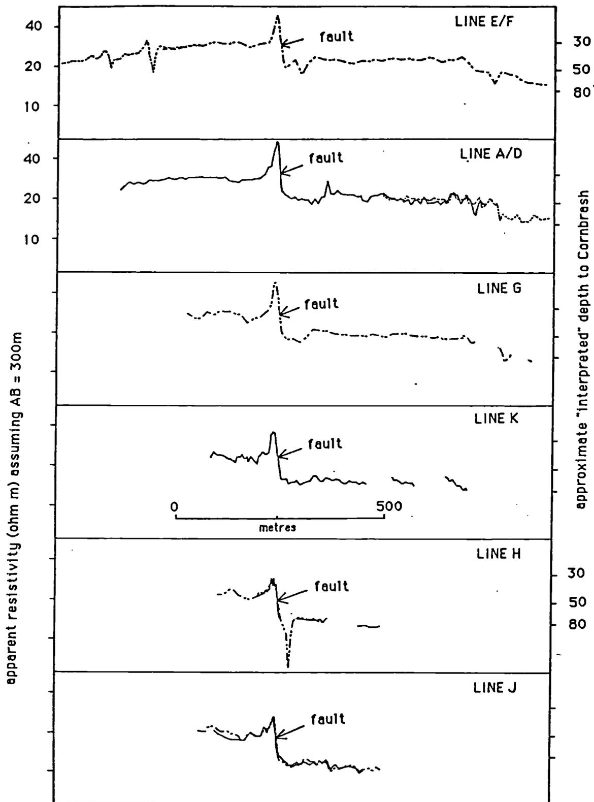
Figure 2. Resistivity profiles across the presumed fault
