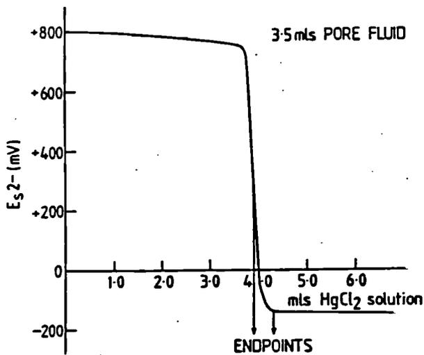
Titration of 80d. old 85% EPS-15%PC pore fluid with  $10^{-2} \text{M HgCl}_2$ .
