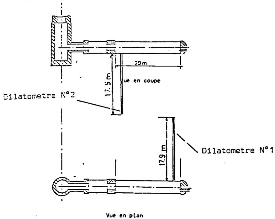
Fig. 1 : SITUATION OF THE DILATOMETER CREEP TEST
