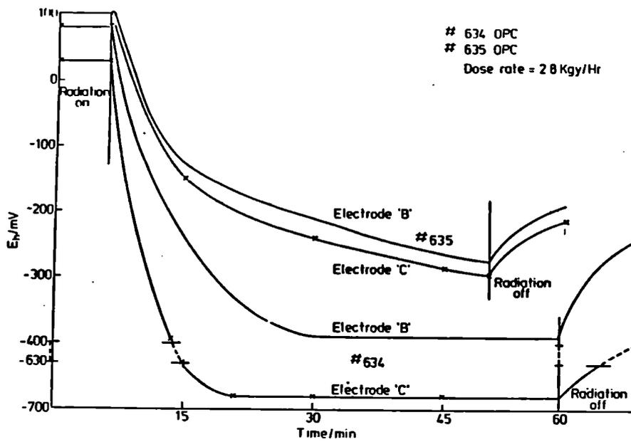
Fig. 10.  $E_h$  variations with irradiation does for OPC pastes.
