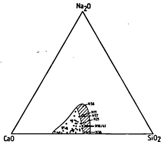
Fig. 4. Anhydrous compositions of representative  $\text{Na}_2\text{O}-\text{CaO}-\text{SiO}_2-\text{H}_2\text{O}$  gels aged up to 182 days.
