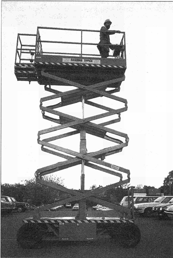
Figure 2: Personnel lift of the scissors type incorporating Burnside hydraulic cylinders.
