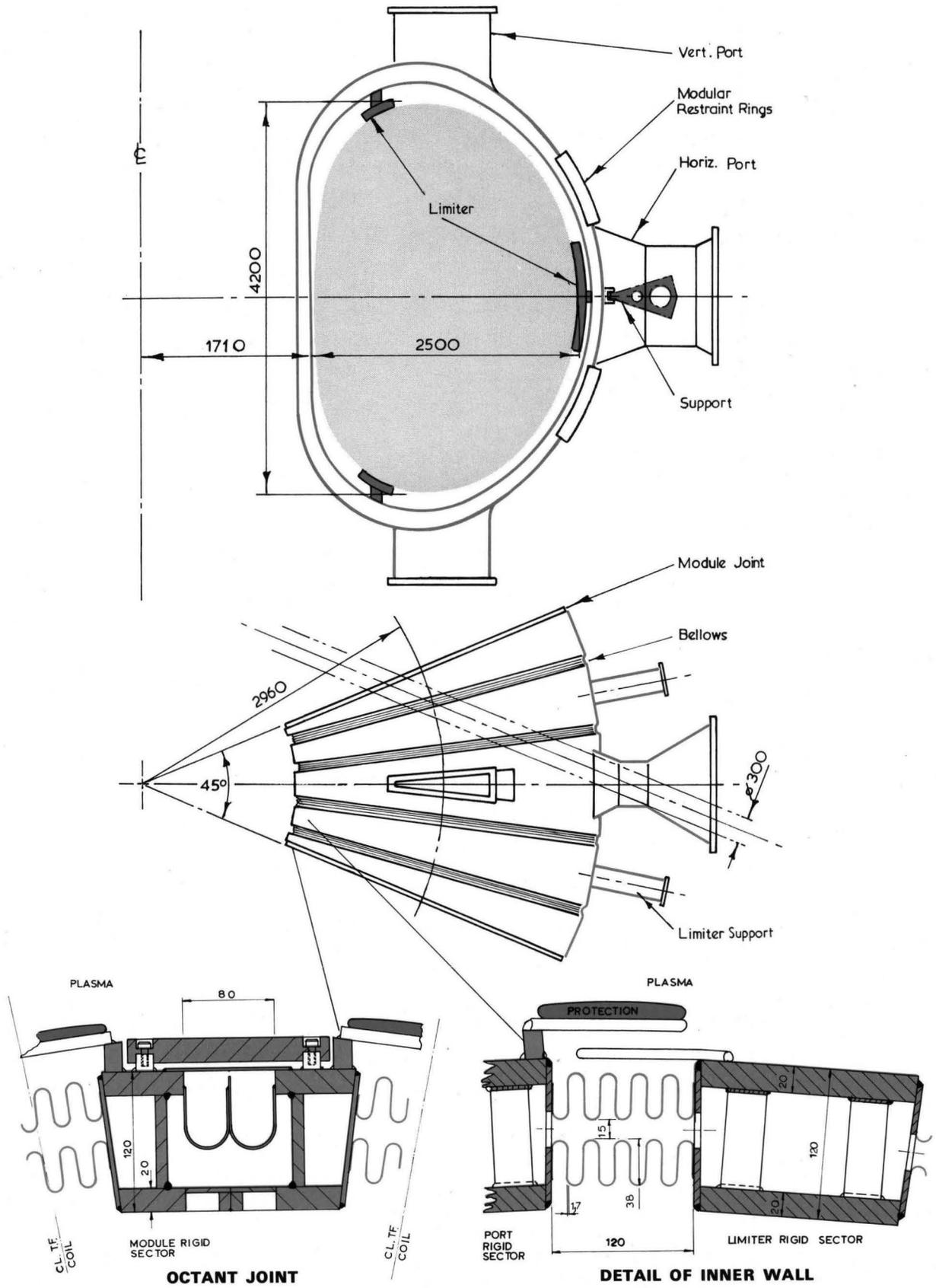
General Lay-Out of the Vacuum Vessel Octant
