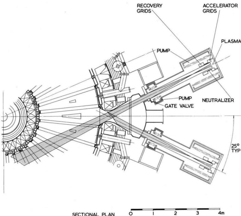
Installation with Six Injectors on a JET port
