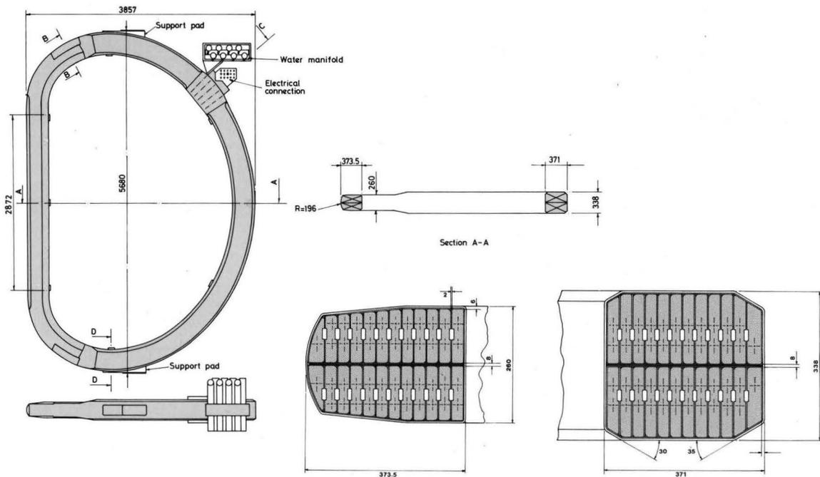
PARAMETERS OF ONE TOROIDAL FIELD COIL
