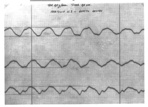
Cal. lg/mm - Timer O.l sec. HAMMER No. 1 - left elbow
