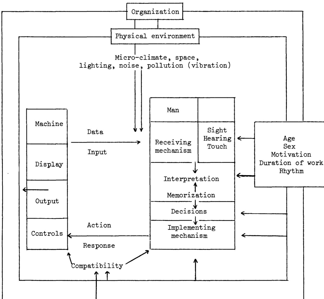
The above diagram shows the working model used by us in our research. It should be noted that the man-machine system must be interpreted not only in relation to the wider physical environment but also to the man-man system which is equally important in the case of the workplaces studied by us because of the highly responsible nature of the drivers' duties and the complex organization involved.
