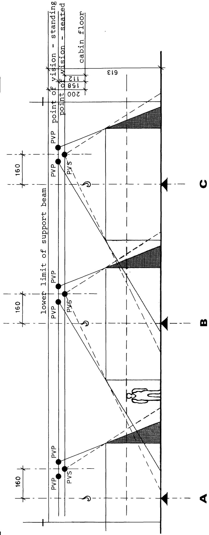
ZONES VISIBLE AND INVISIBLE DURING OPERATIONS AT A (MOBILE STORAGE UNIT), B AND C ( FIXED STORAGE UNITS°.
