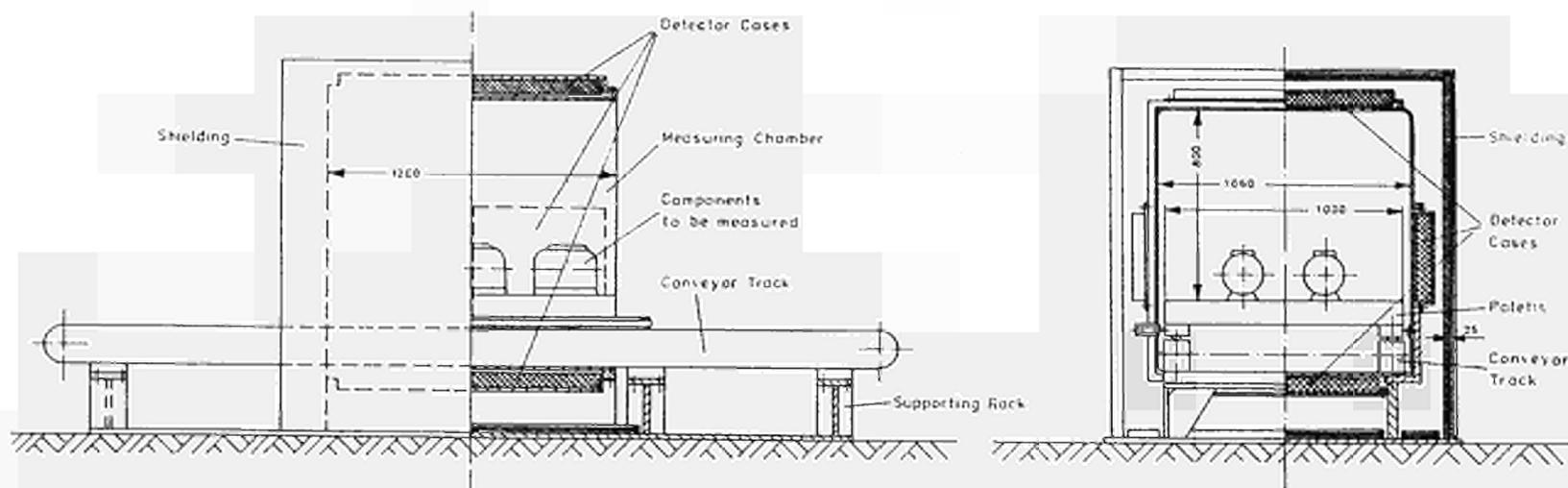
Figure 1 : Preliminary Layout of Measuring Device
