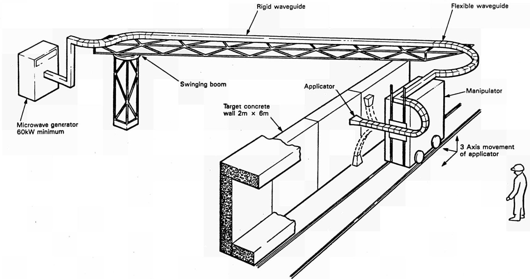
Figure 3: Proposal for prototype machine
