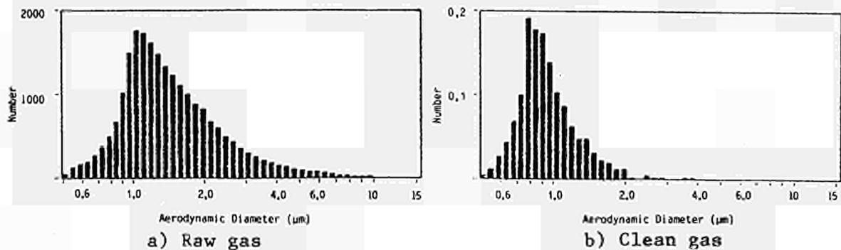
Figure 2: Histogram of particle size distribution (wire brush)
