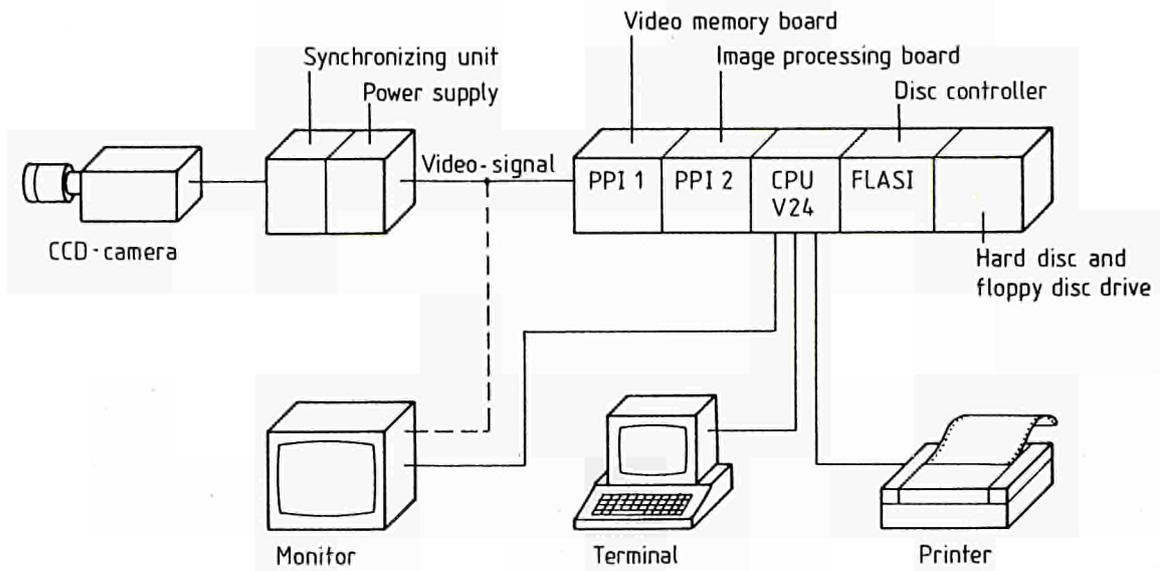
Fig. 1: Block Diagram of the Image Processing System with CCD-Camera
