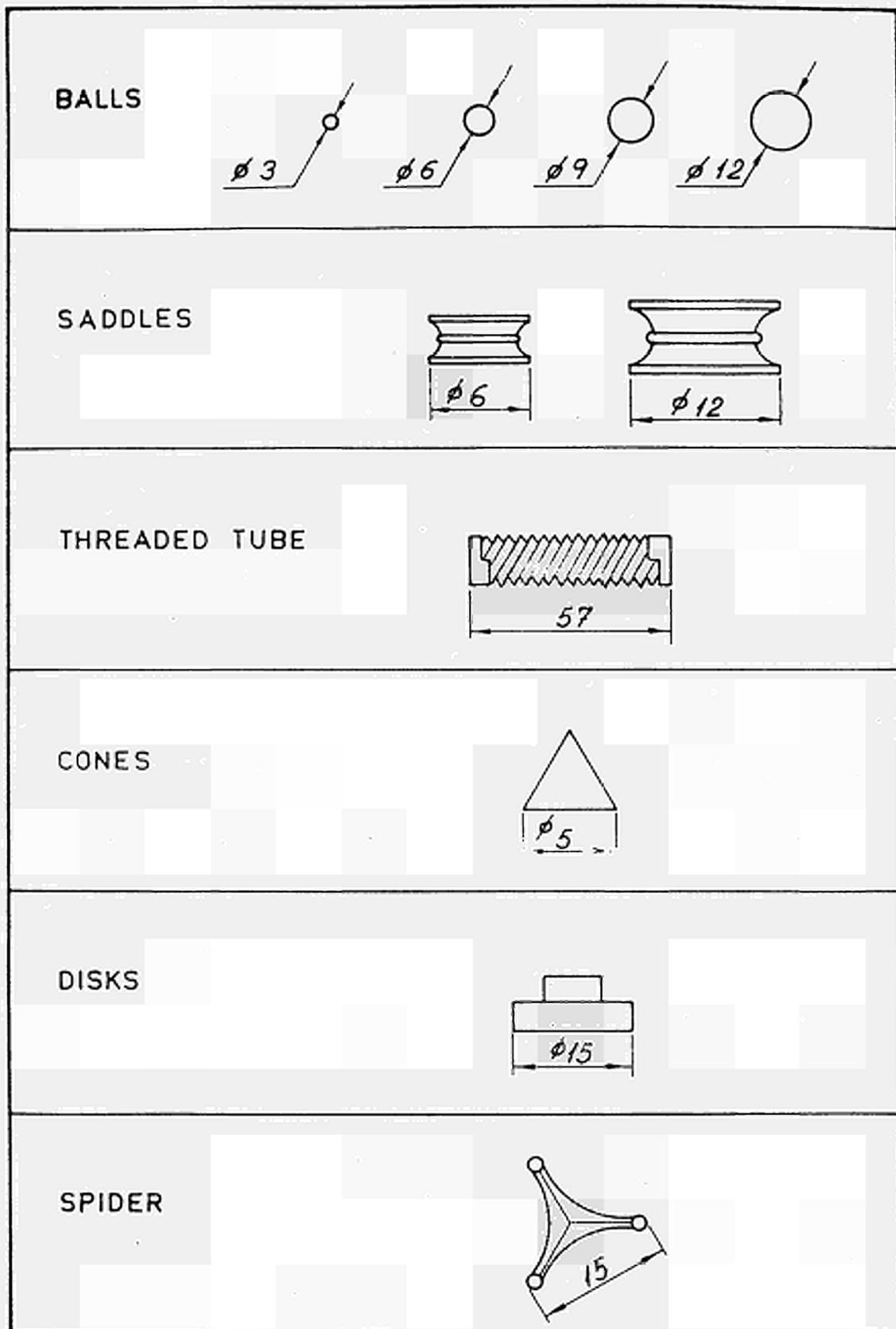
Figure 3: Abrasives of different sizes and geometries
