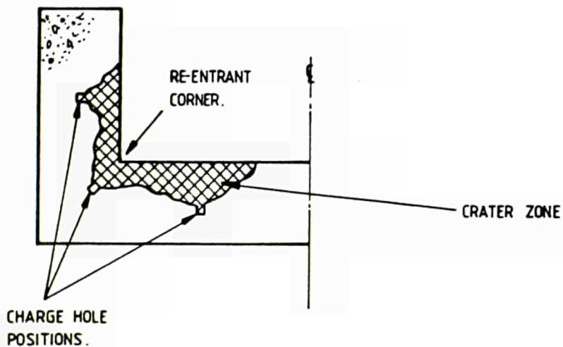
Fig. 2. Section showing removal of concrete from a re-entrant corner.
