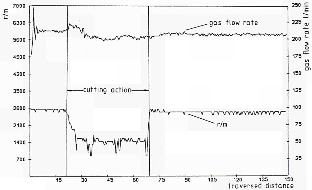
Fig. 6: Gas Flow Rate and Rotation Speed during Underwater Cutting
