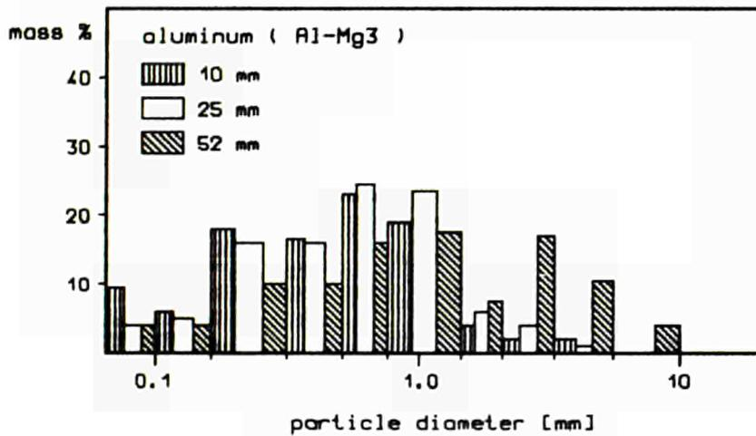
Fig. 2: Sieve size analysis of the settled kerf material
