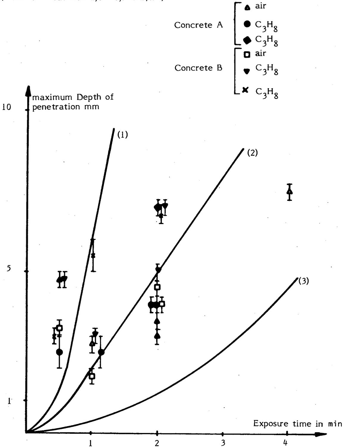
Figure 2: Erosion depth as a function of the thermal exposure time
