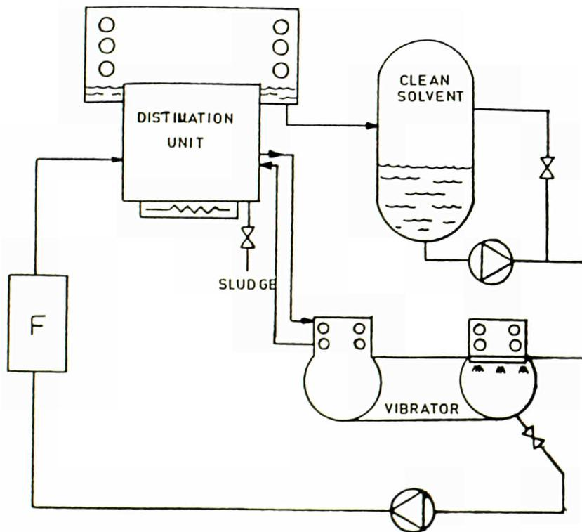
Figure 2: Vibratory decontamination system
