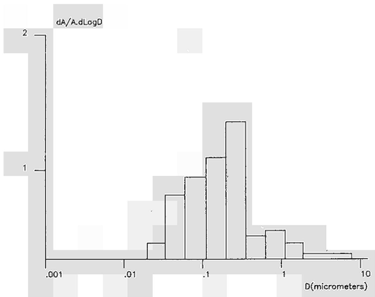
Figure 4: Radioactivity ( $^{137}\text{Cs}$ ) distribution in size range of aerosols produced by underwater plasma torch cutting of RAPSODIE plates
