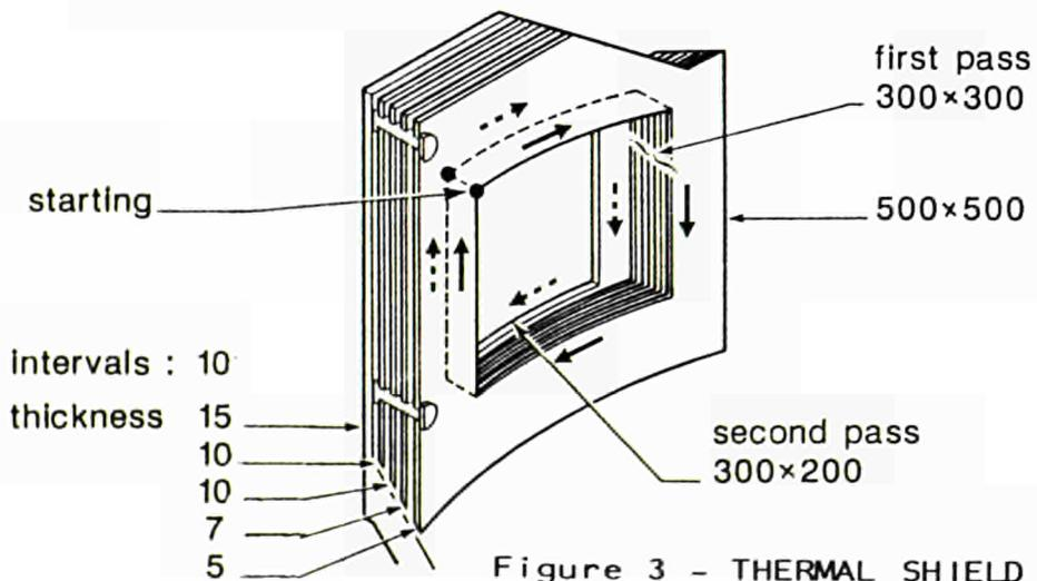
Figure 3 - THERMAL SHIELD ASSEMBLY
