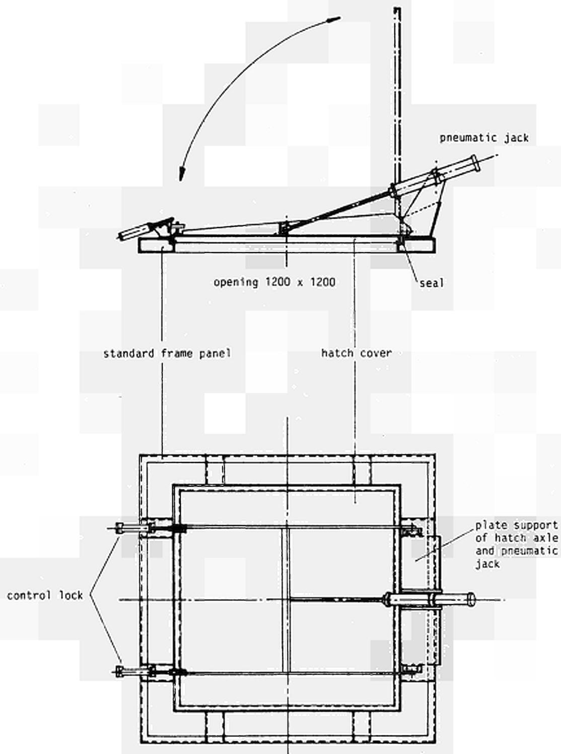
Figure 1. Swivelling panel
