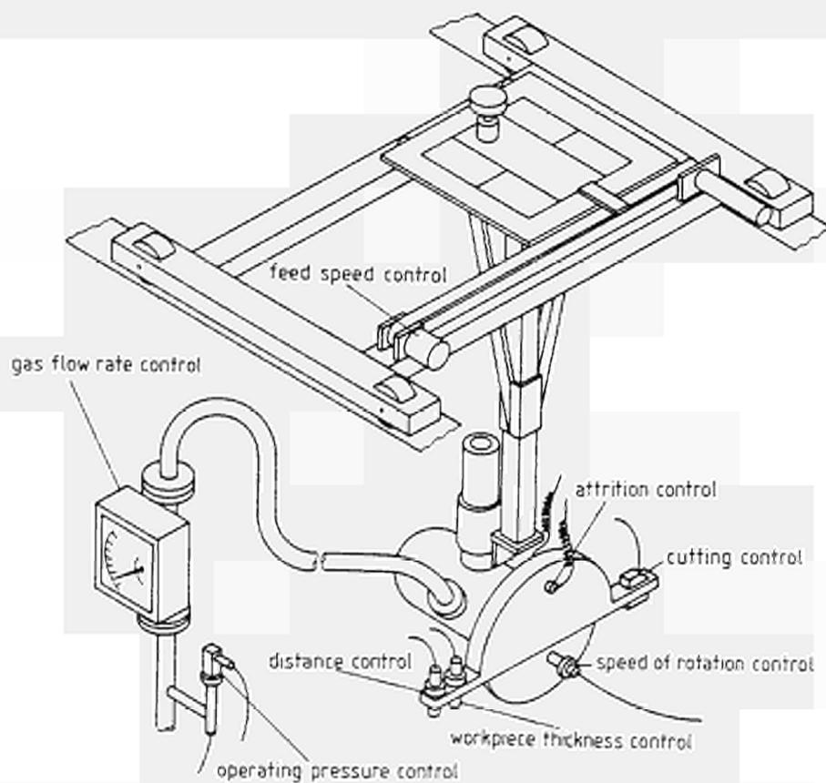
Fig. 4: Sensor Attachment for the Abrasive-Wheel Cutting-Off Process Underwater
