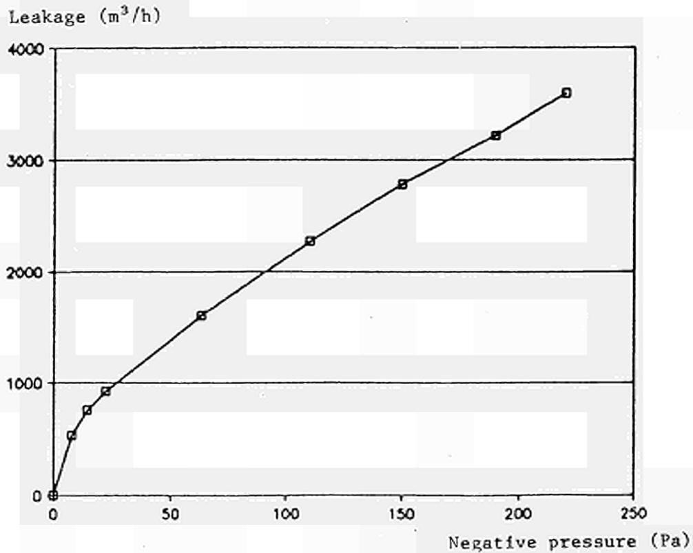
Figure 4: Leakage of the safe enclosure area
