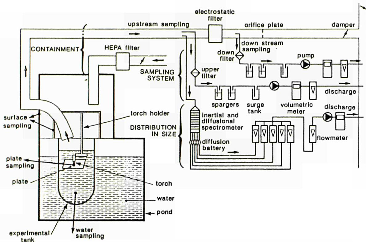
Figure 6 - DIAGRAM OF THE EXPERIMENTAL ASSEMBLY FOR AEROSOLS MEASUREMENTS
