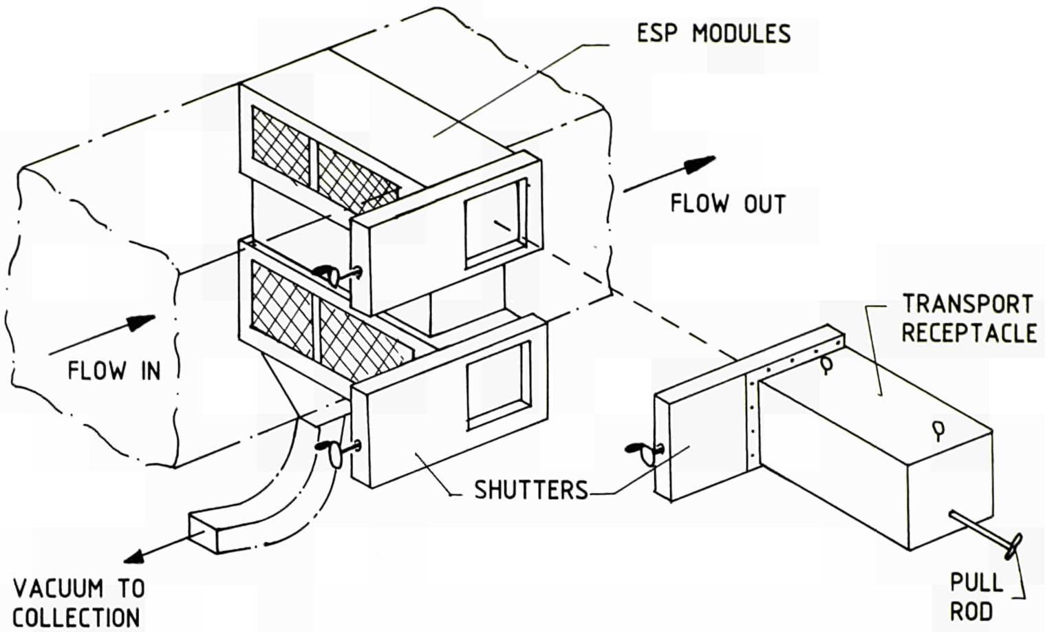
FIGURE 5: SCHEMATIC OF AN ESP FOR REMOTE HANDLING
