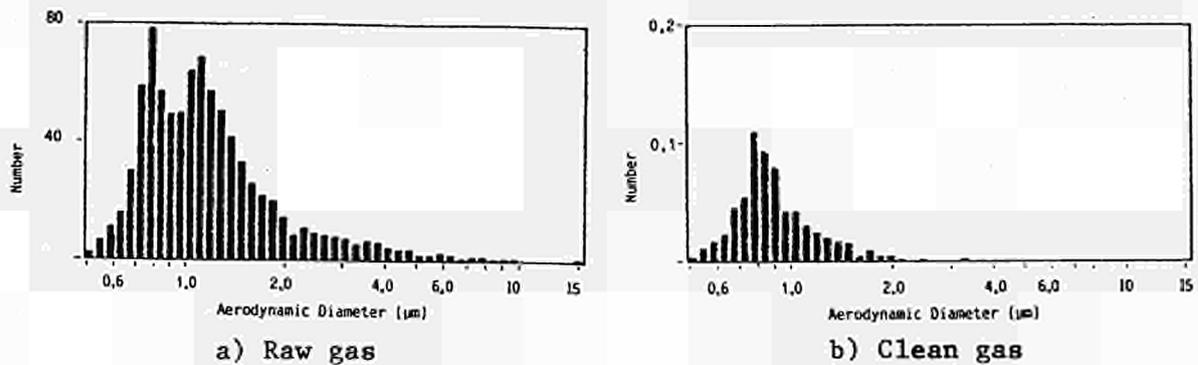
Figure 1: Histogram of particle size distribution (flame scarfing)
