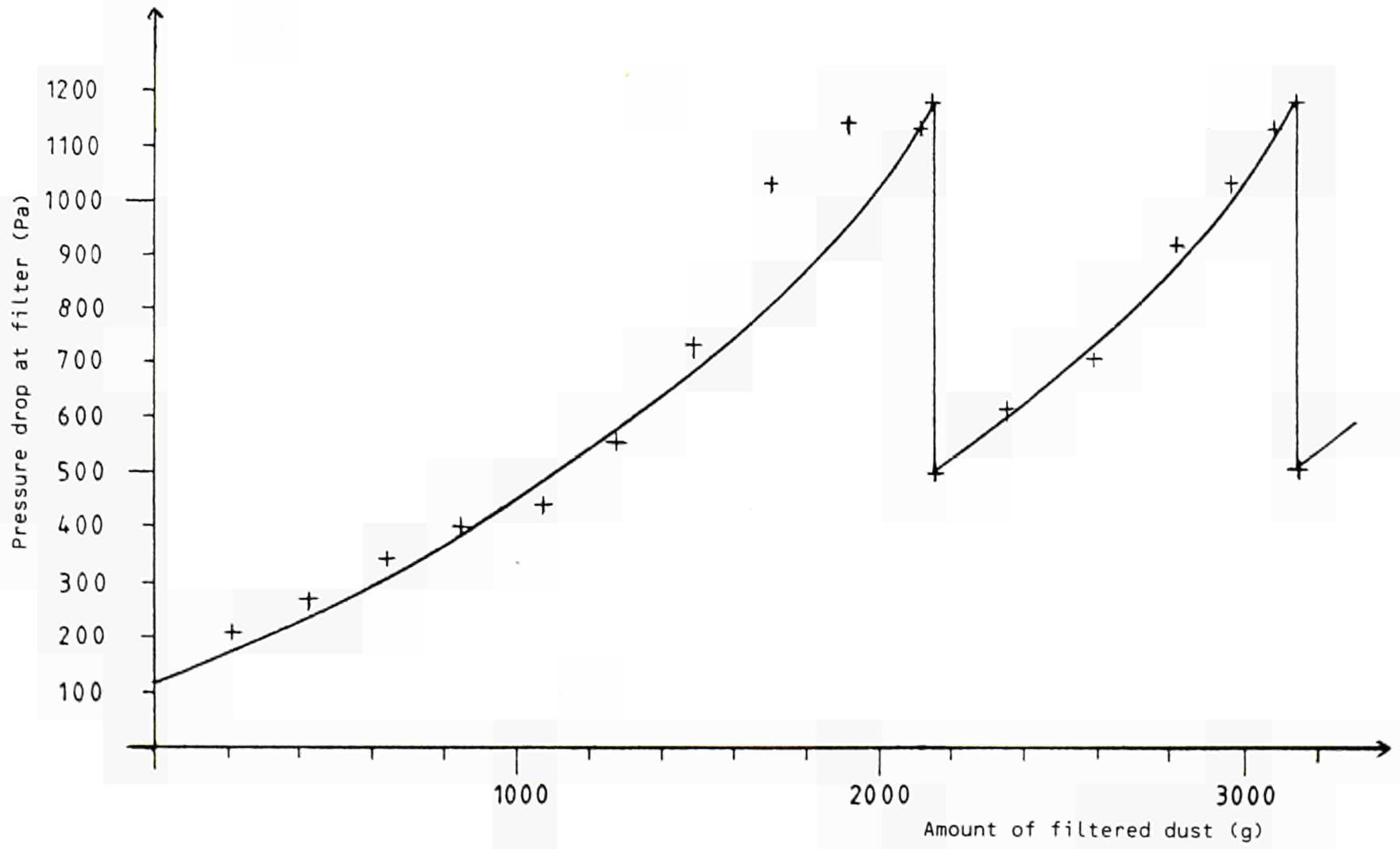
Figure 3 : Pressure drop at filter as a function of the amount of filtered dust
