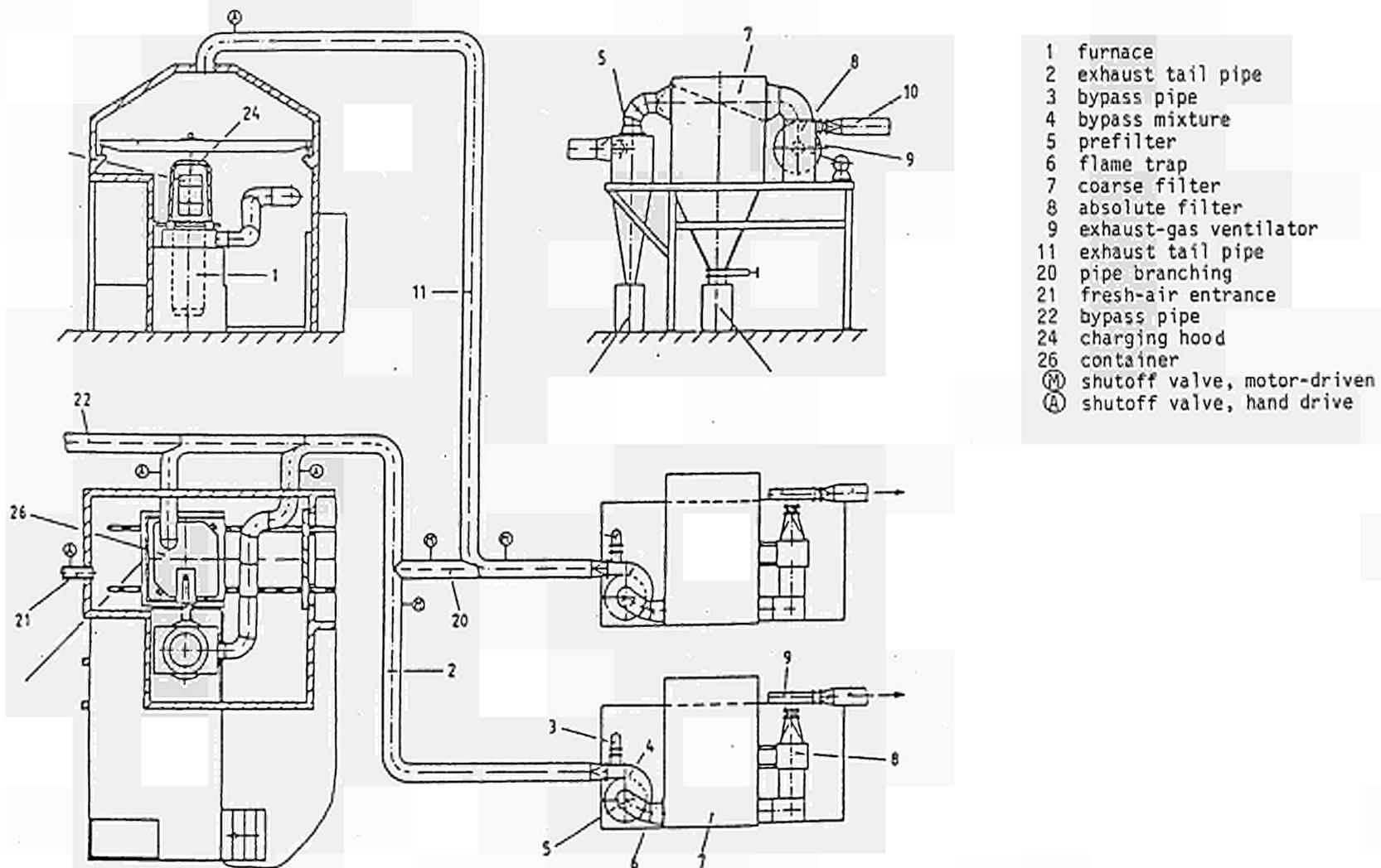
Fig. 2 Concept for the installation of a furnace at KRB A recommended by the companies GNS/Siempelkamp
