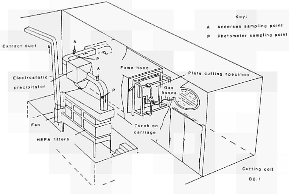
Figure 1: Flame cutting and fume generation rig
