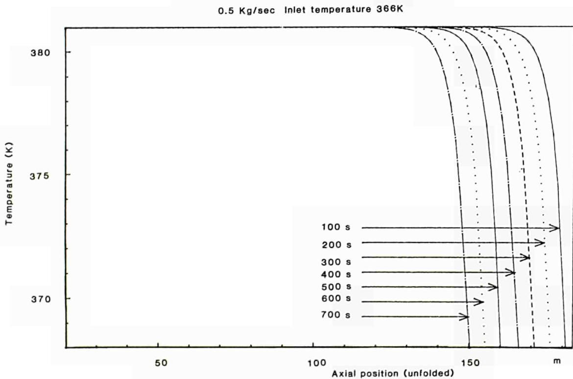
Figure 2. Movement of condensation zone
