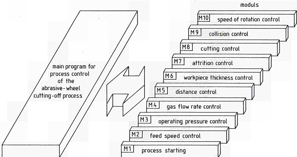
Fig. 2: Software Structure
