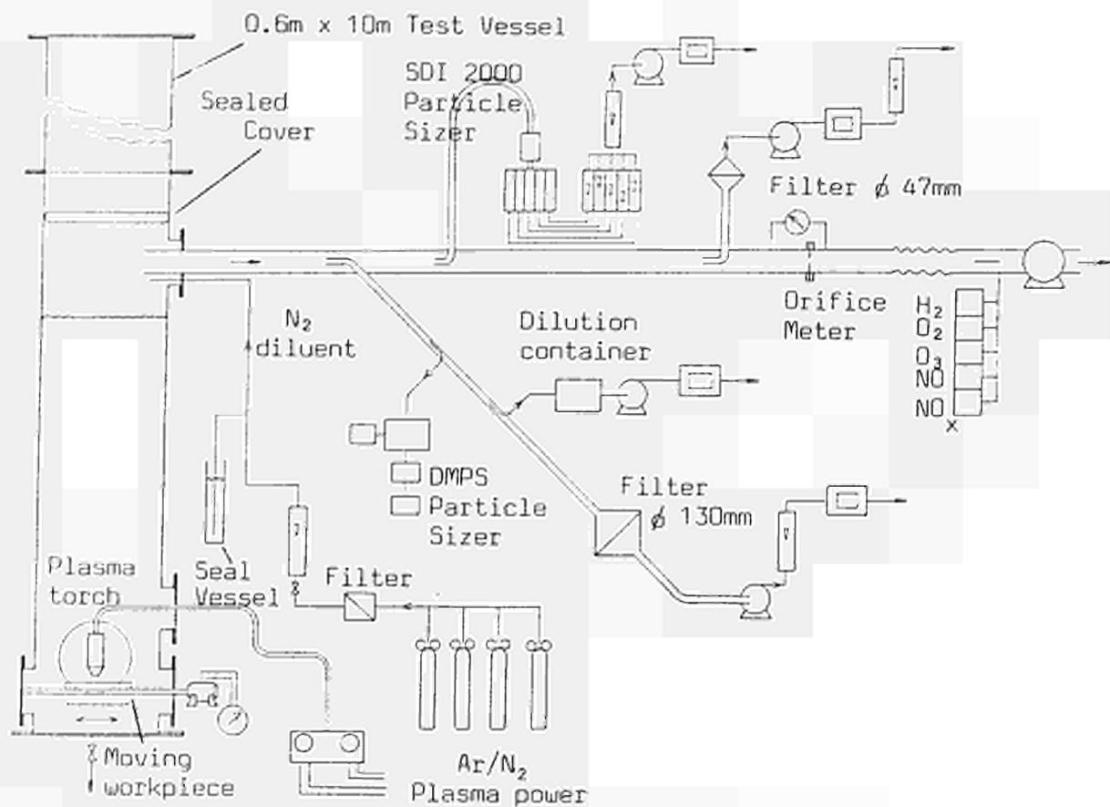
Figure 3. Sampling, fume and gas analysis instrumentation on deep water test vessel
