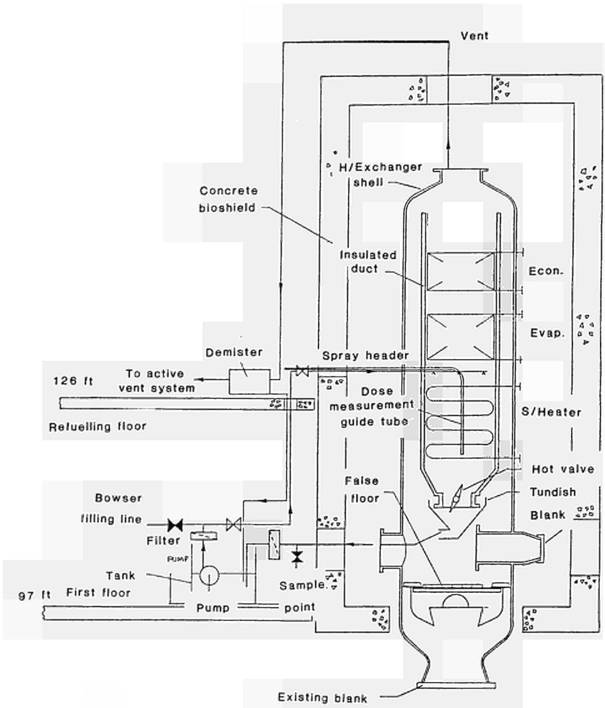
Figure 4. Heat exchanger decontamination
