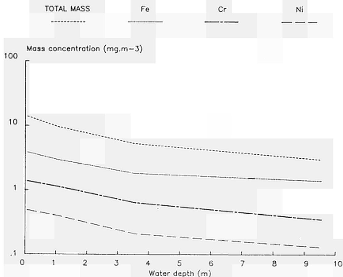
Figure 1: Influence of the water depth on aerosol mass concentration for underwater plasma torch cutting of stainless steel plate ( $e = 38 \text{ mm}$ )
