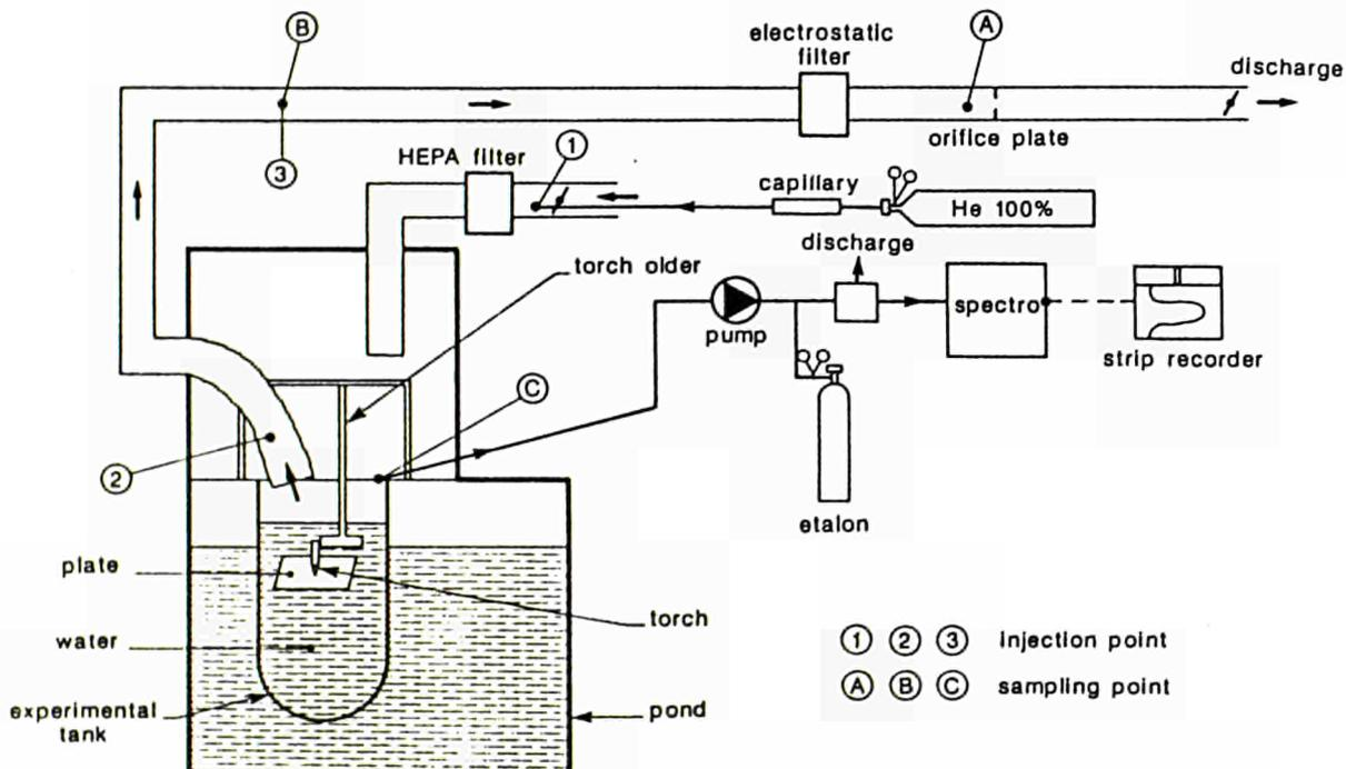
Figure 7 - DIAGRAM OF THE EXPERIMENTAL ASSEMBLY FOR HELIUM TRACER
