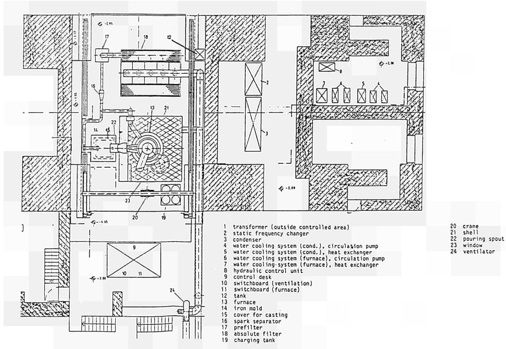
Fig. 1 Concept for the installation of a furnace at KRB A recommended by the company Noell, Würzburg
