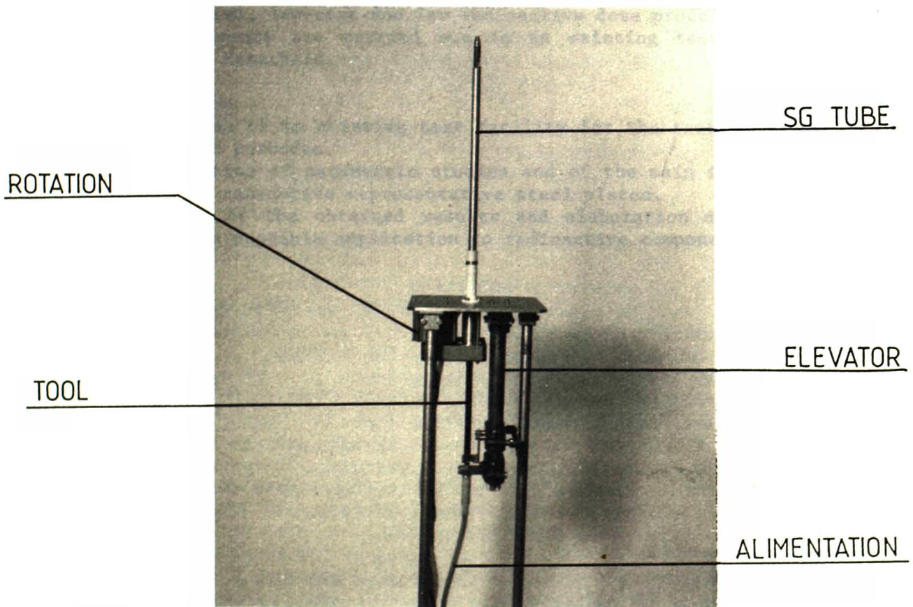
FIGURE 2 : Full scale testing bench for transversal cutting
