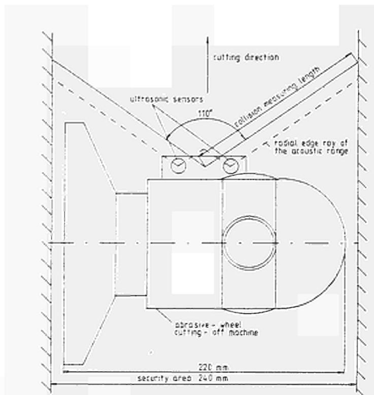
Fig. 3: Schematic Presentation of the Working Area of the US-Sensor
