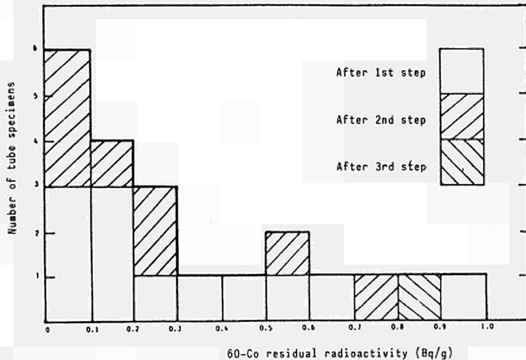
FIGURE 3 - Residual radioactivity of tube specimens at the end of 2<sup>nd</sup> in scale testing.
