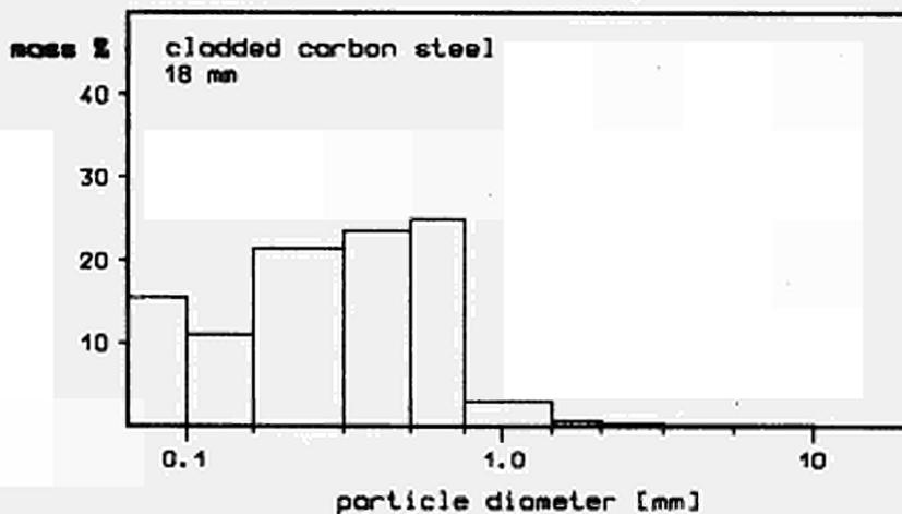
Fig. 1: Sieve analysis of the settled kerf material of cladmed carbon steel
