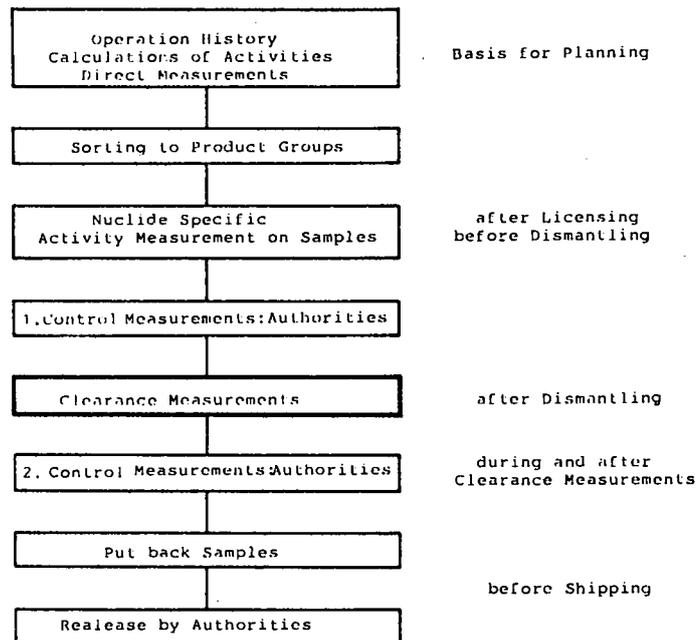
Figure 3: Release procedure KKN-Dismantling
