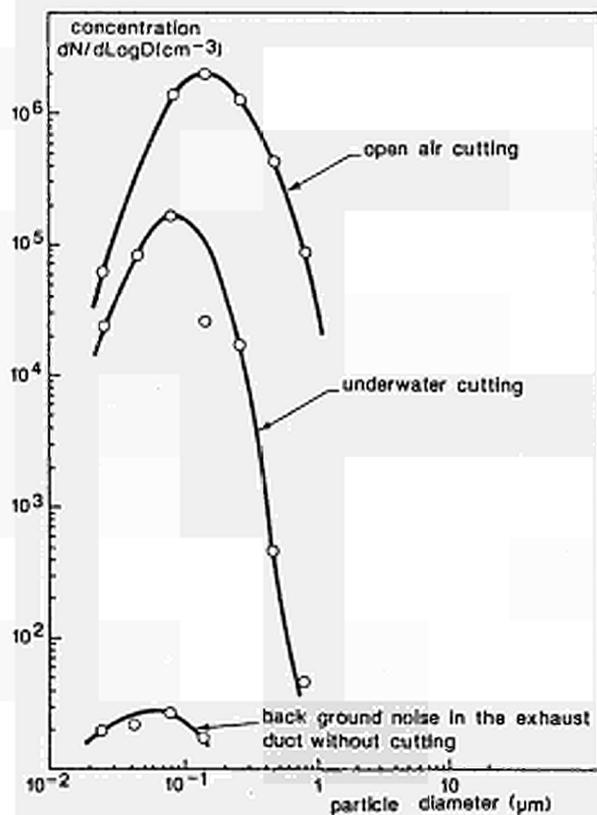
Figure 4 - GRANULOMETRIC DISTRIBUTION IN THE EXHAUST DUCT
