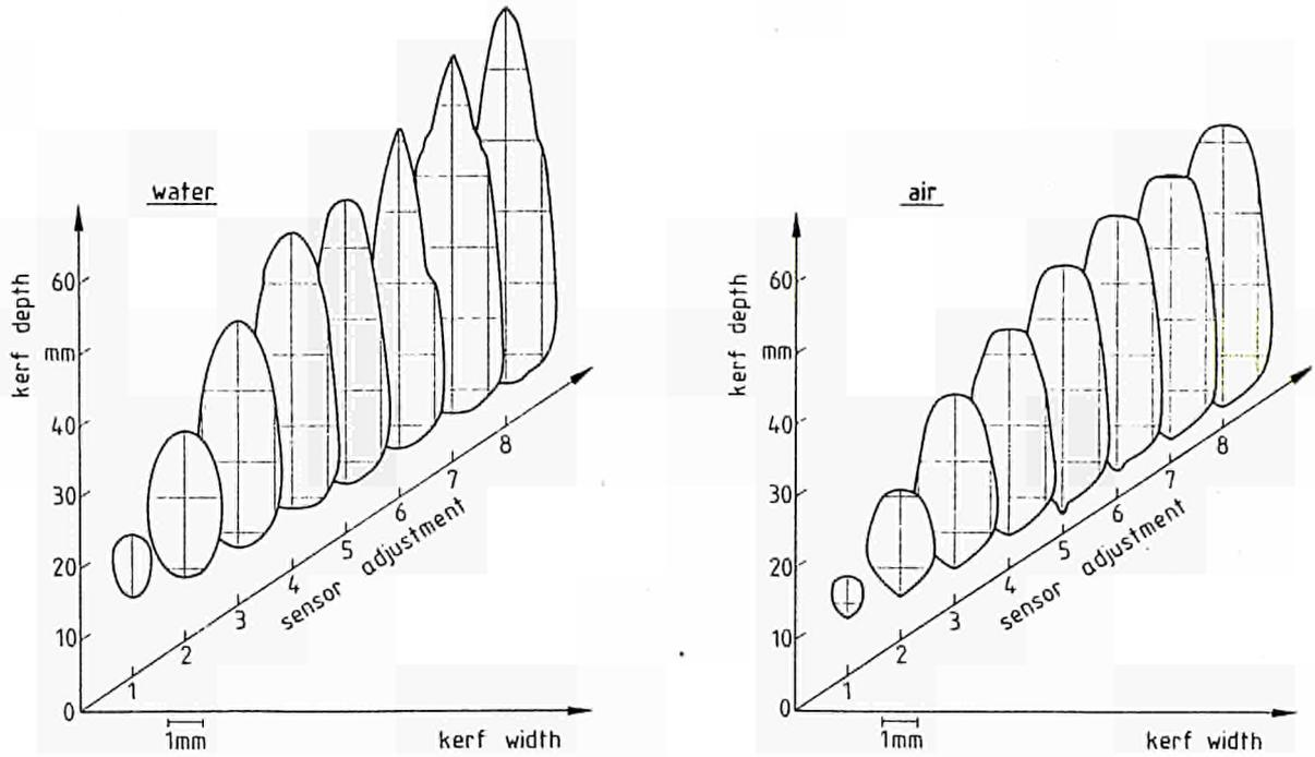
Fig. 5: Working Area of the Optical Sensor for Work Underwater and in Air
