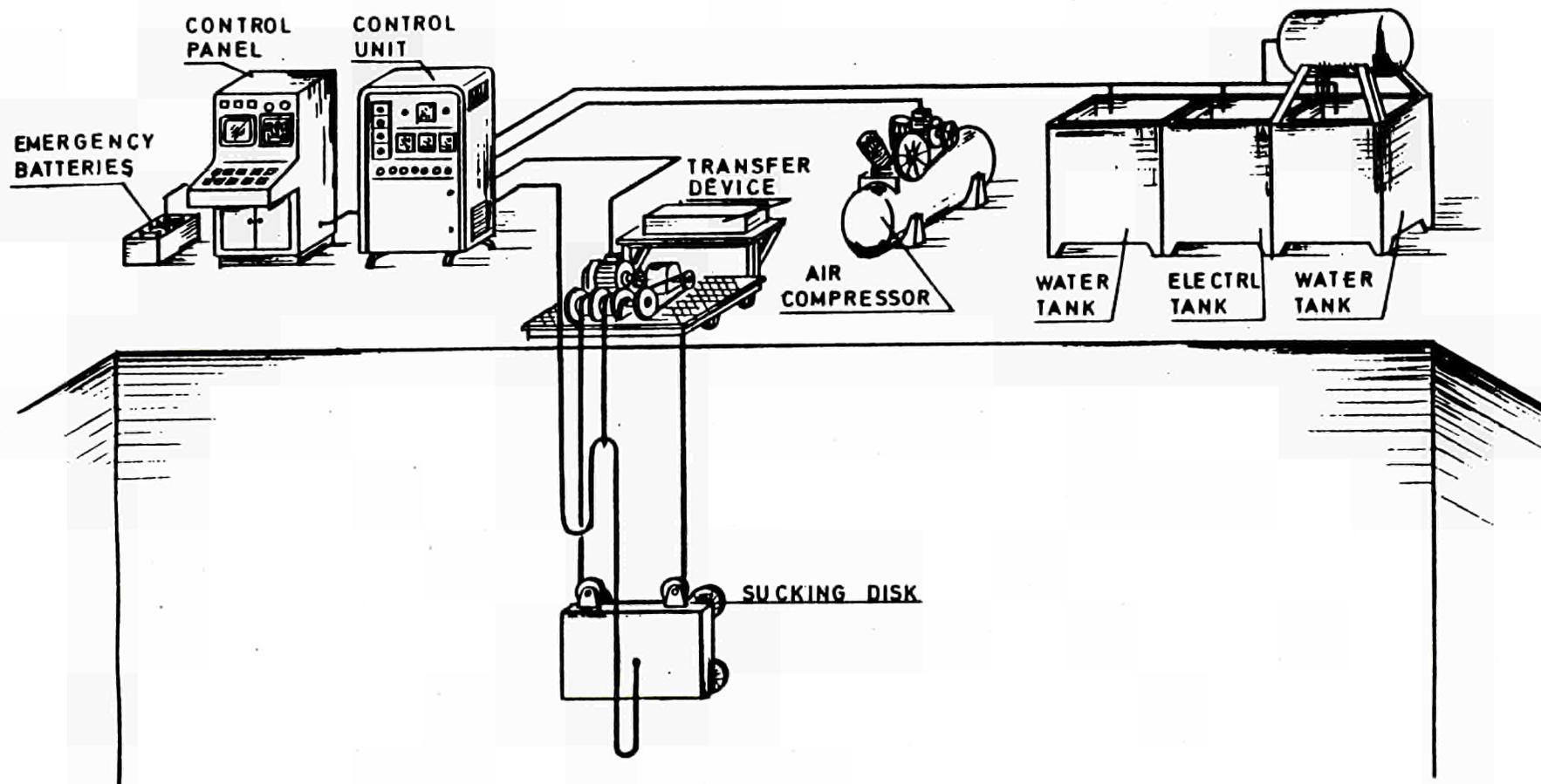
Figure 4 - Underwater Electropolishing System
