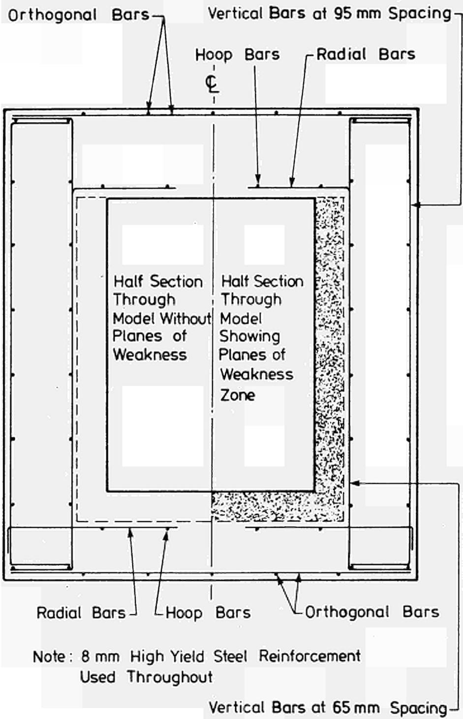
FIGURE 3 : REINFORCEMENT LAYOUT
