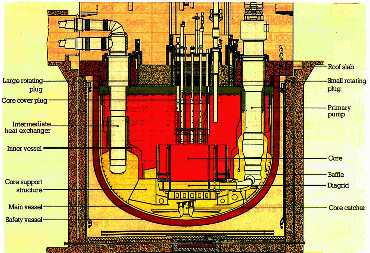
Figure 2: Fast breeder reactor block
