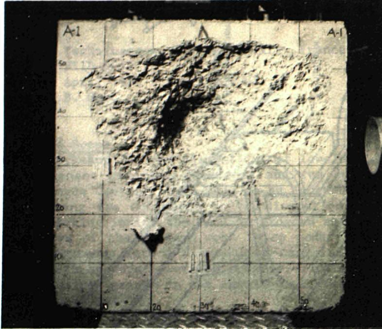
Figure 1: Damage to concrete block after first attack
