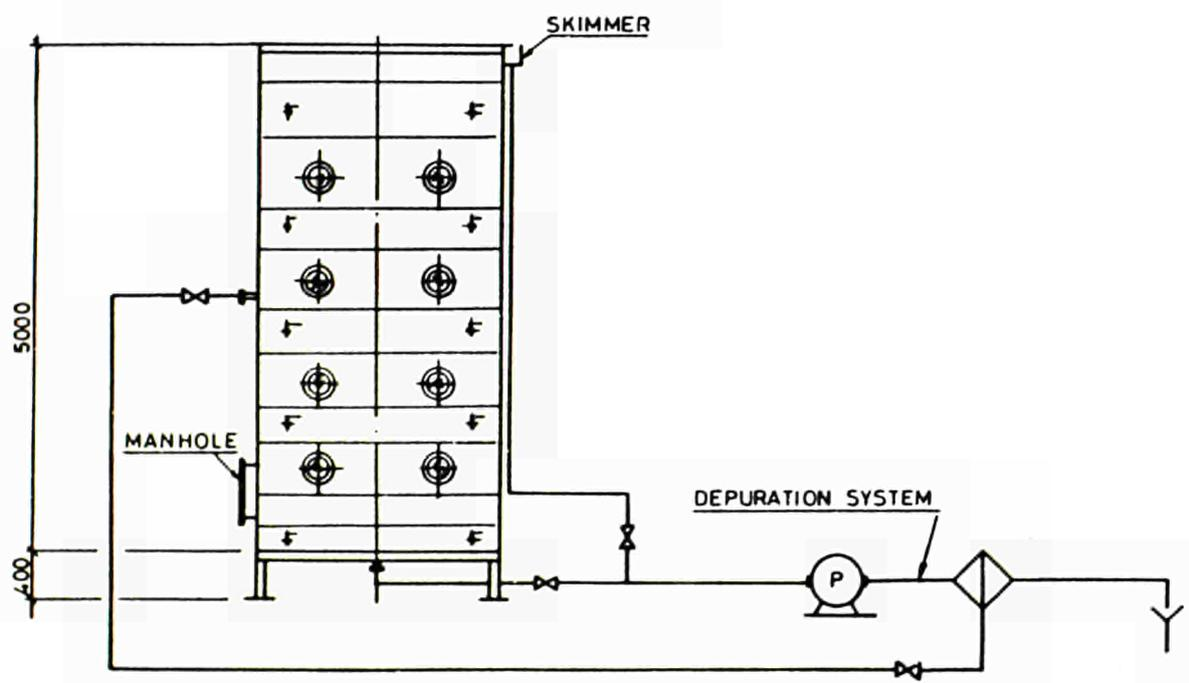
Figure 3 - Pool for underwater testing
