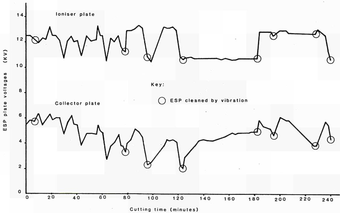
Figure 4. Changes in the ESP plate voltages with dust build-up
