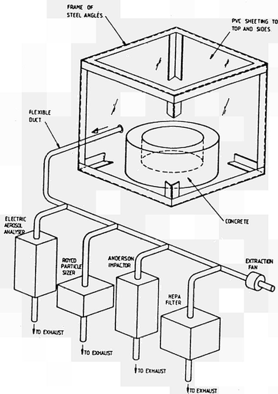
Fig. 3. Sketch of test set-up for particle size distribution analysis.
