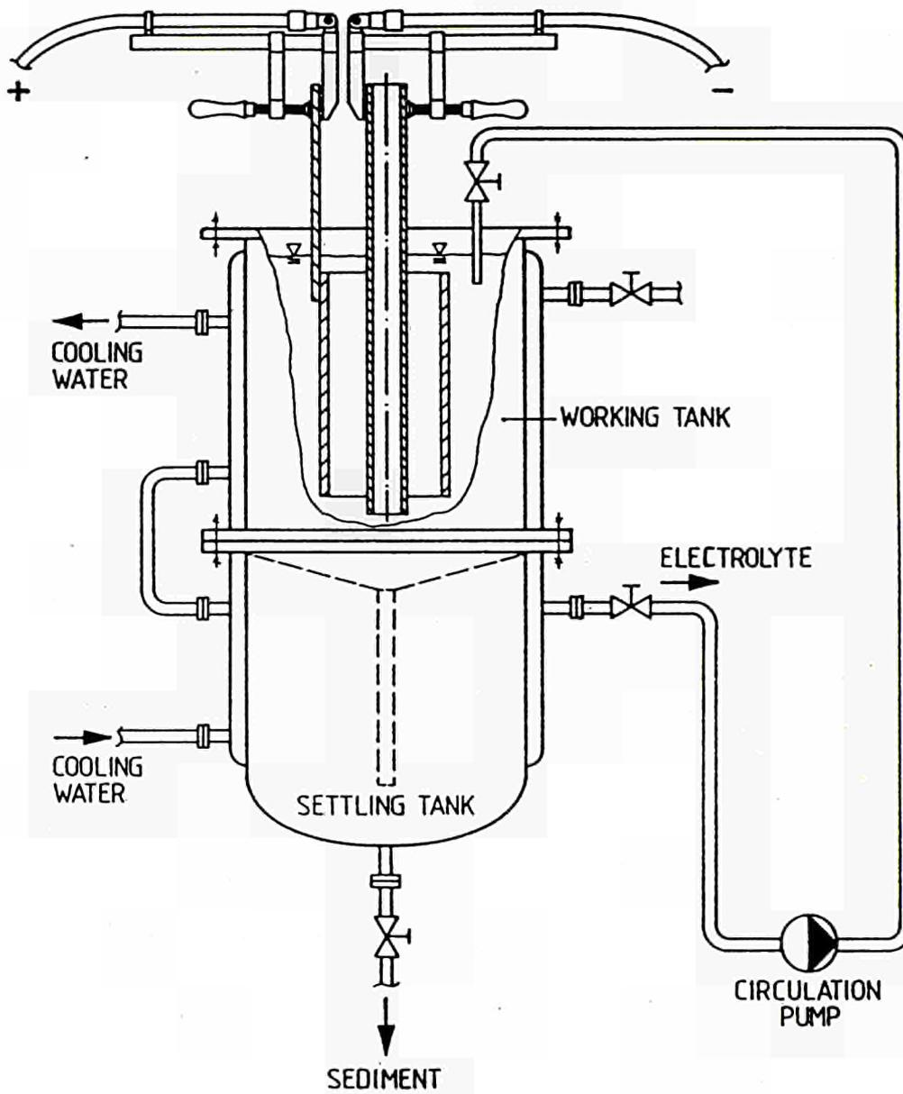
Figure 1: The electropolishing pilot plant 400 A
