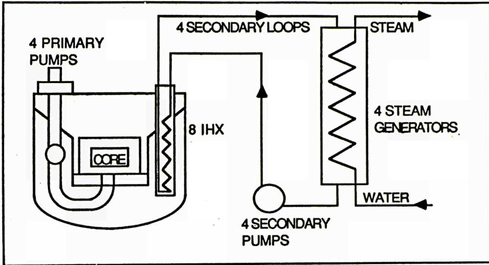
Figure 1: Pool type fast breeder reactor
