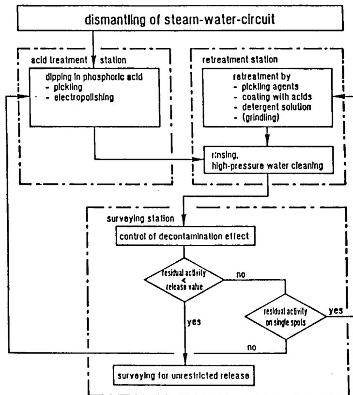
Fig. 1 Flow chart for decontamination of components of the steam-water-circuit
