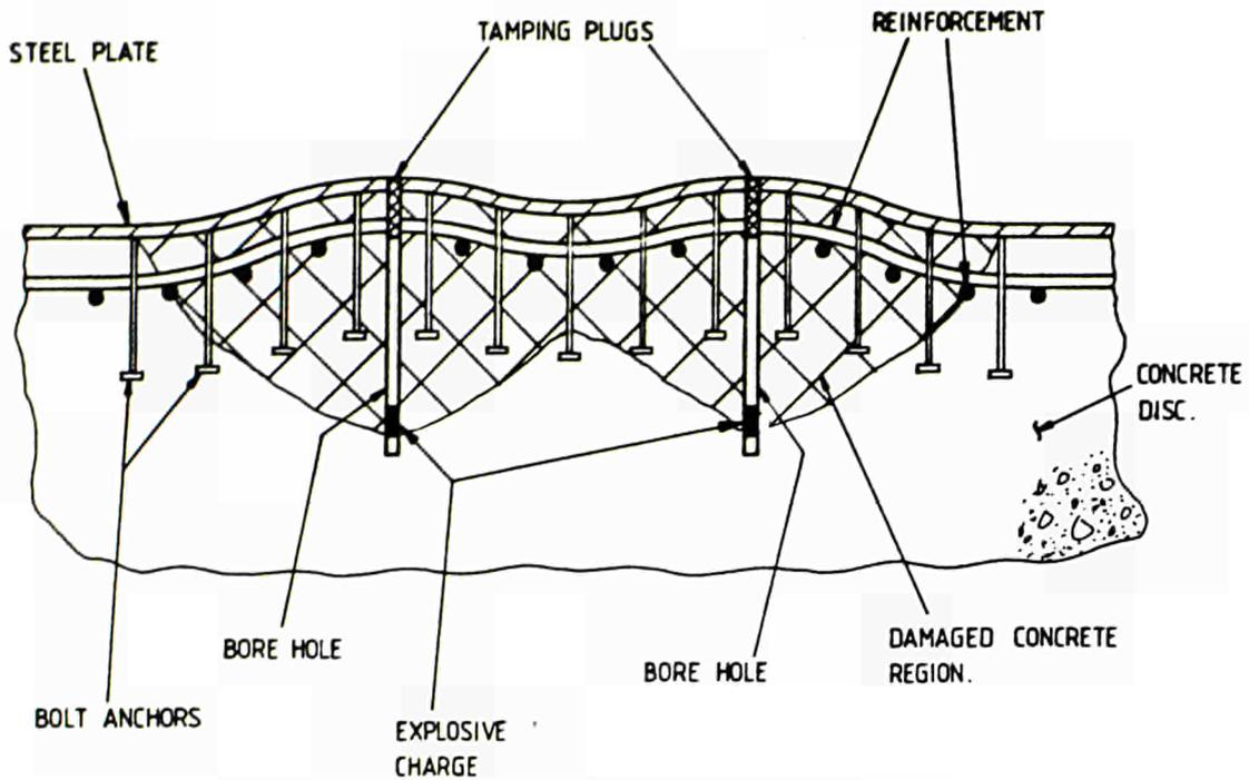
Fig. 1. Sketch of simulation of a steel lined concrete face after firing of multiple charges.
