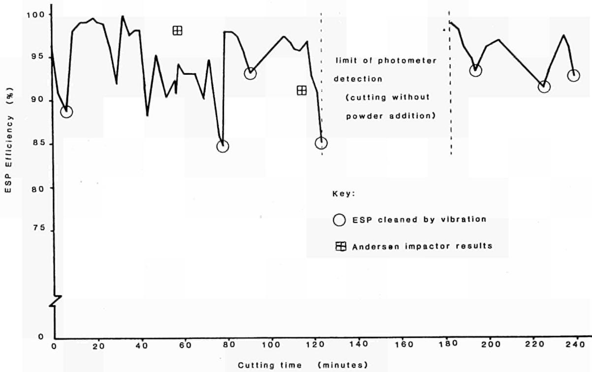
Figure 3. Efficiency of the electrostatic precipitator with time (photometer results)
