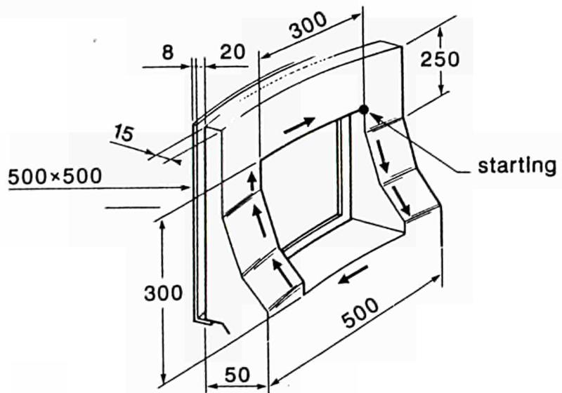
Figure 2 - VESSEL WALL WITH VARIABLE THICKNESS
