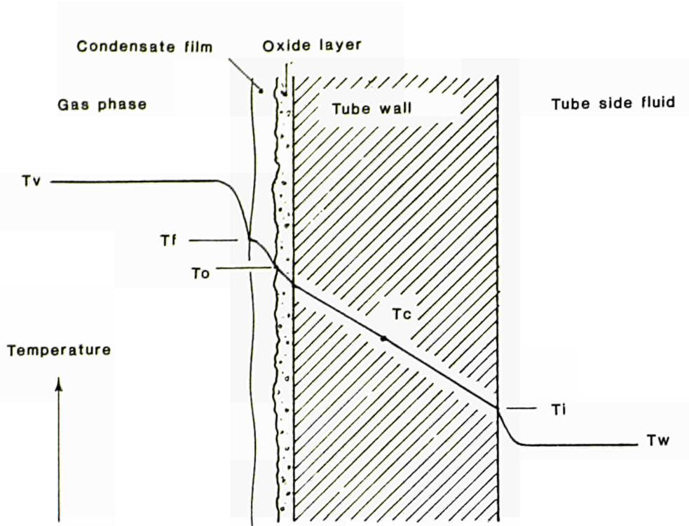
Figure 1. Temperature profile through the heat transfer regions
