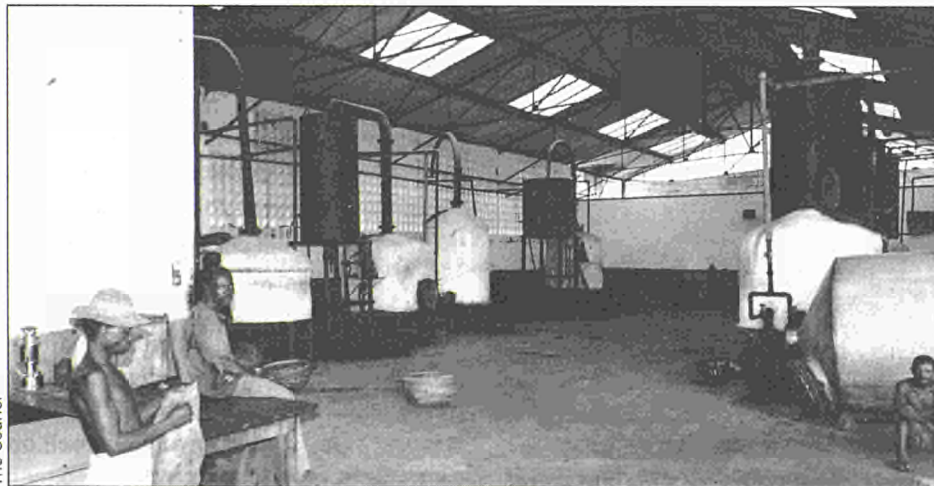
A factory for distillation of ylang-ylang. Most of the equipment is old and outdated
