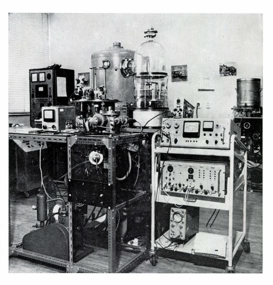
Some of the evaporation units used for the fabrication of nuclear targets and standards. The possibilities of heating the different metals and compounds to be evaporated *in vacuo* range from resistance heating to electron bombardment, r.f. heating and sputtering.
