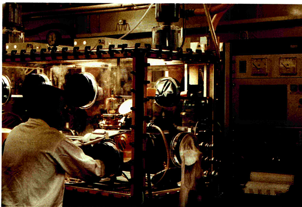
Fig. 2 Installation for welding of fuel pin end caps
