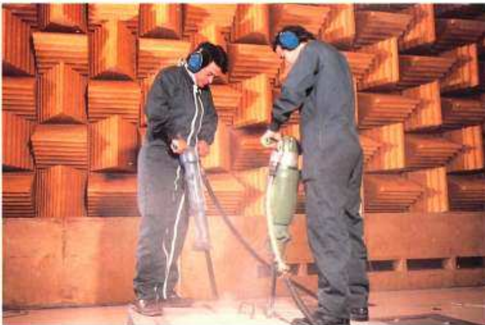
Testing pneumatic drills in an anechoic chamber; checking risks to hearing.
