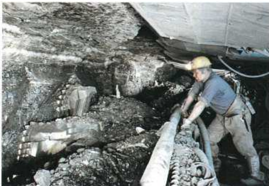
More powerful coal-cutting machinery generates more dust. Photo: RAG-Foto
