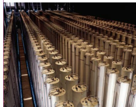
*Cascade hall in a gas centrifuge enrichment plant.*
