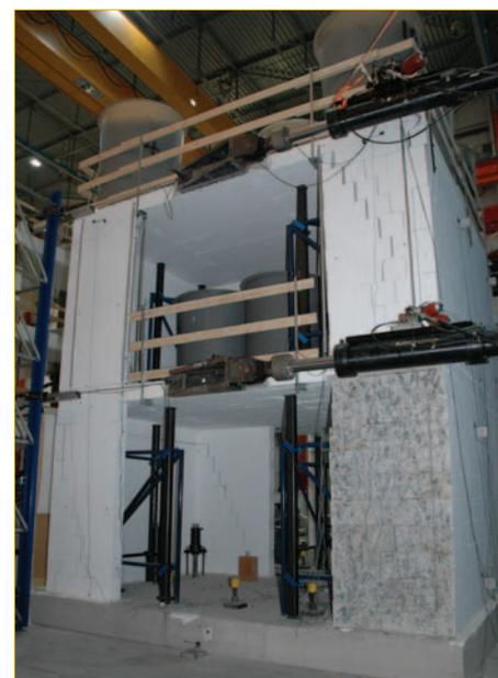
Figure 1: Masonry house specimen tested at the ELSA laboratory in the framework of the competitive project ESECMaSE: a series of pseudo-dynamic tests representing earthquakes of increasing intensity has been carried out up to the onset of collapse characterised by large stepwise cracks and/or joint slidings in most walls.
