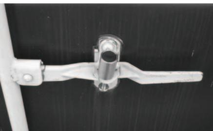
*Passive electronic seal with three transponders on a container.*
