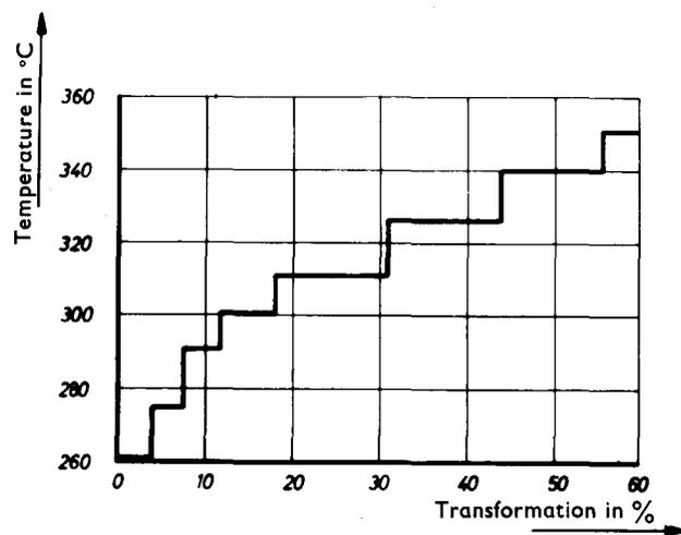
Fig. 4 — Transformation of  $\text{Ca}(\text{OH})_2$  into  $\text{CaCO}_3$  as a function of the temperature.
