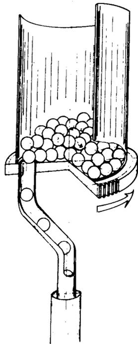
Fig. 2 — Schematic representation of the Singulizer.
