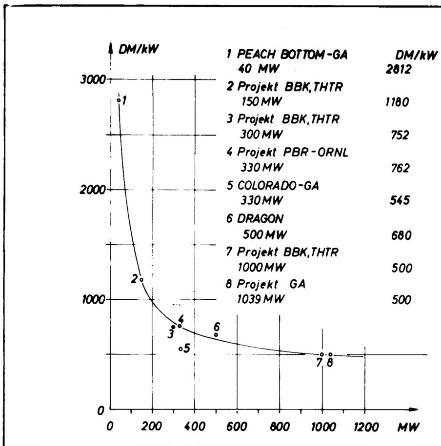
Fig. 4 — Specific capital costs of high temperature reactor stations as a function of the reactor power.
