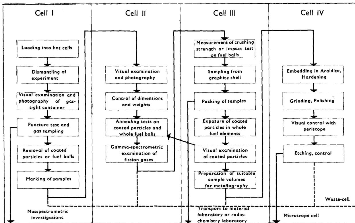
Fig. 7 — Operations in THTR cells.
