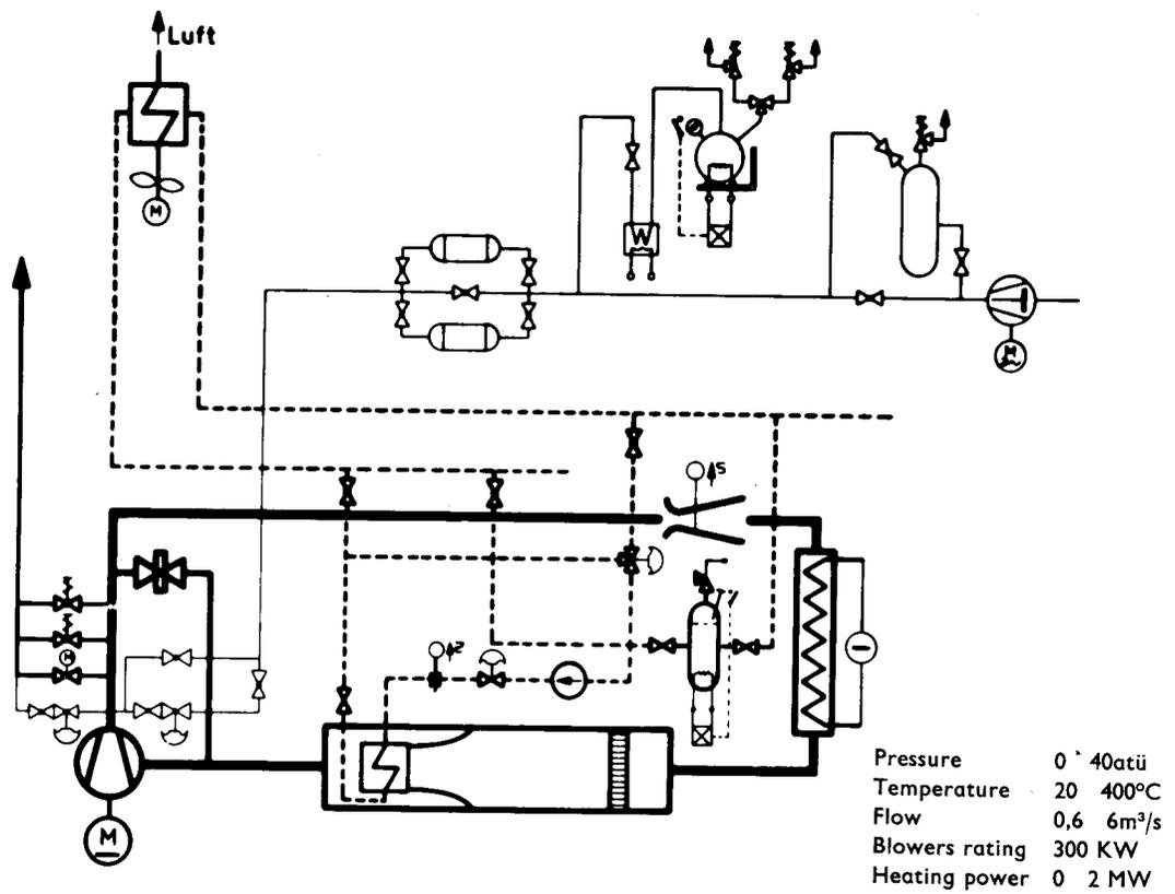
Fig. 2 — Sketch of the High Pressure Gas Channel.
