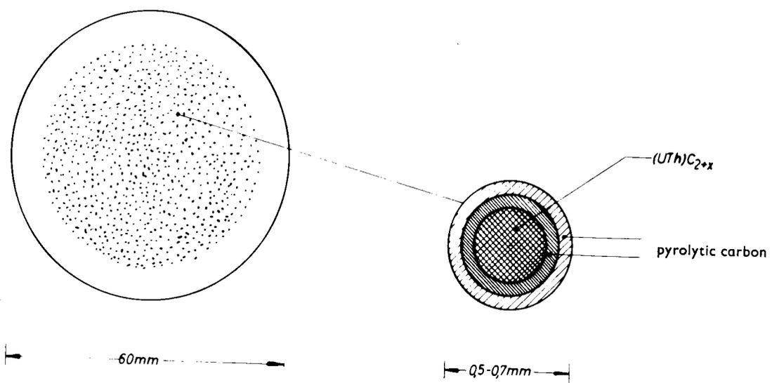
Fig. 1 — Fuel element with coated particles.
