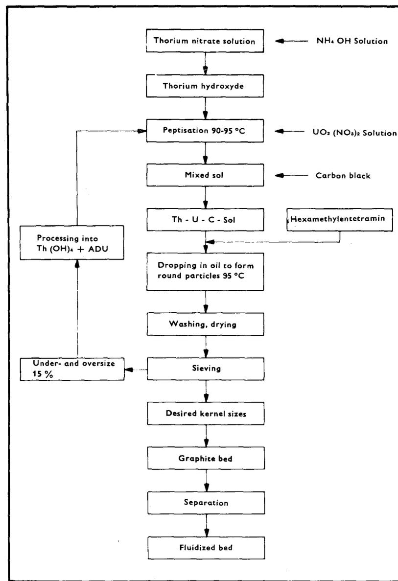
Fig. 3 — Preparation of particles Sol. gel method.
