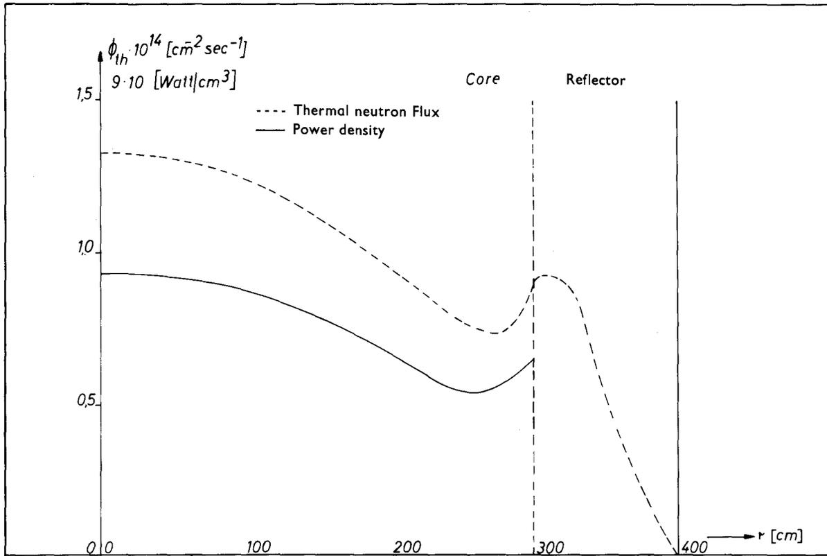
Fig. 4 — Thermal neutron flux and power density in the radial direction (core middle).
