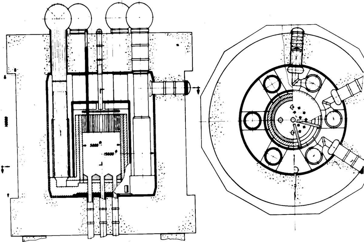
Fig. 1 — Sectional view of the 300 MWe THTR prototype.
