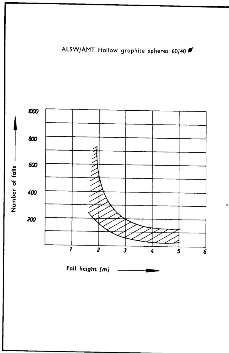
Fig. 7 — Fall tests on a bed of balls.
