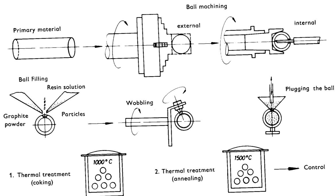
Fig. 6 — Preparation of hollow sphere fuel elements.
