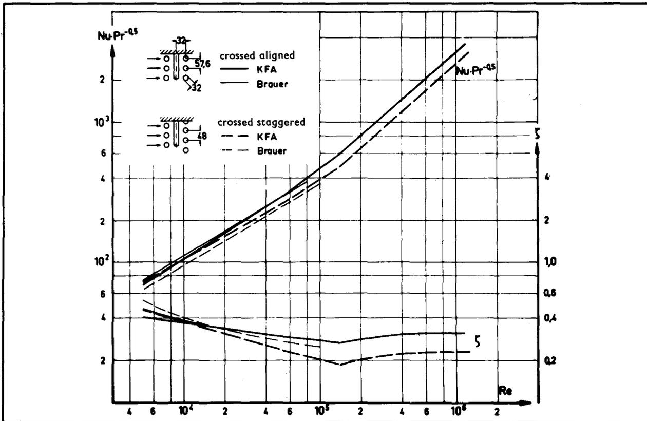
Fig. 6 — Heat transfer and pressure drop for two crossed tubes arrangement.
