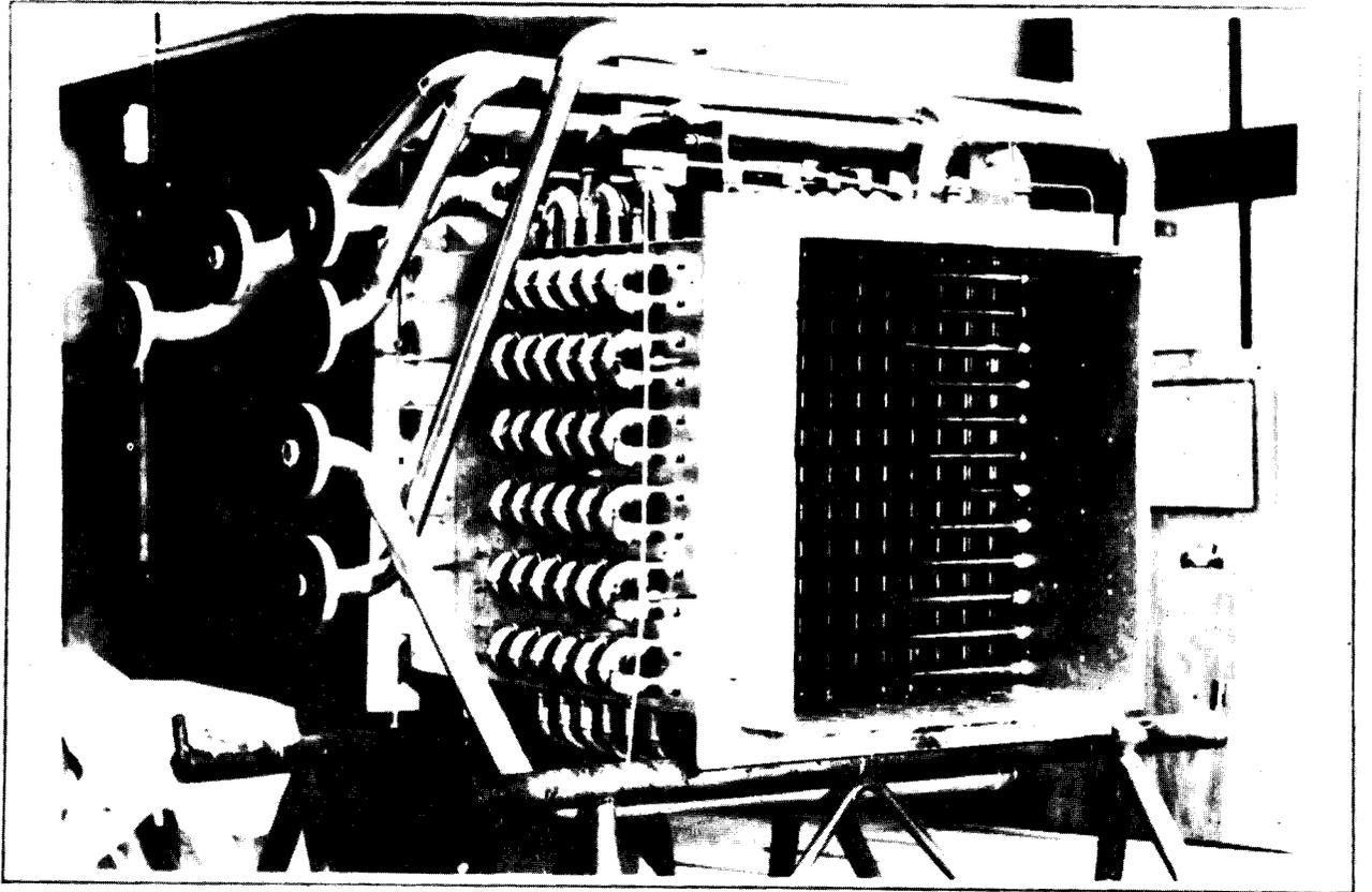
Fig. 1 — Crossed aligned tubes bundle.
