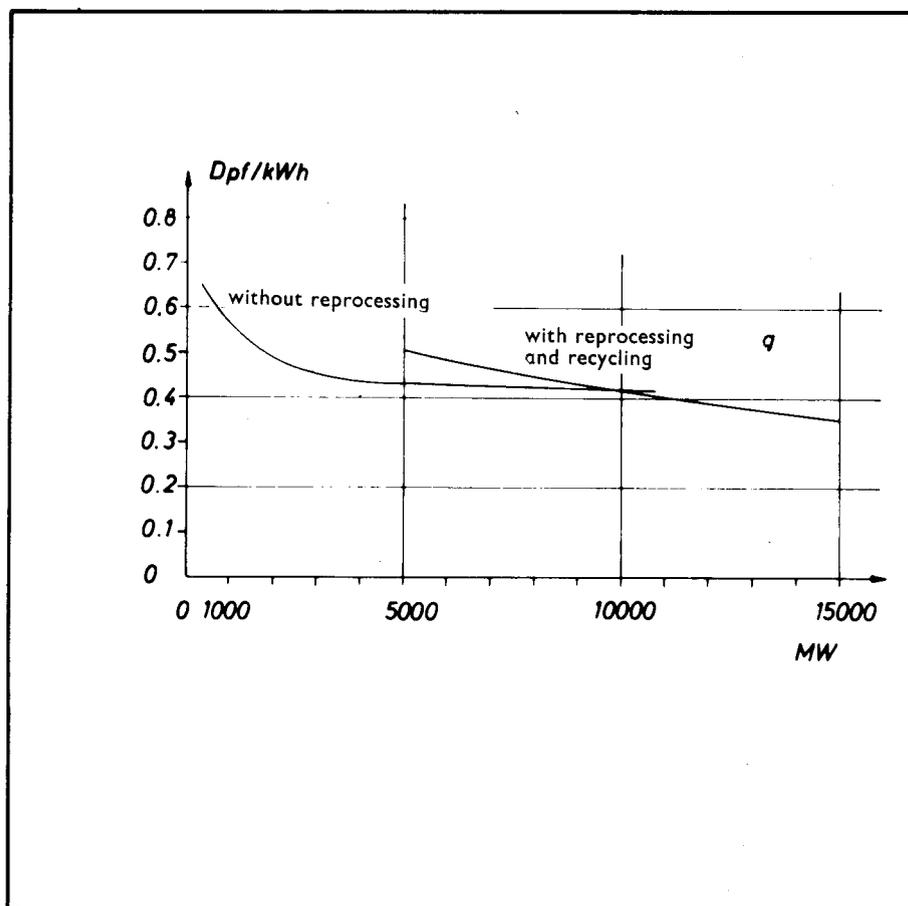
Fig. 5 — Fuel cycle costs as a function of the reactor power.
