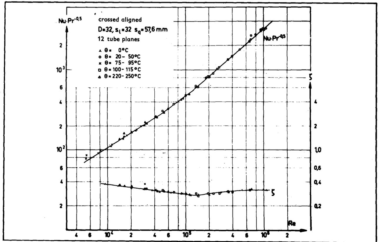
Fig. 5 — Heat transfer and pressure drop for the crossed aligned tubes arrangement.
