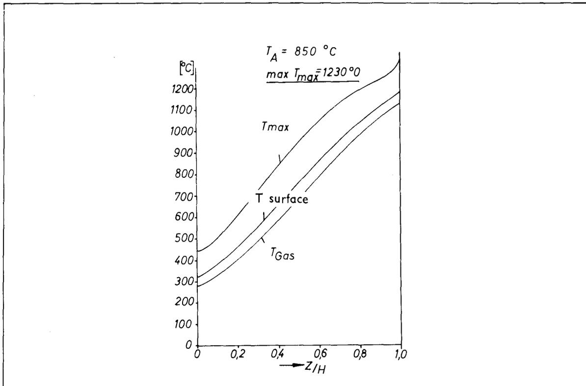
Fig. 5 — Axial temperature distribution.
