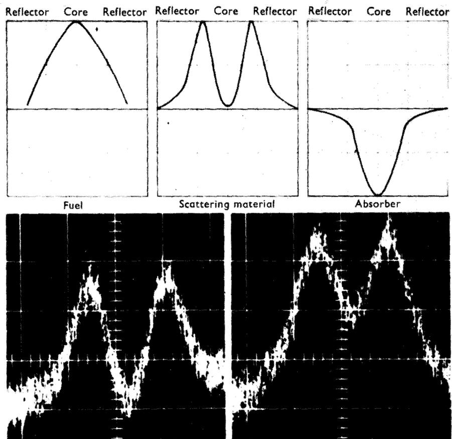
Fig. 4 — Influence function and measured signal of a critical assembly.
