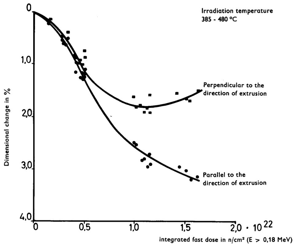
Fig. 1 — Dimensional changes of isotropic graphite.
