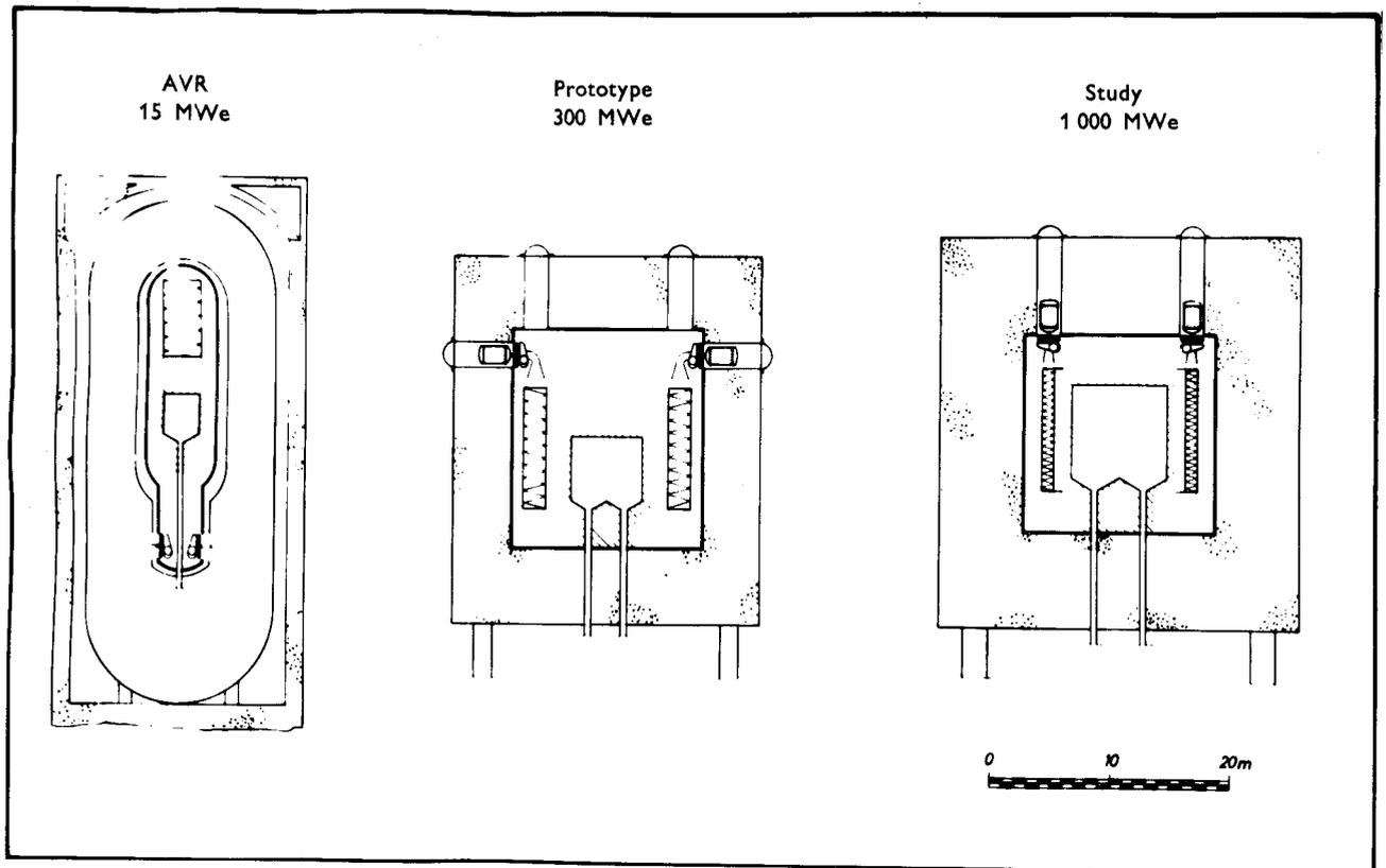
Fig. 3 — Size comparison between the AVR, a 300 MWe and a 1 000 MWe prototypes.
