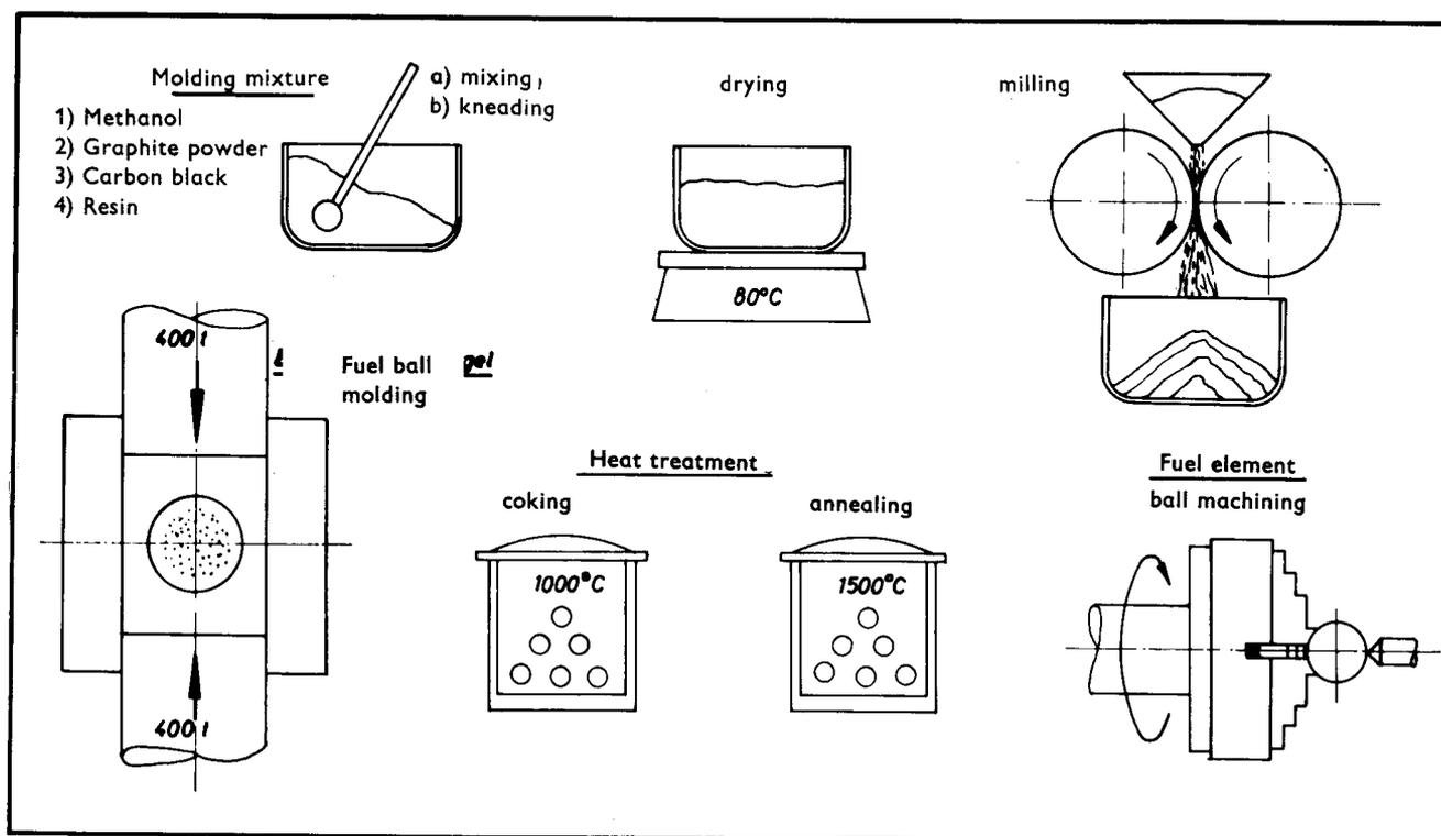
Fig. 8 — Preparation of molded fuel elements.
