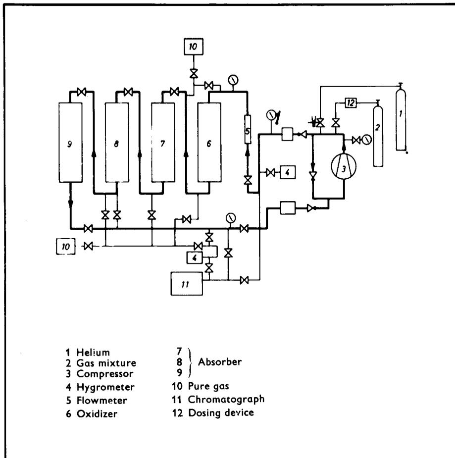
Fig. 5 — Schematic representation of the rig used for the laboratory tests.
