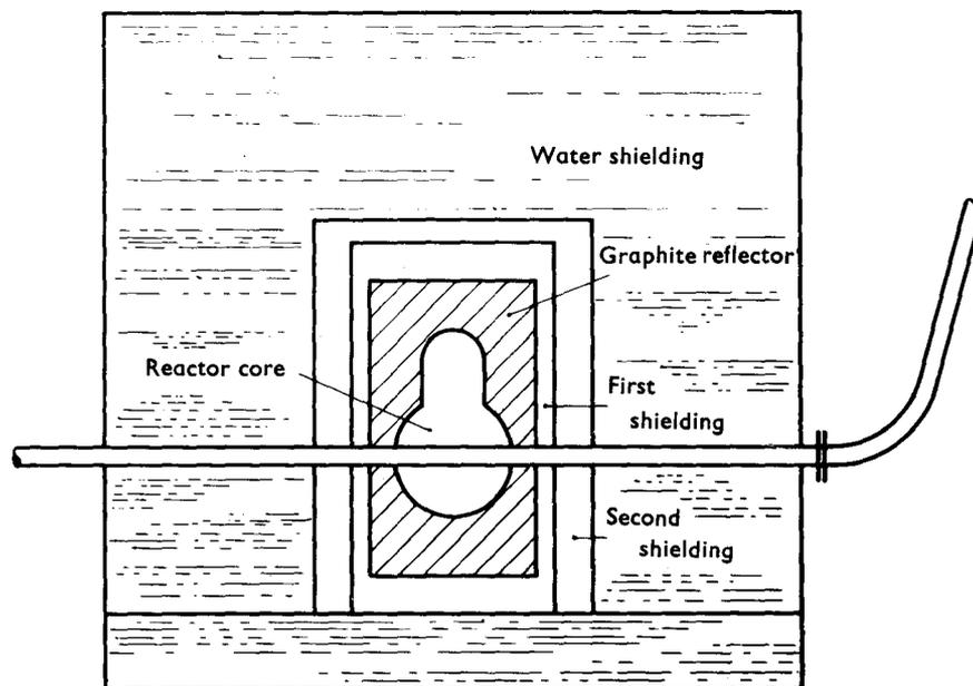
Fig. 5 — Sketch of a homogeneous liquid reactor used for the development of a burn-up measurement.
