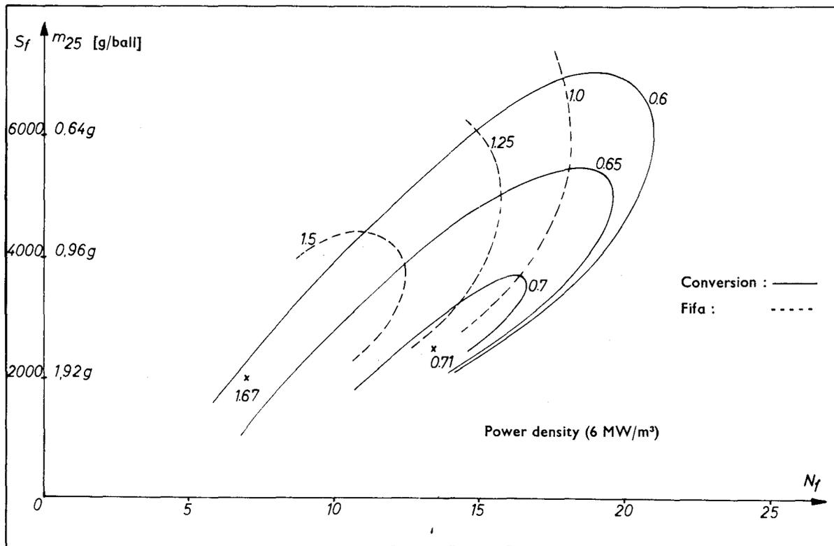
Fig. 1 — Conversion factor and fifa "without reprocessing".
