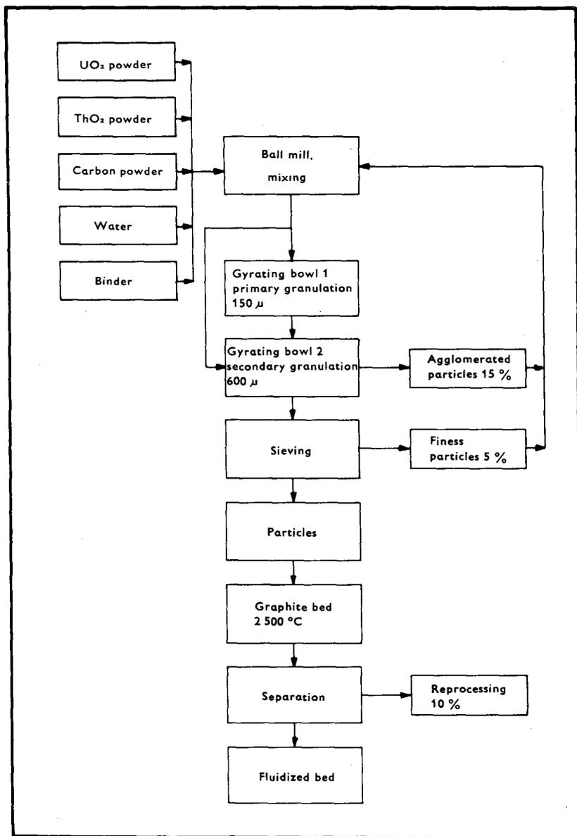
Fig. 2 — Preparation of particles gyration bowl method.
