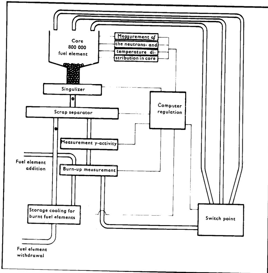
Fig. 1 — Schema of the loading-unloading circuit.
