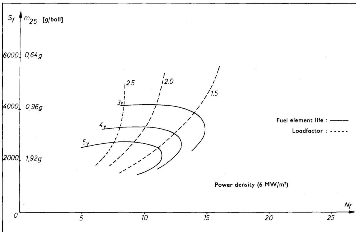
Fig. 2 — Load factor and fuel element lifetime "without reprocessing".
