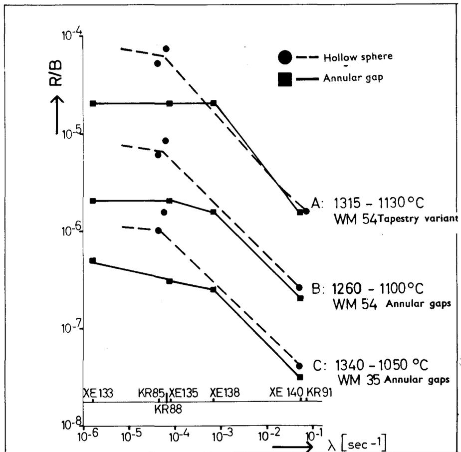
Fig. 4 — Fission gas release of coated particles under irradiation.
