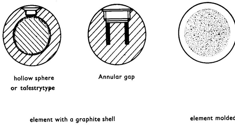
Fig. 1 — Fuel element types for high temperature gas cooled reactor.
