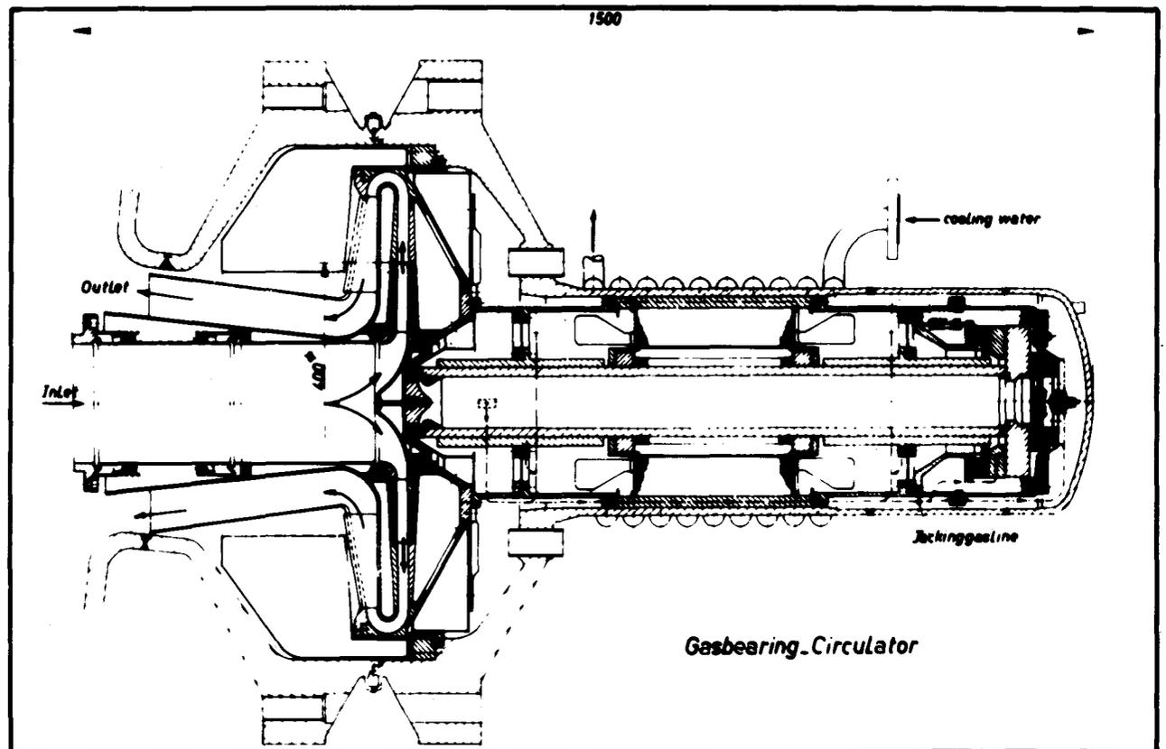
Fig. 4 — Section through the Dragon blower.
