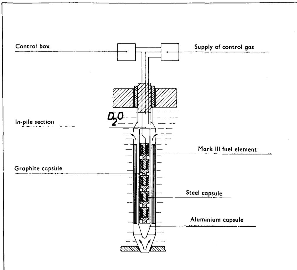
Fig. 3 — Irradiation capsule for coated particles.
