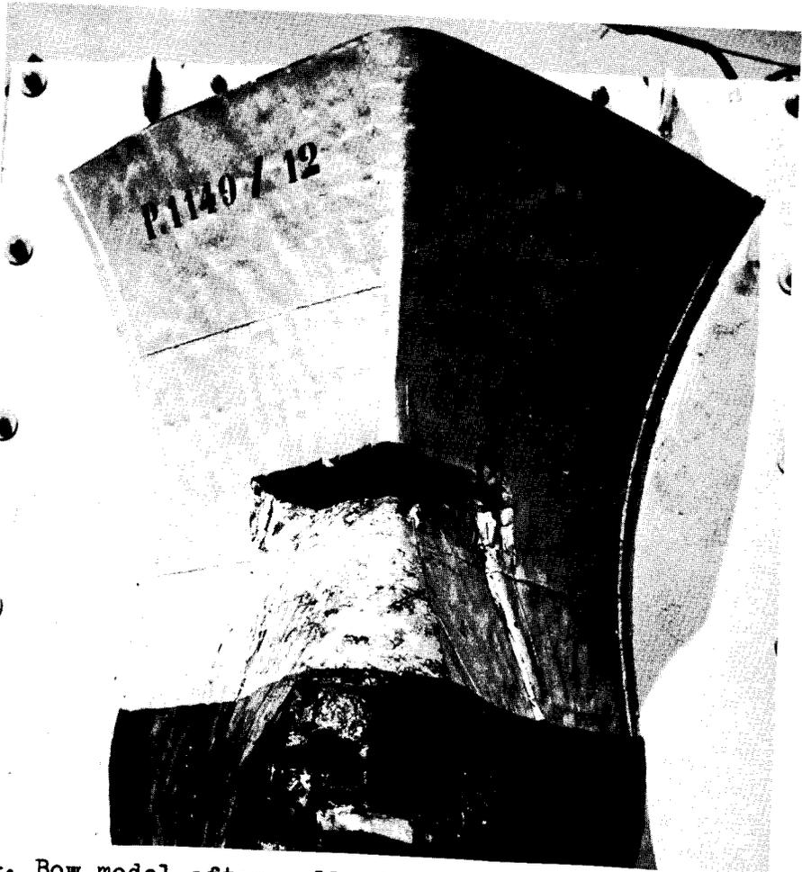
34. Bow model after collision test No. 12
