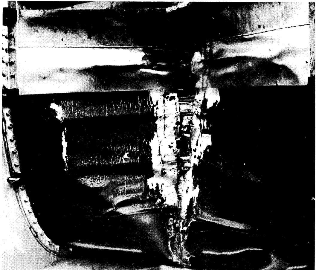
29. Ship side model after collision test No. 9
