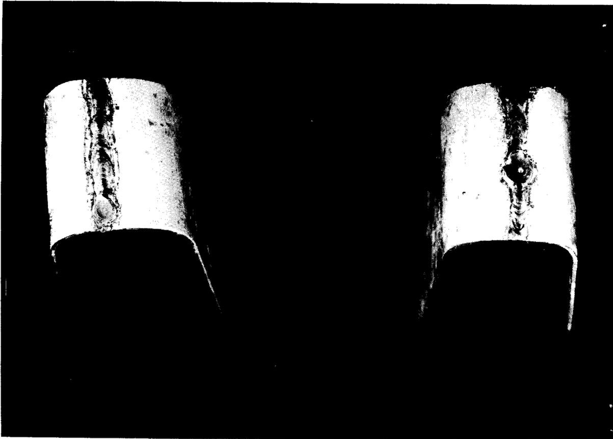
1. 180° bending test of an electrically welded specimen
