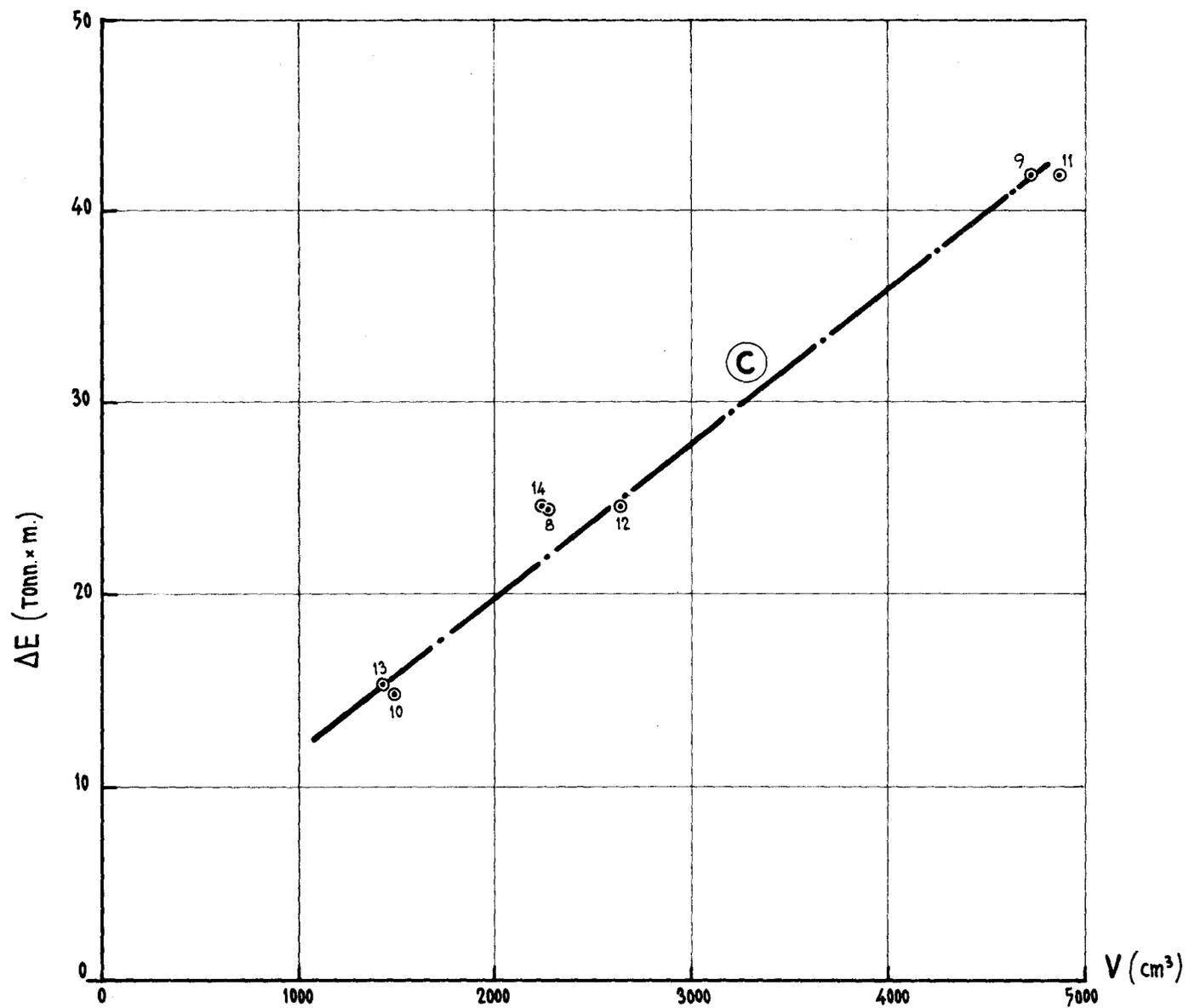
Fig. 42 RELATION BETWEEN VOLUMES OF MATERIAL AFFECTED BY THE COLLISION AND DISSIPATED ENERGY
