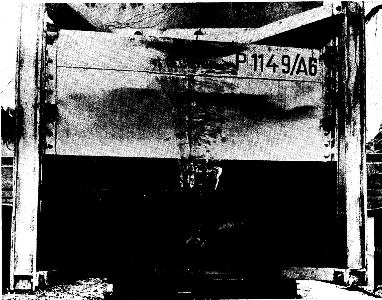
22. Ship side model after collision test No. 6
