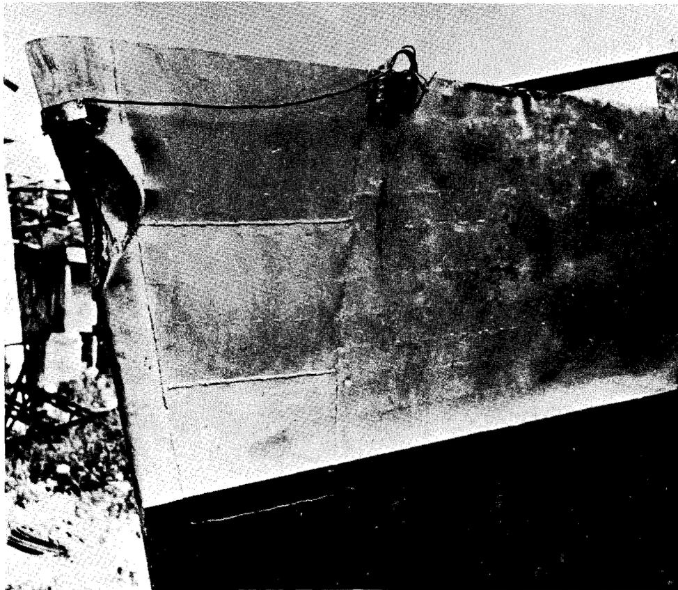
24. Bow model after collision test No. 7
