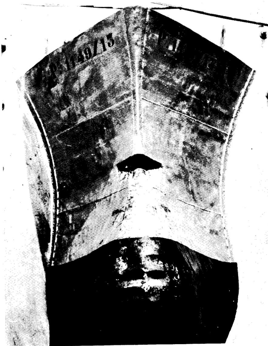
36. Bow model after collision test No. 13
