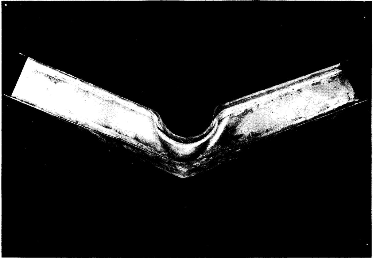
3. Bending test of a tin soldered H specimen
