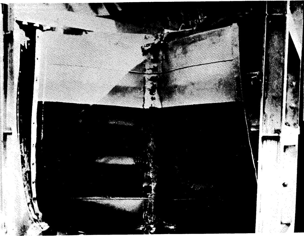
14. Ship side model after collision test No. 2
