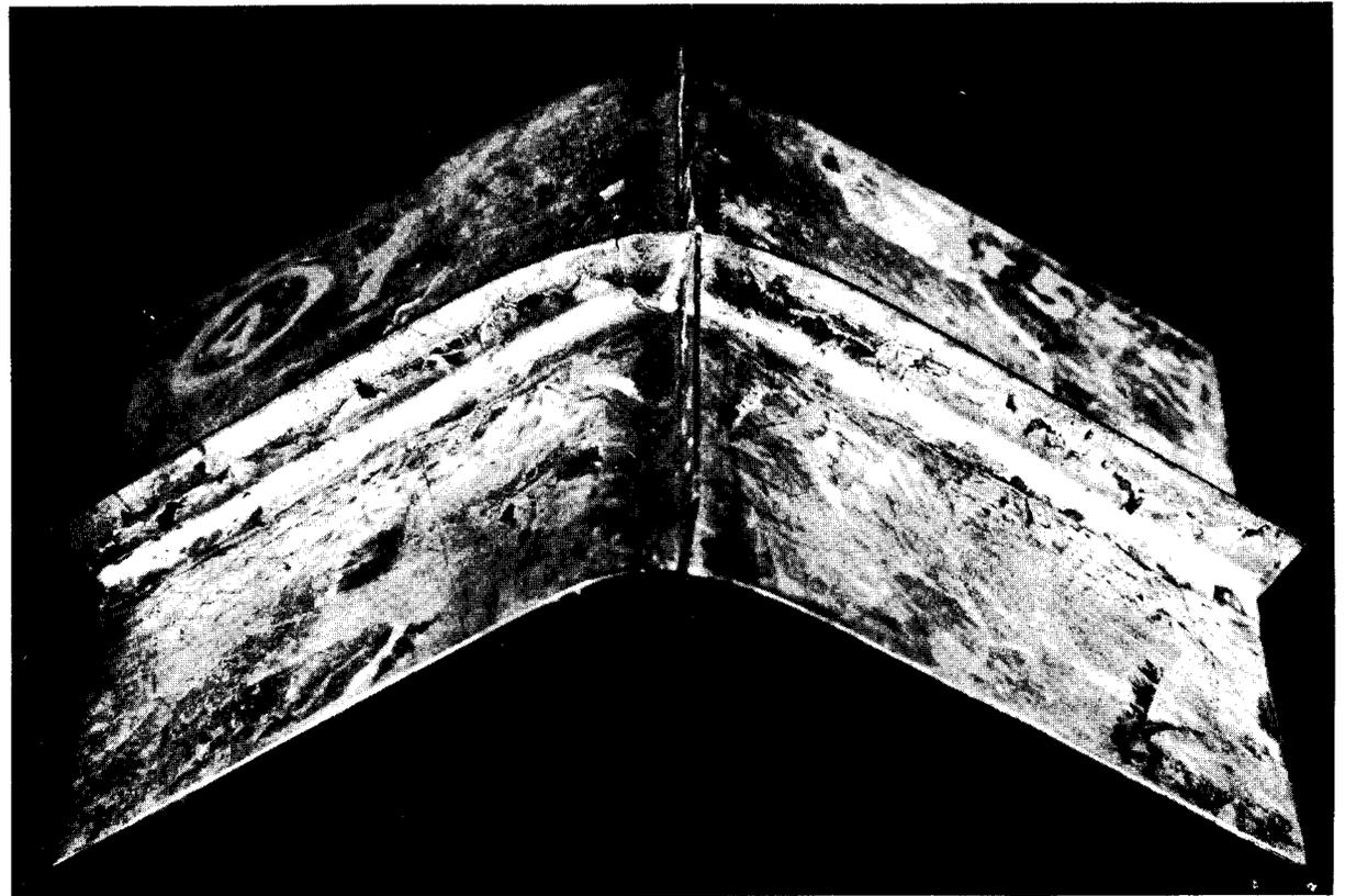
4. Bending test of a tin soldered cross shaped specimen
