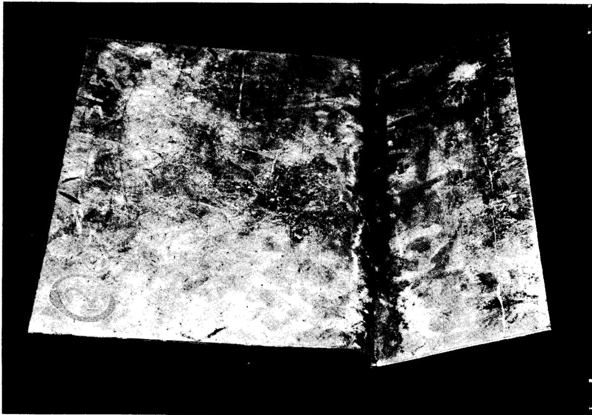
2. 180° bending test of a tin soldered T specimen
