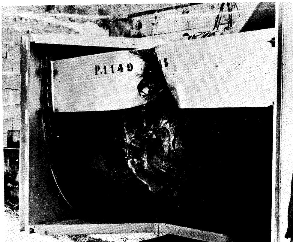
37. Ship side model after collision test No. 13
