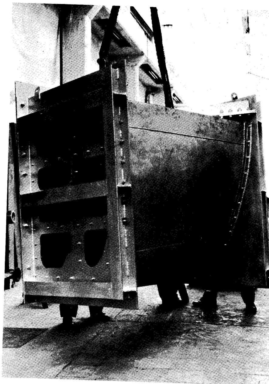
10. Ship side model for collision test No. 1
