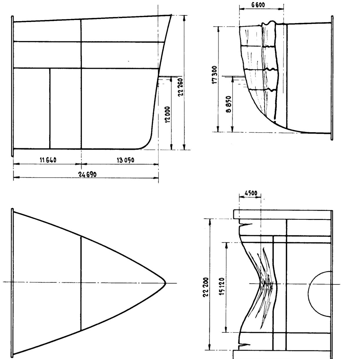
BOW AND SHIPSIDE MODELS BEFORE 6<sup>TH</sup> COLLISION TEST
