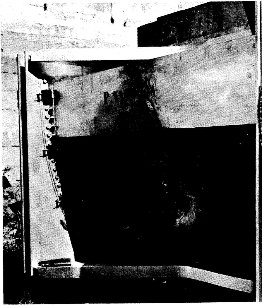
39. Ship side model after collision test No. 14
