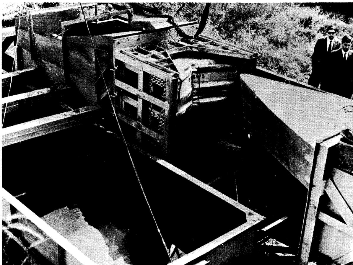
19. Bow and ship side models after collision test No. 5
