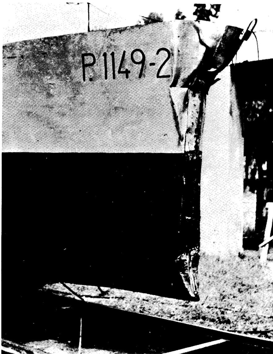
17. Bow model after collision test No. 4
