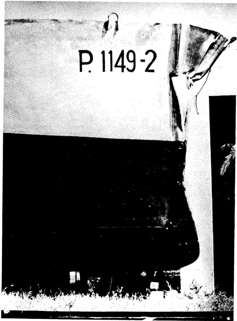
15. Bow model after collision test No. 3
