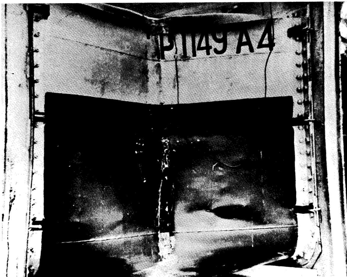
16. Ship side model after collision test No. 3
