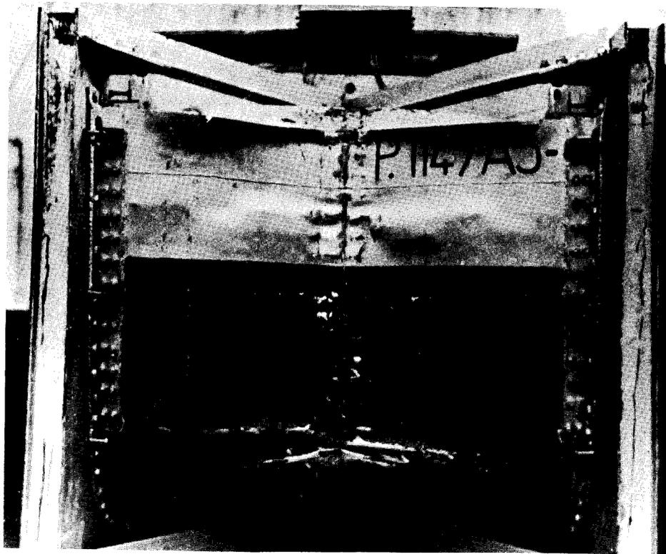
18. Ship side model after collision test No. 4
