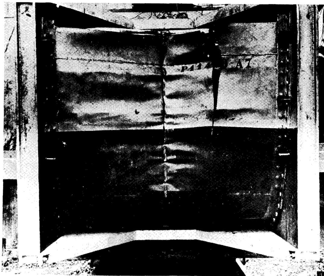
25. Ship side model after collision test No. 7
