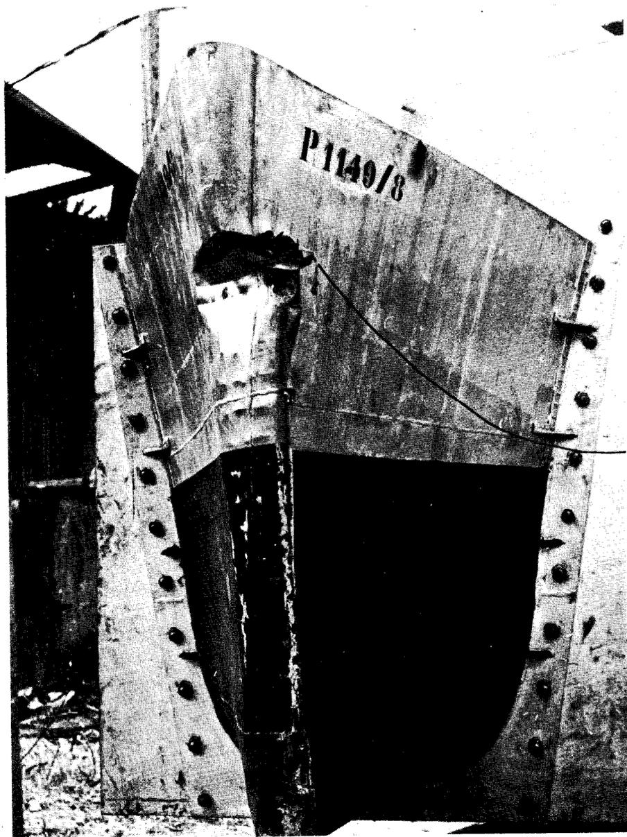
26. Bow model after collision test No. 8
