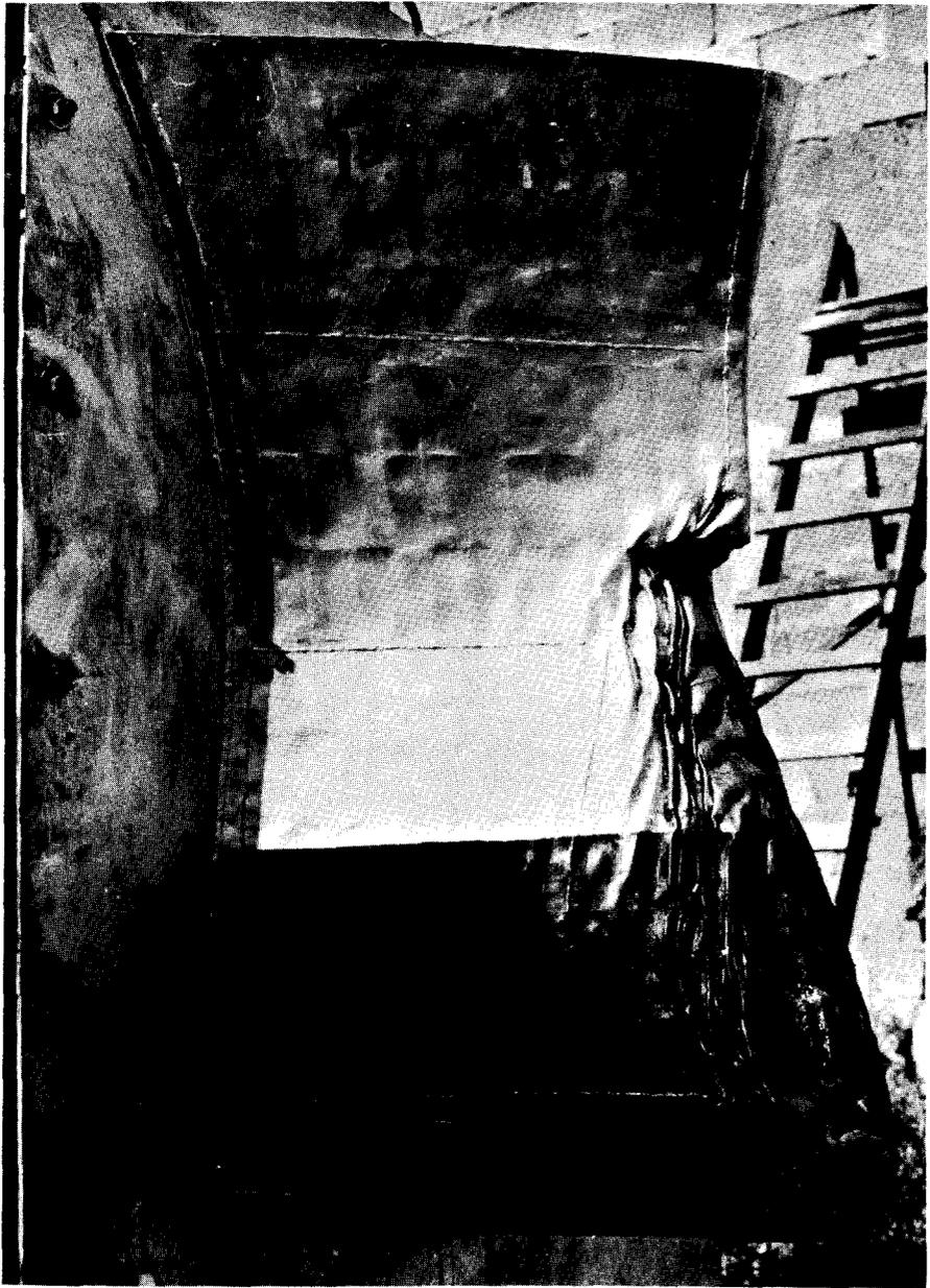
38. Bow model after collision test No. 14
