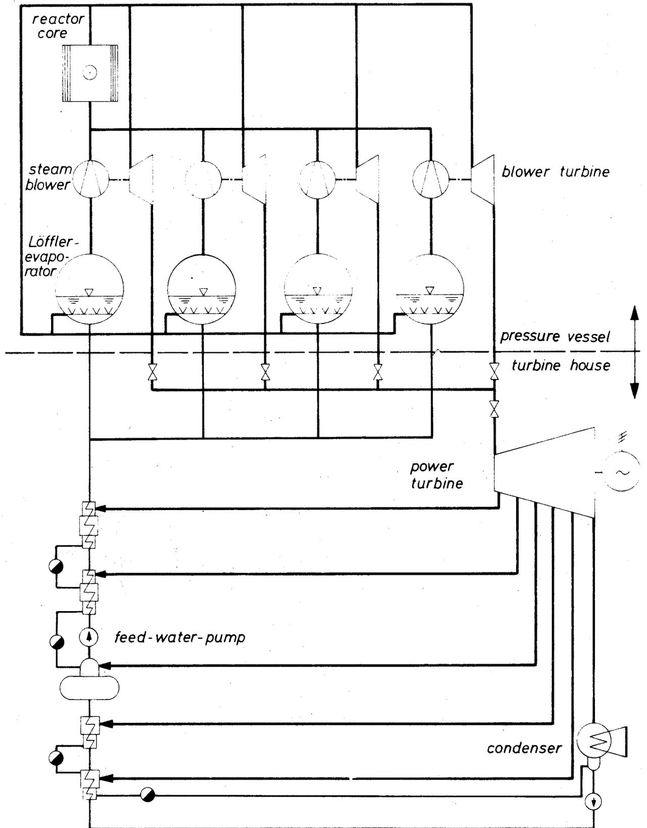
Fig.10 Heat flow diagram of a steam cooled fast reactor
