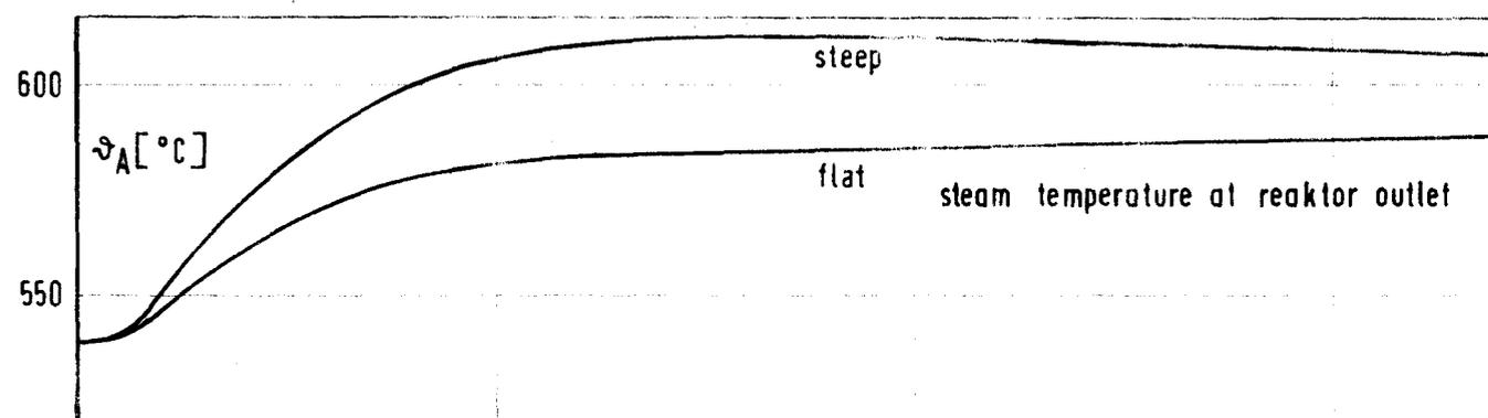
Fig. 6 Steam mass flow and exit temperature transients following the failure of 1 out of 6 blowers
