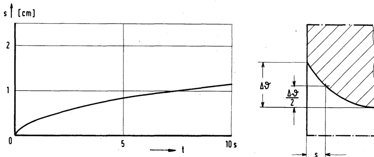
Fig. 3 Penetration depth of a temperature disturbance in steel
