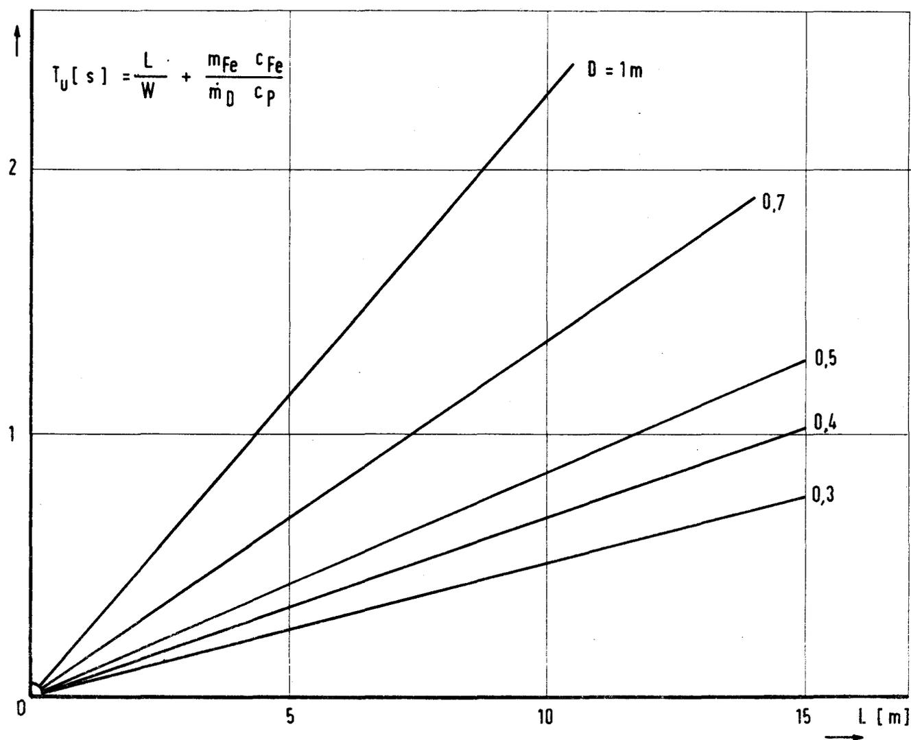
Fig. 4 Delay time in steam pipes
