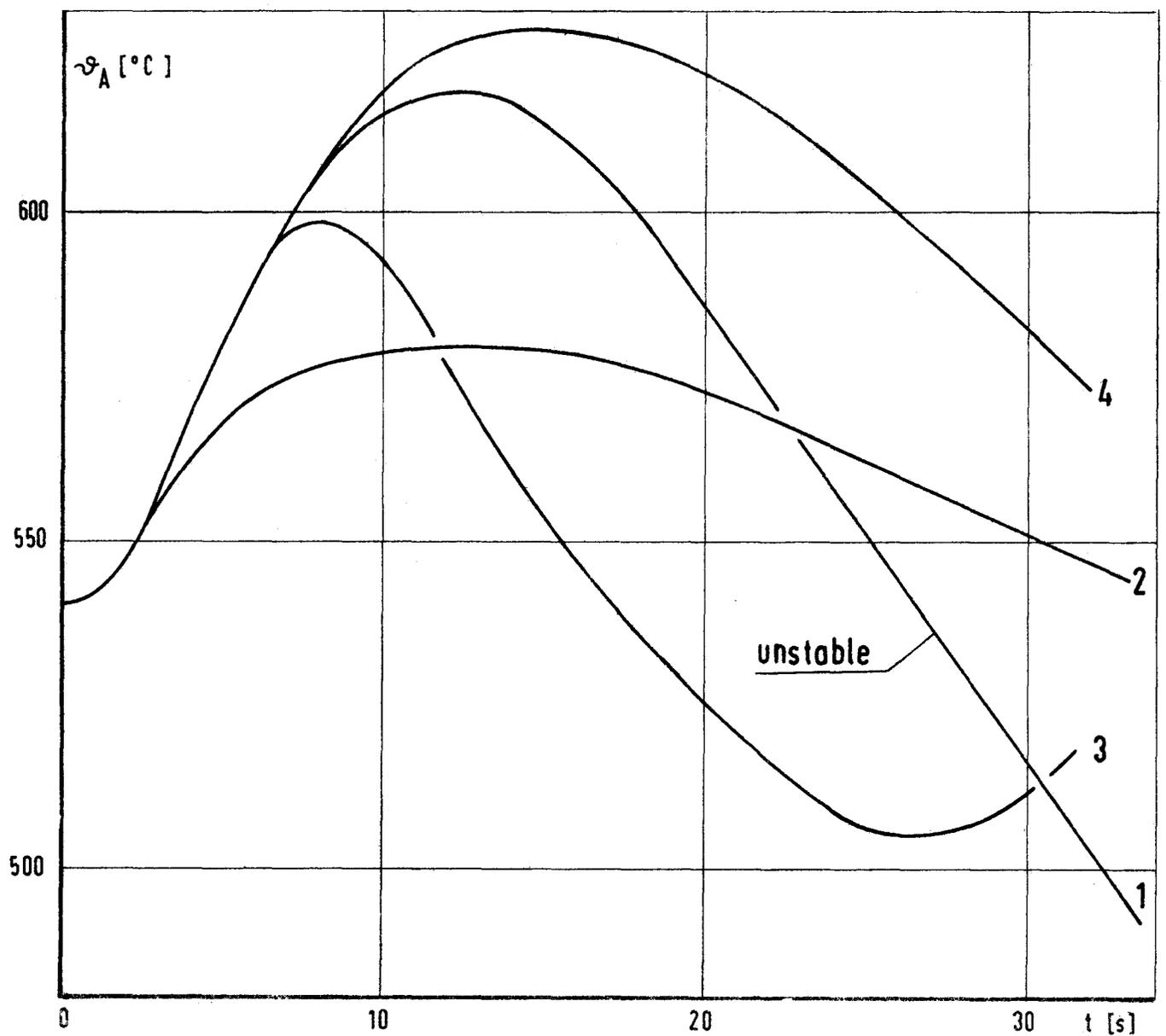
Fig. 5 Exit steam temperature transient following a 0.2\$ reactivity step
