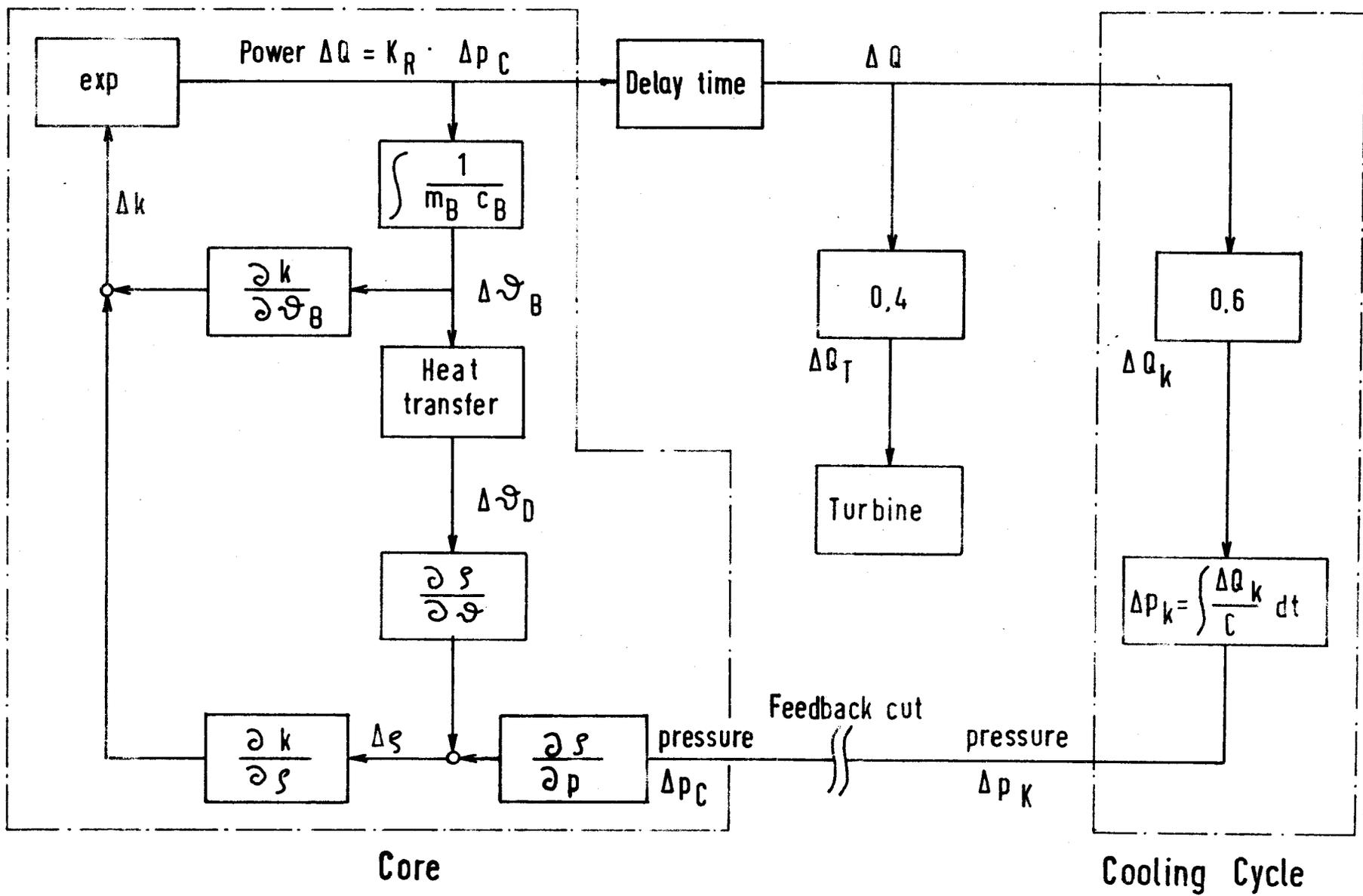
Fig. 1 Feedback of core and cooling cycle
