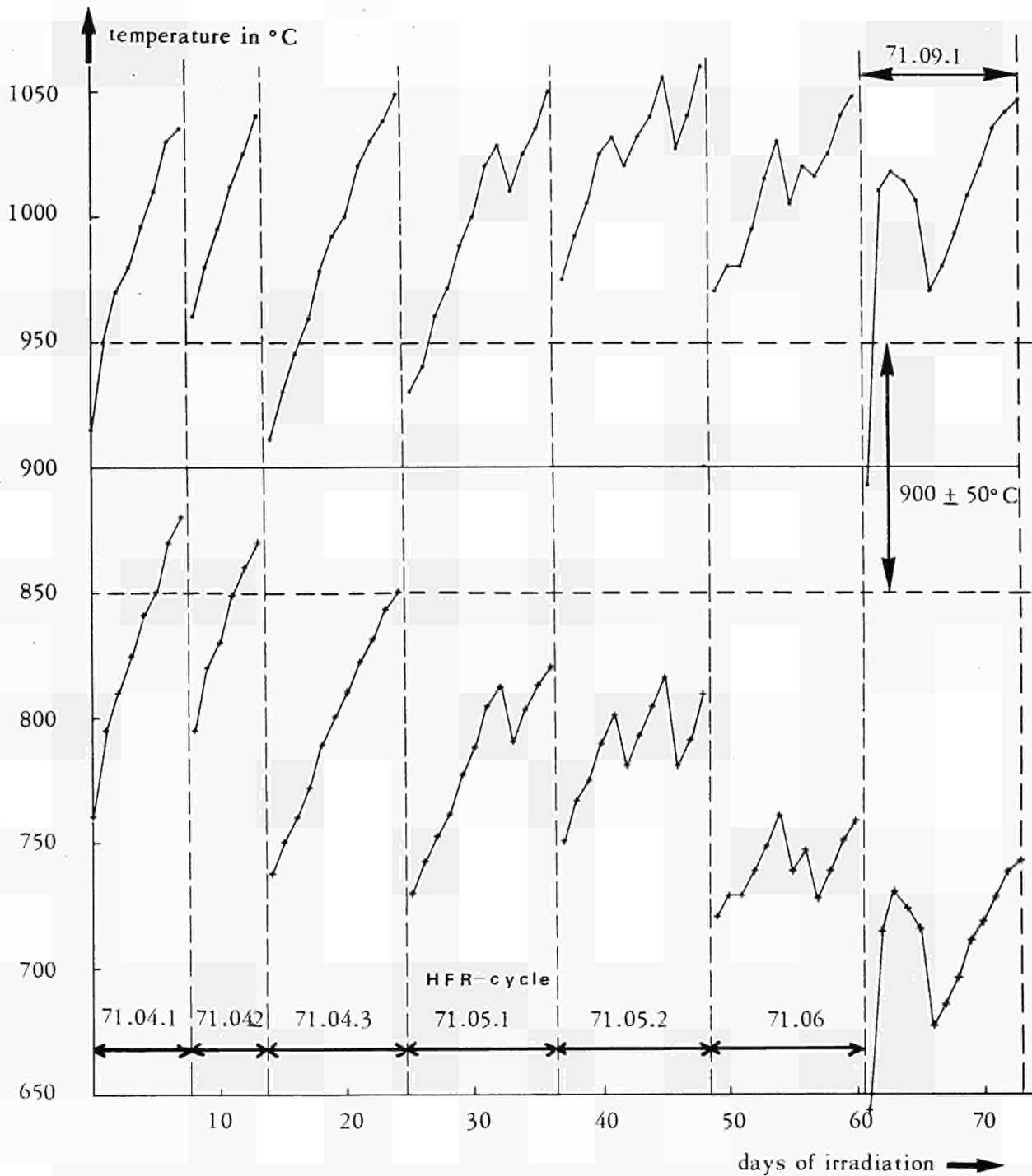
Fig. 15 Graphite-box-nr. 1: Temperatures measured with the thermocouples nr. 14 and 16 (see Fig. 9) as a function of the irradiation days
