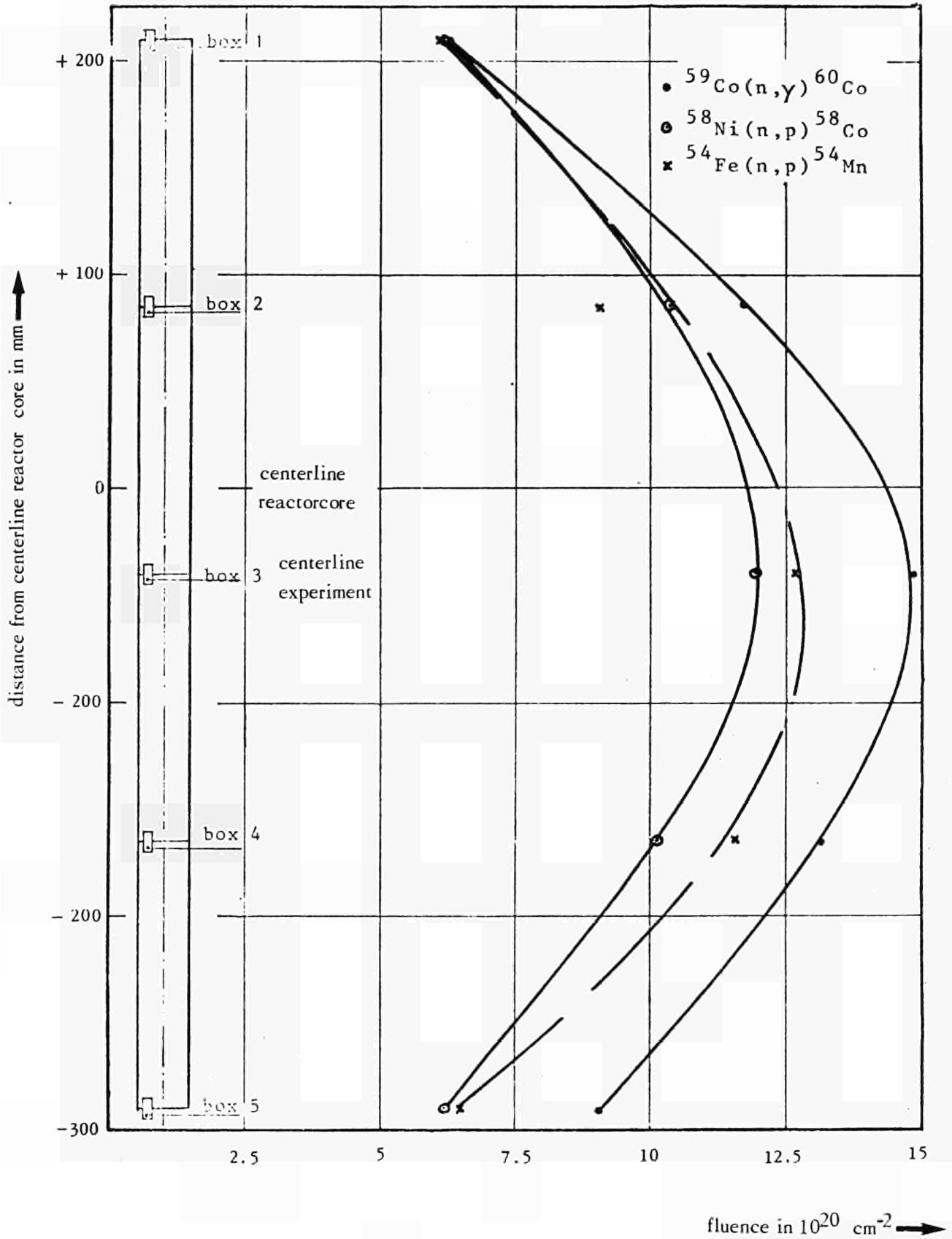
Fig. 24b Vertical thermal and fast fluence distributions measured in experiment E96-1, HFR-position E3, [ Ref. 6 ]
