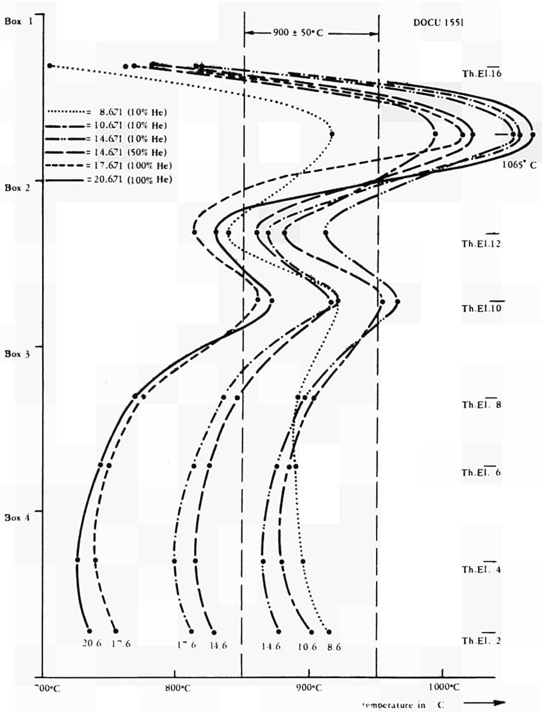
Fig. 11 Vertical temperature distribution measured with the inner thermocouples during the HFR-cycle 71.05.2. Gas mixture in outer capsule in parentheses
