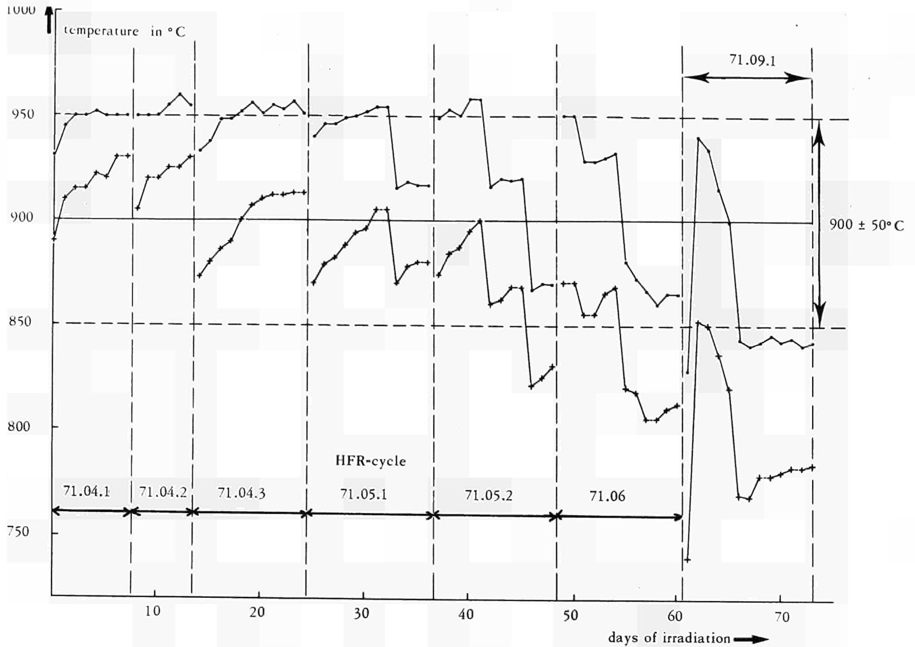
Fig. 16 Graphite-box-nr. 2: Temperatures measured with the thermocouples nr. 10 and 12 (see Fig. 9) as a function of the irradiation days
