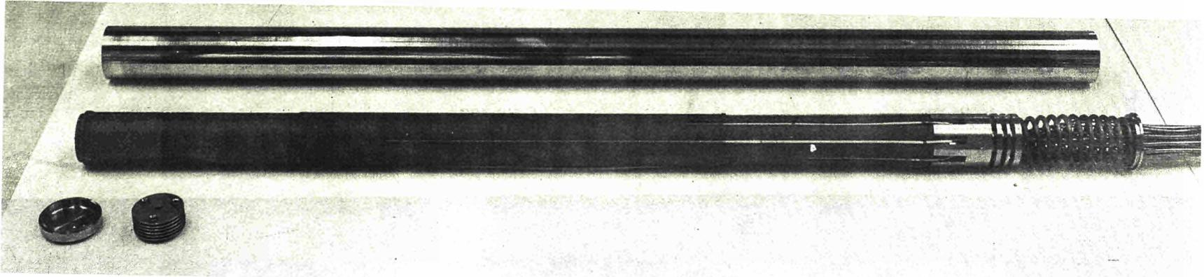
Fig. 6 Sample carrier. Graphite-boxes assembled with st.stl. tube, end caps and heat shield not yet assembled
