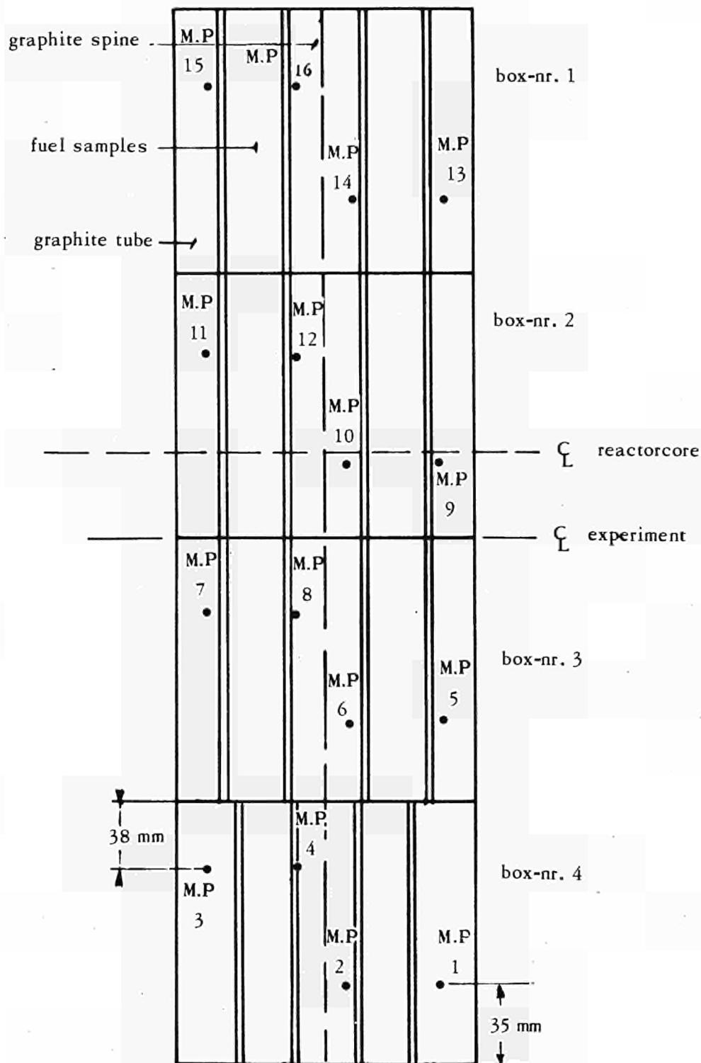
Fig. 9 Positions of the thermocouples nr. 1-16 in the graphite boxes (M.P. = measuring point)
