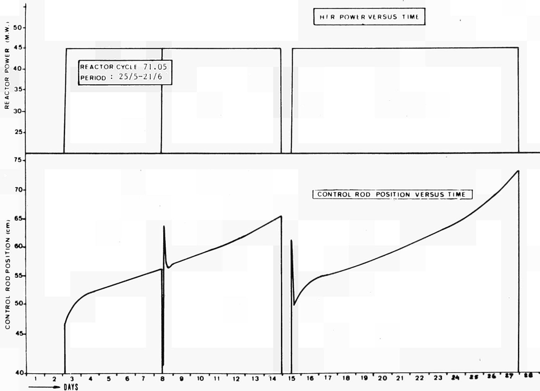
Fig. 21 HFR power and control rod position vs. time. HFR-cycle 71.05
