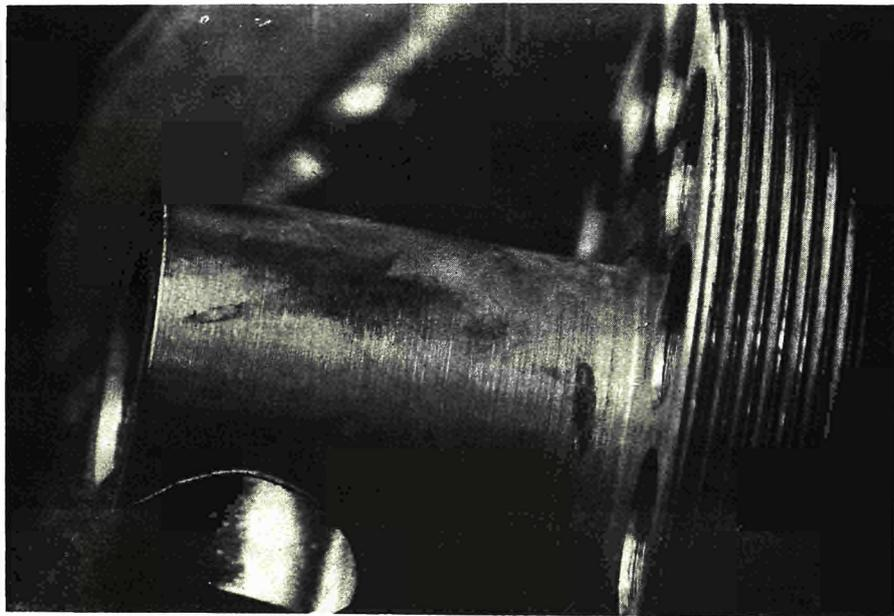
Fig. 26 Fretting on the outer endplug caused by the bent part of a minitube and by vibration.
