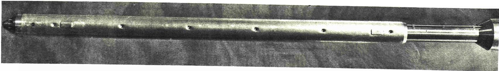
Fig. 7 Irradiation-rig. In-pile section assembled with Al-thimble
