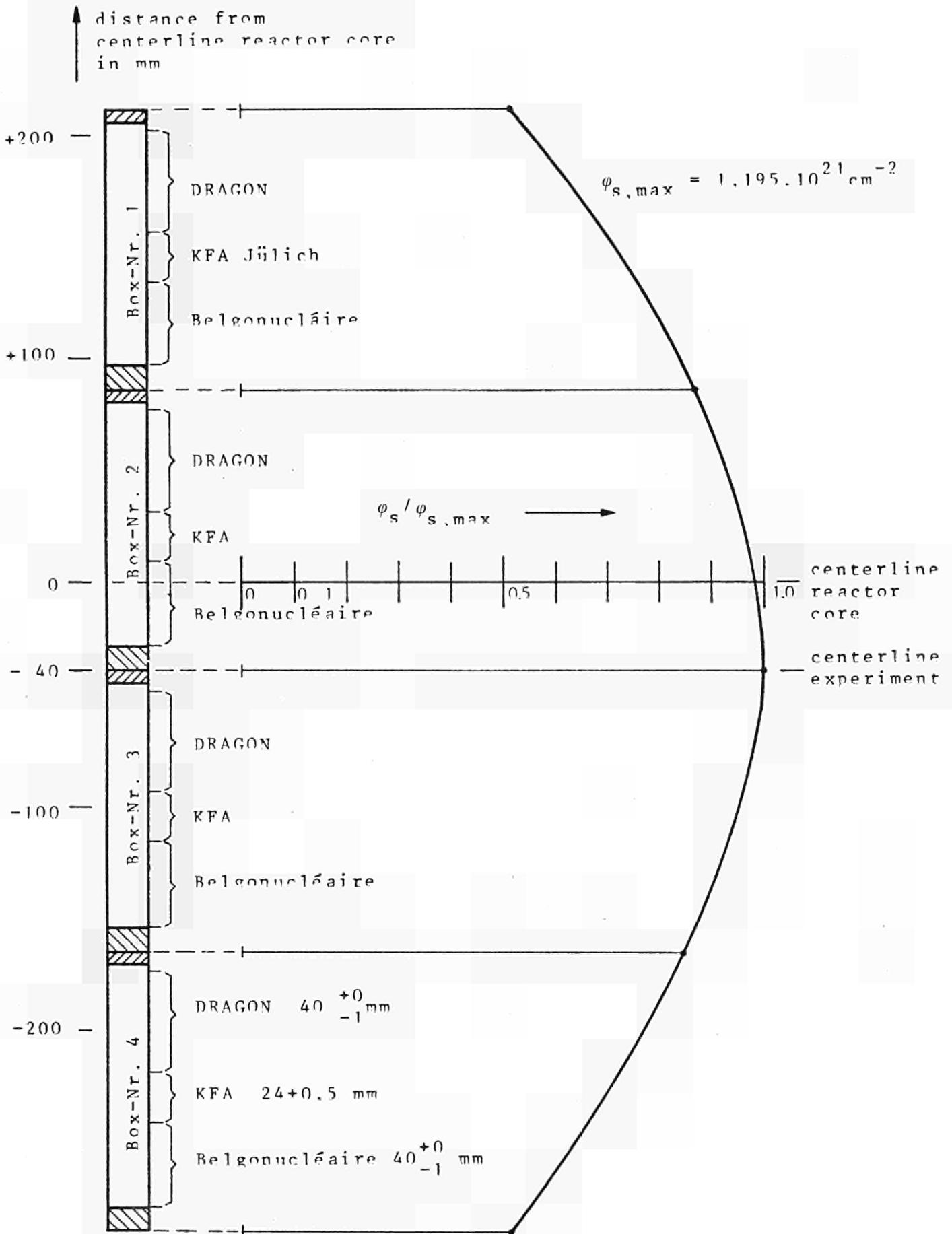
Fig. 24a Relative vertical fast fluence distribution  $\phi_s / \phi_{s,max}$  in position E3 after 72.4 days of irradiation [Ref. 6]
