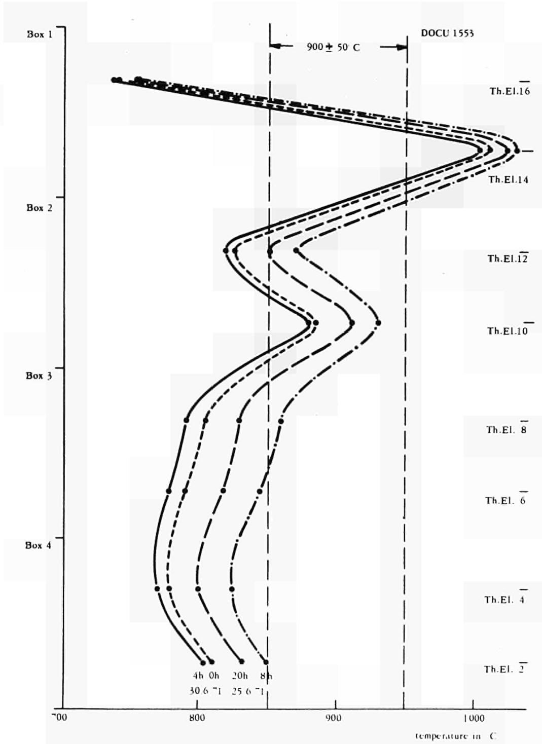
Fig. 13 Vertical temperature distribution measured with the inner thermocouples on June 29th and 30th, 1971, indicating an anomalous behaviour of the capsule (see 3.2.1)
