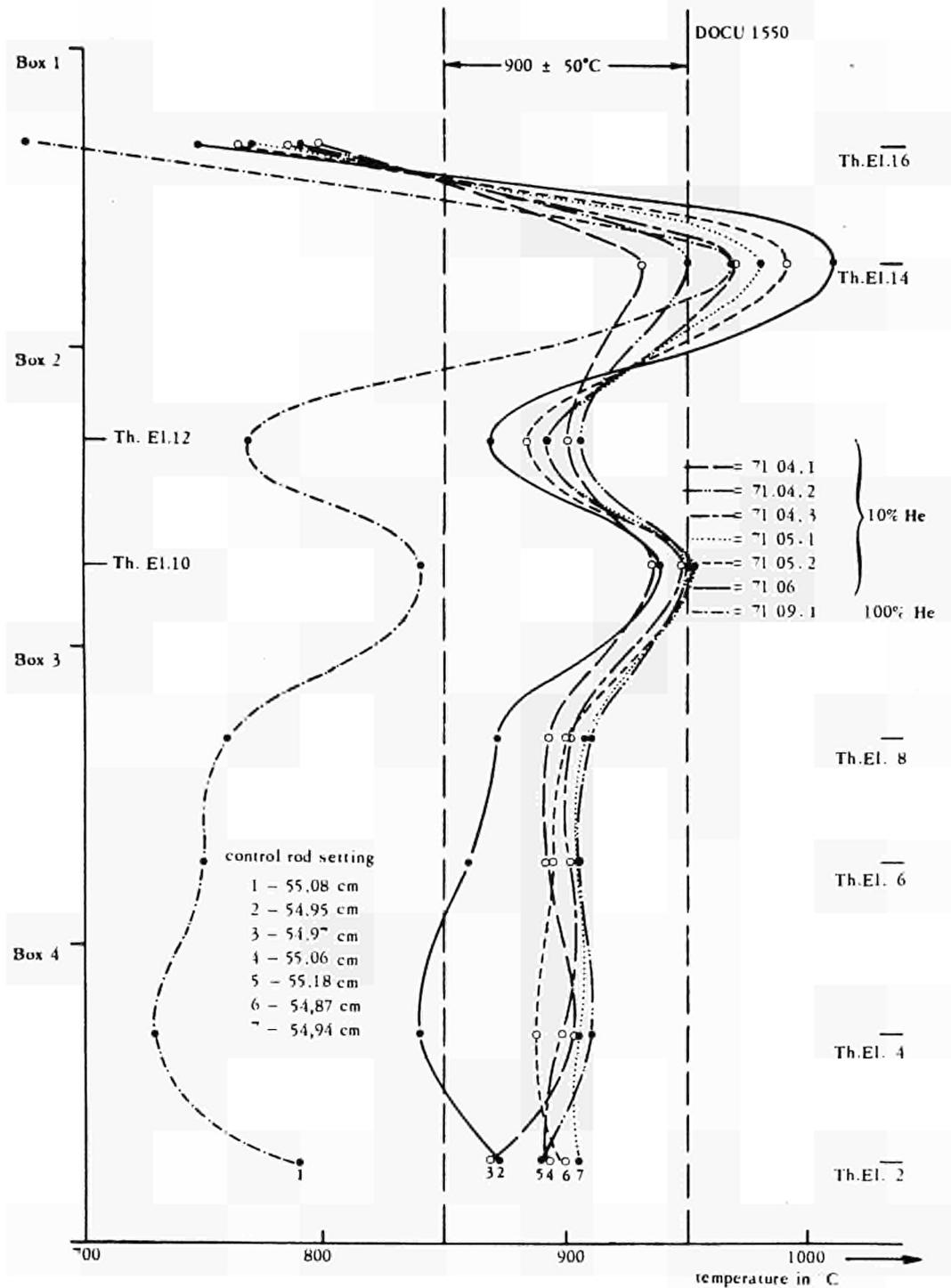
Fig. 10 Vertical temperature distribution measured with the inner thermocouples at mid-cycle (control rod setting about 55 cm) of each irradiation cycle. Gas mixture in outer capsule: 90% N<sub>2</sub> + 10% He (cycle 71.09.1 only 100% He).
