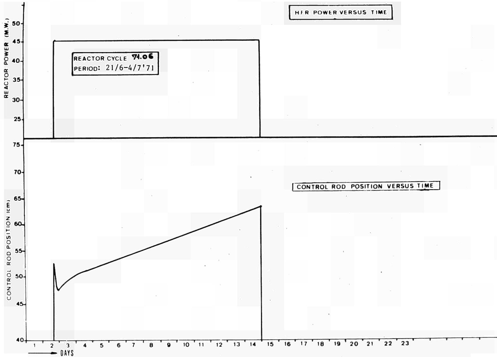
Fig. 22 HFR power and control rod position vs. time. HFR-cycle 71.06
