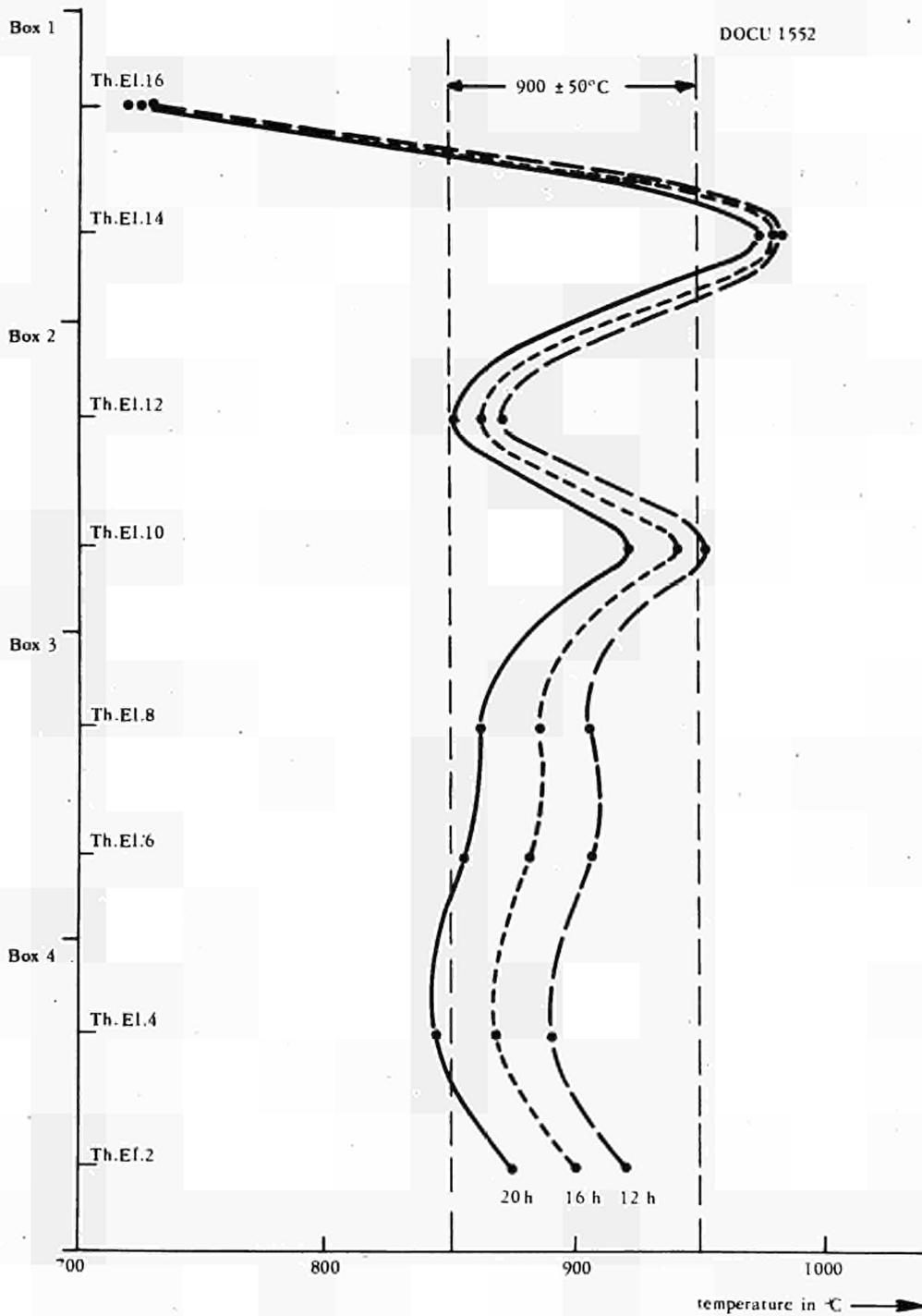
Fig. 12 Vertical temperature distribution measured with the inner thermocouples on June 26th, 1971, indicating an abnormal behaviour of the capsule (see 3.2.1)
