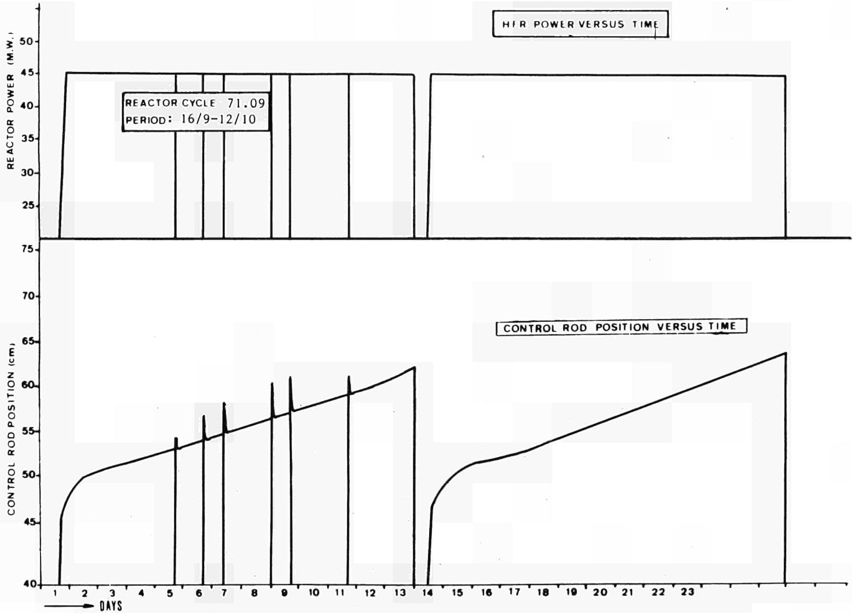
Fig. 23 HFR power and control rod position vs. time. HFR-cycle 71.09
