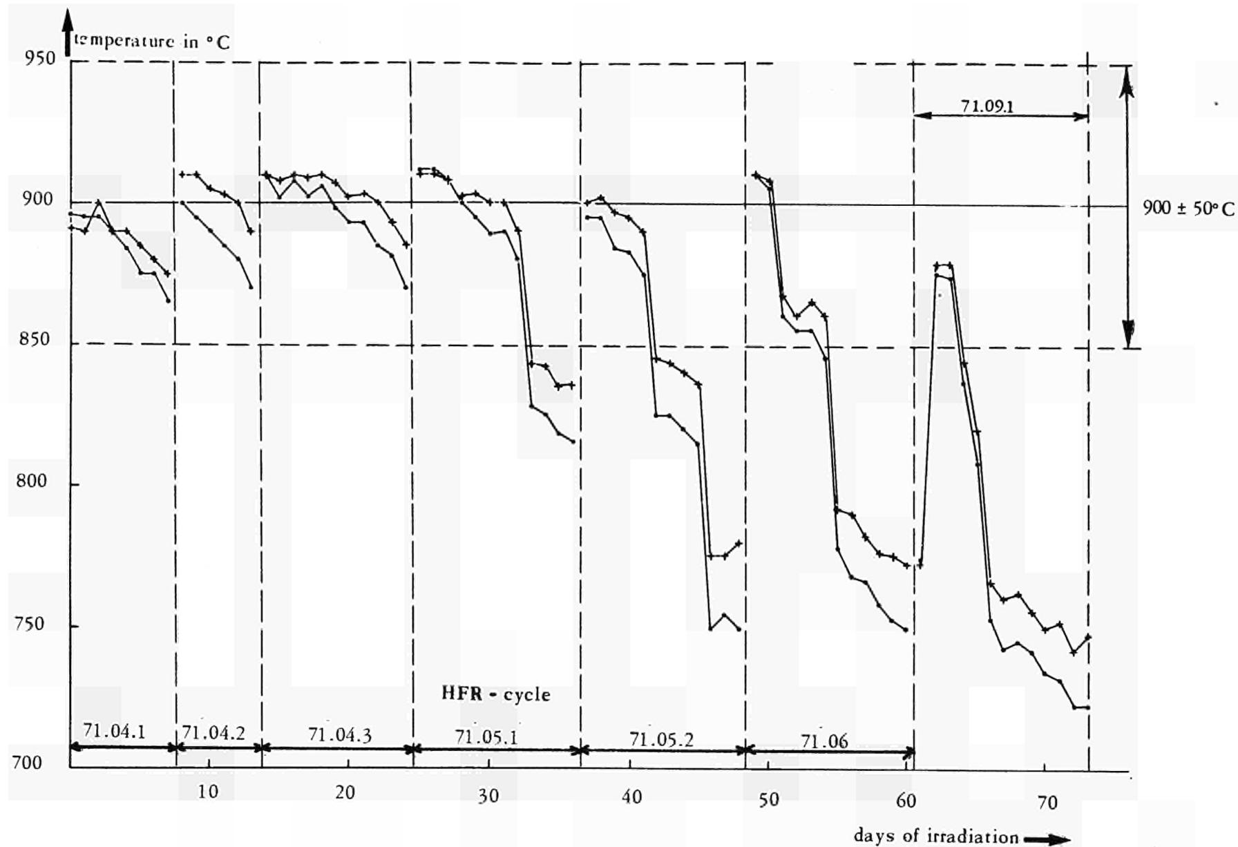
Fig. 18 Graphite-box-nr. 4 : Temperatures measured with the thermocouples nr. 2 and 4 (see Fig. 9) as a function of the irradiation days
