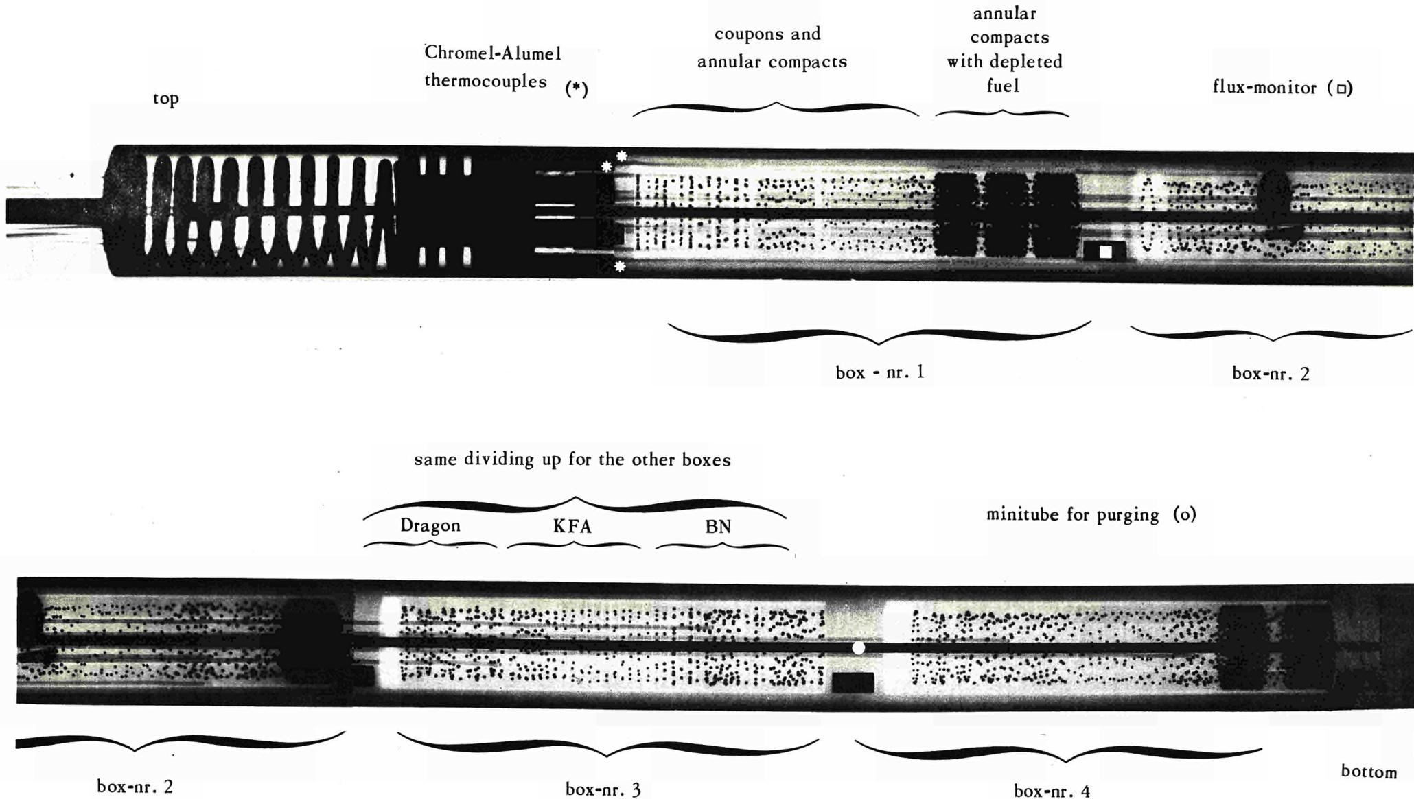
Fig. 8 Panoramic x-ray of 900°C HFR-rig (E96 - 1) before irradiation
