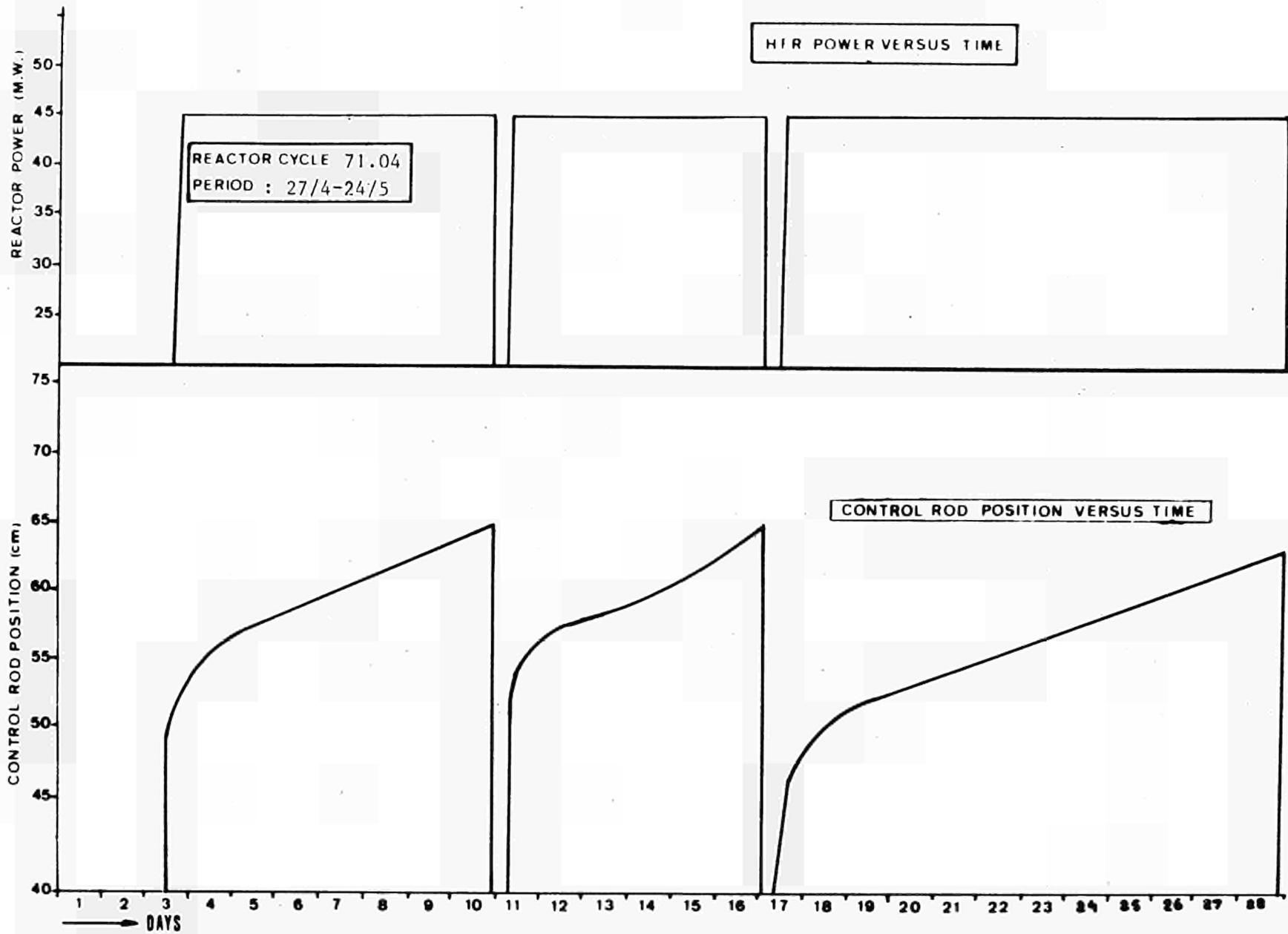
Fig. 20 HFR power and control rod position vs. time. HFR-cycle 71.04
