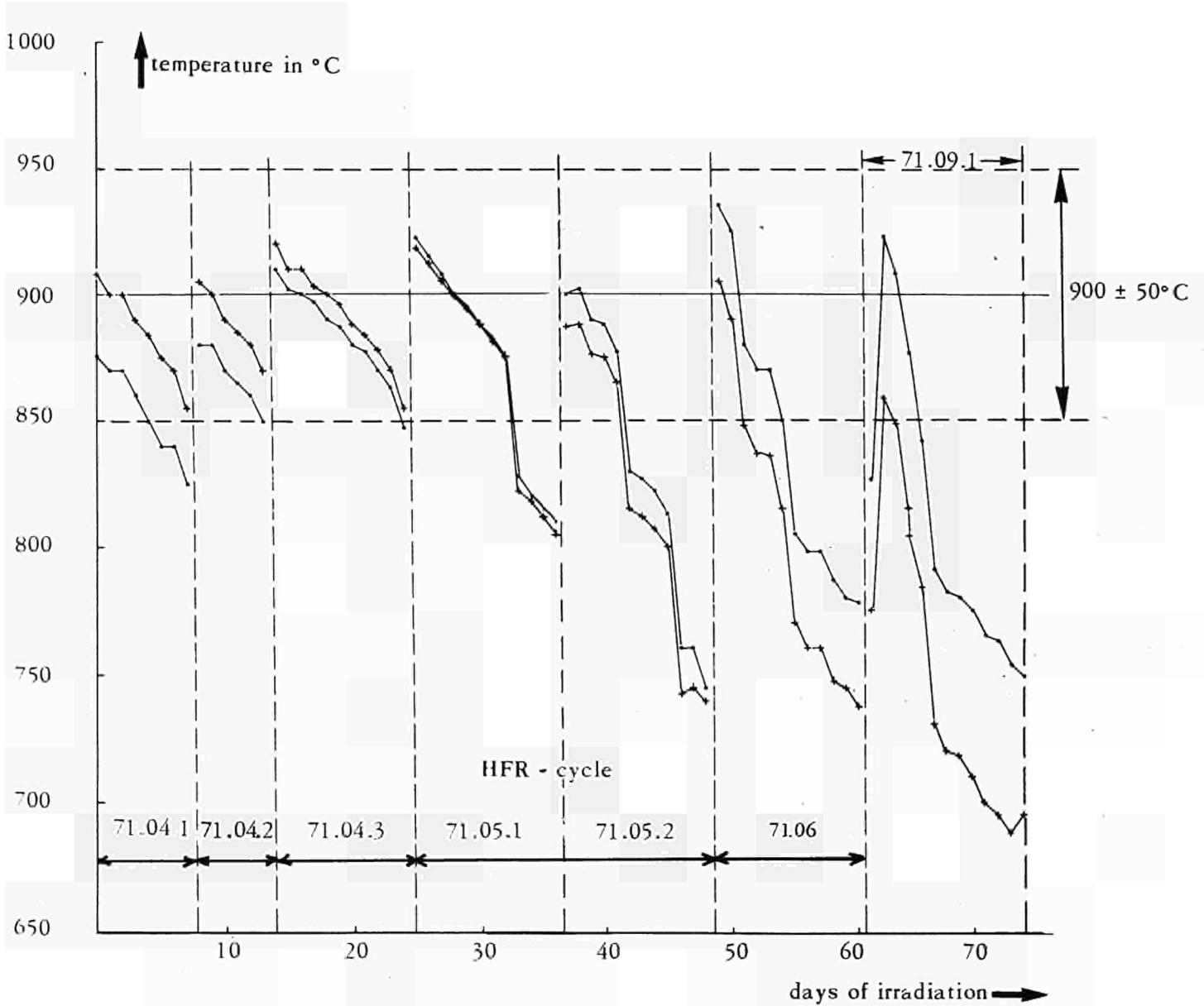
Fig. 17 Graphite-box-nr. 3: Temperatures measured with the thermocouples nr. 6 and 8 (see Fig. 9) as a function of the irradiation days
