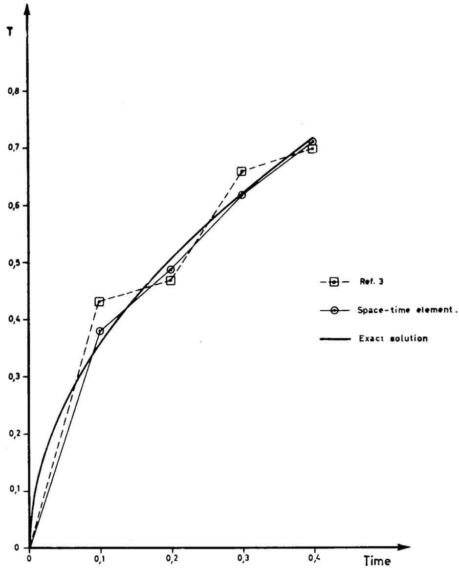
Fig. 2 Temperature distribution versus time at the surface of a semi-infinite solid.
