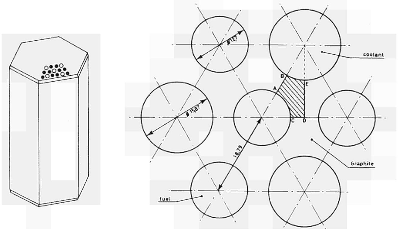
Fig. 4 Graphite matrix of a HTGR fuel element and symmetric cell.
