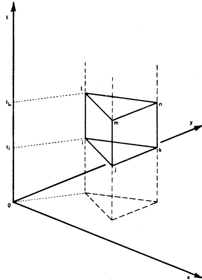
Fig. 1 A right triangular prism in the  $(x,y,t)$  domain.
