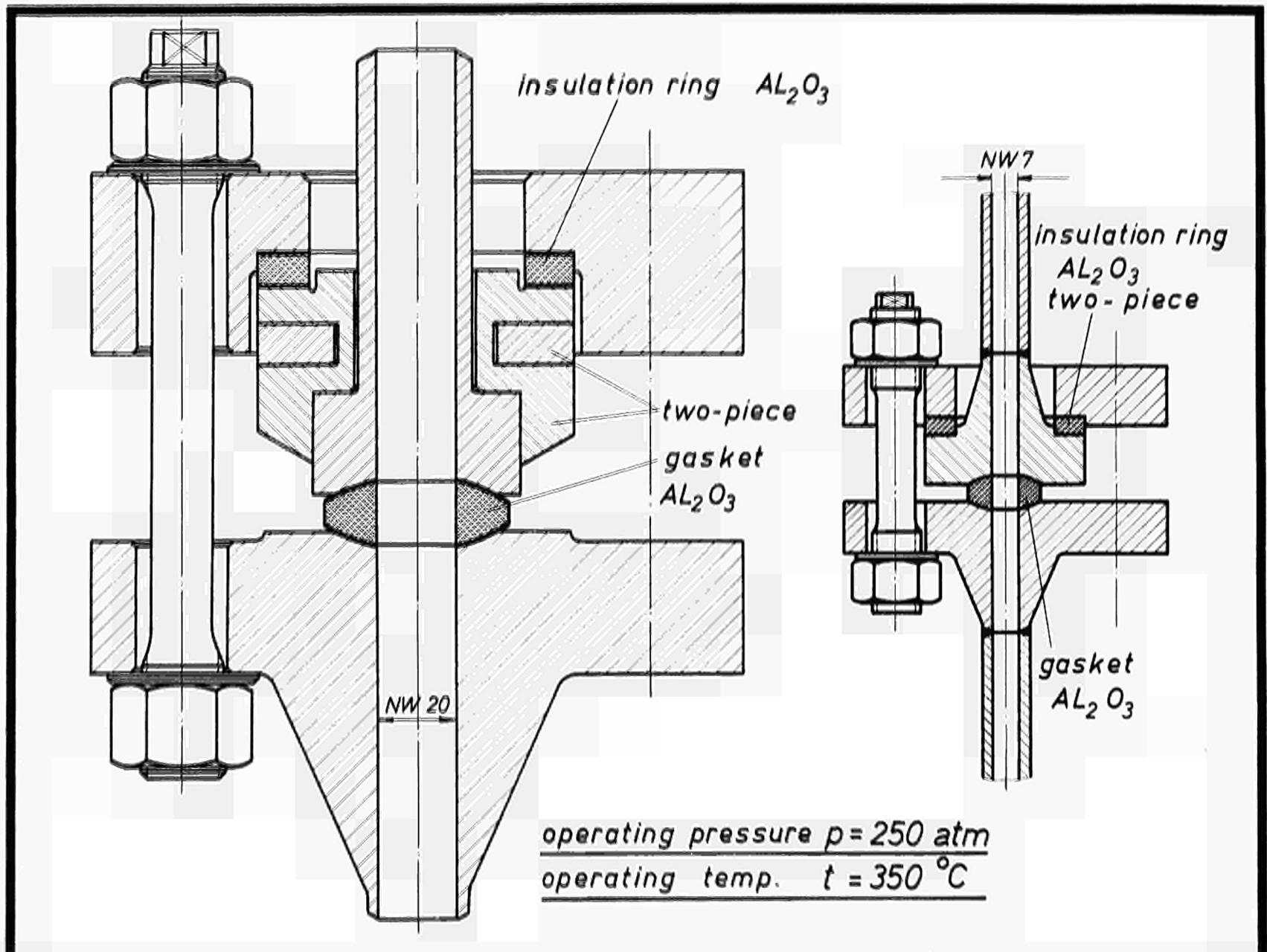
*Fig. 9 Electrical flange insulation*
