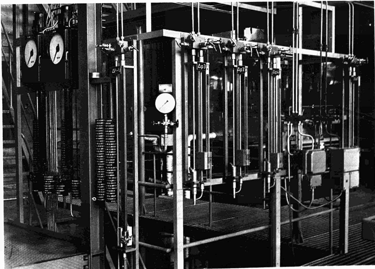
Fig. 8 Massflow- and pressure measuring instruments
