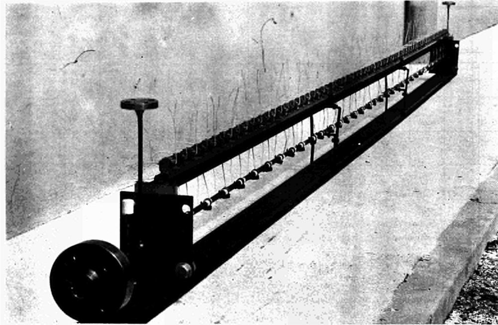
Fig.13 Test section for investigation of the heat transfer to water at high pressures ( $d_o = 14\text{ mm}$ ,  $d_i = 10\text{ mm}$ ,  $l_h = 5100\text{ mm}$ )
