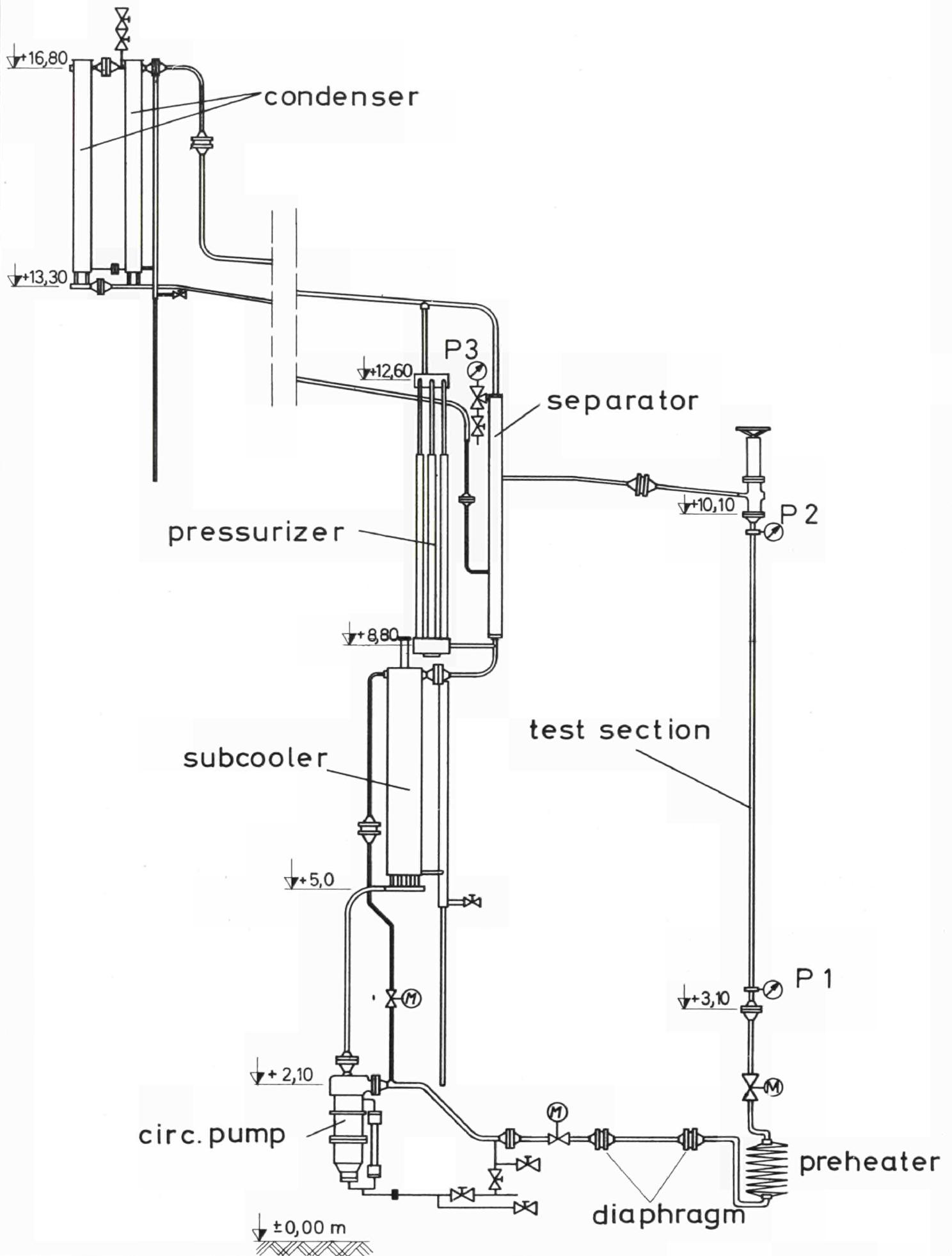
Fig.1 High pressure boiling water loop
