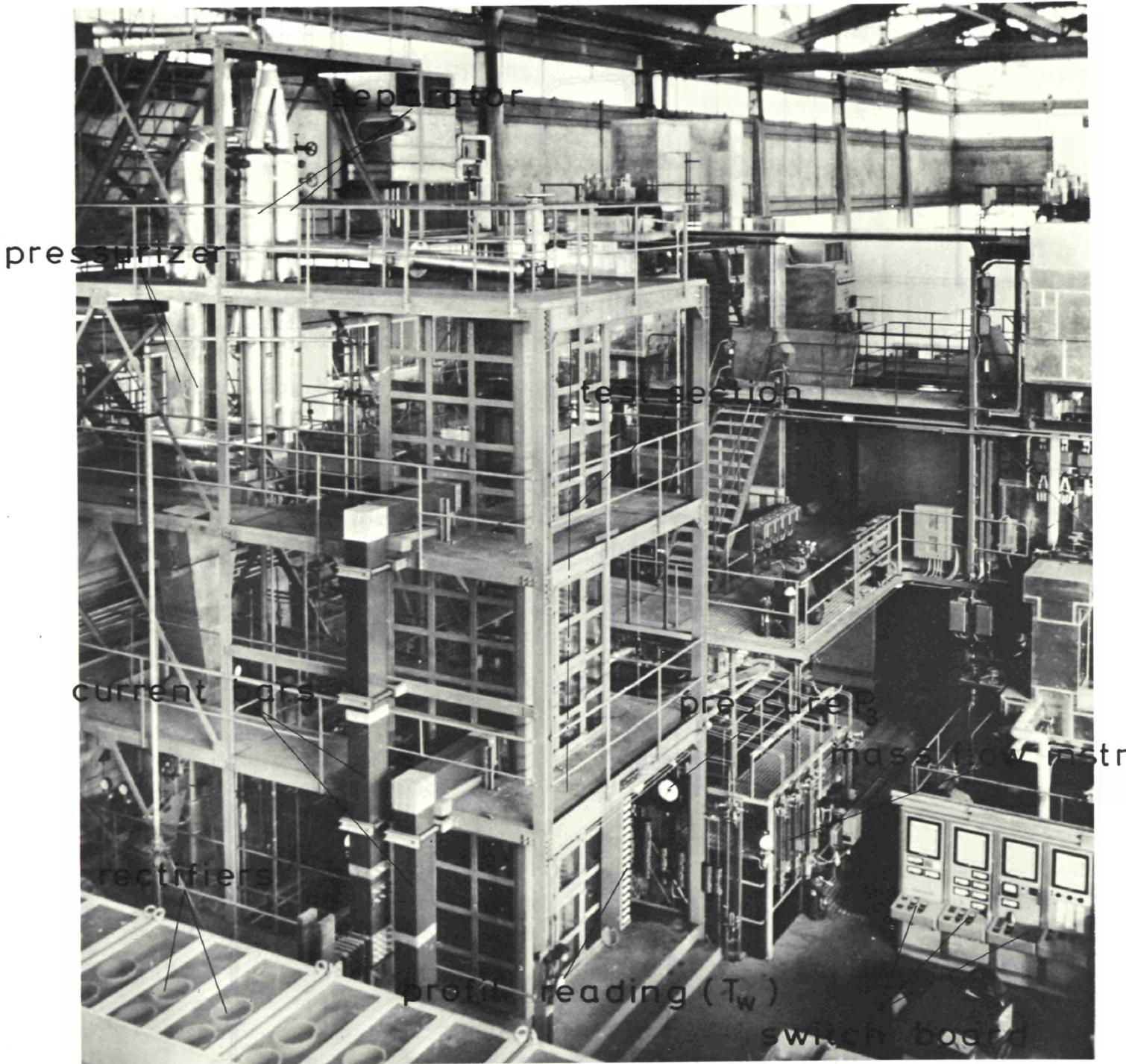
Fig. 2 View of the high pressure boiling water loop
