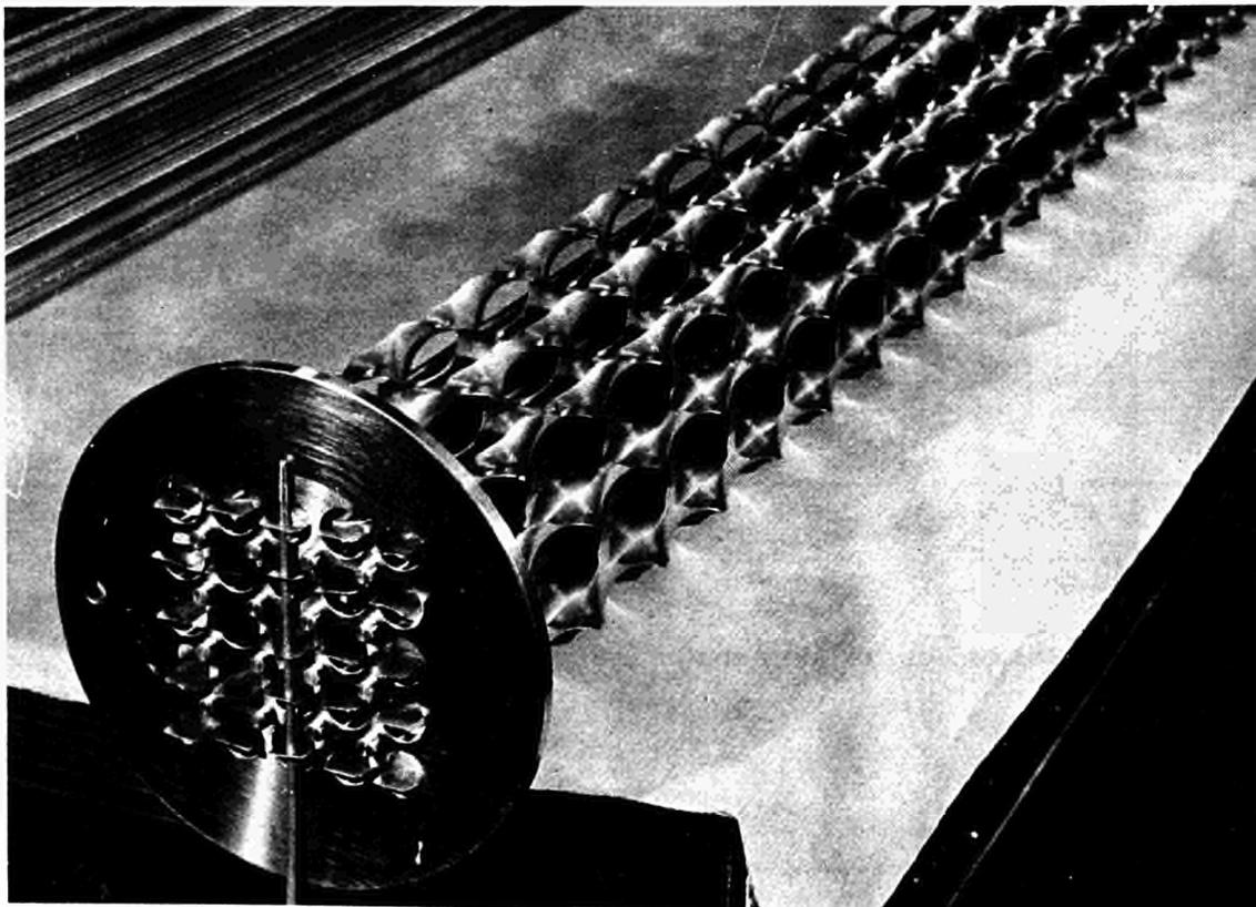
Fig.14 Rod bundle with twisted tapes (SNECMA)
