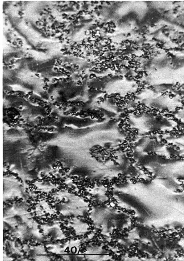
Fig. 13 The segregation of insoluble particles by the mesophase transformation in a briquette pitch. a) Pyrolyzed to 466°C / 820x, Crossed polarizers. b) Pyrolyzed to 489°C / 820x, Parallel polarizers.
