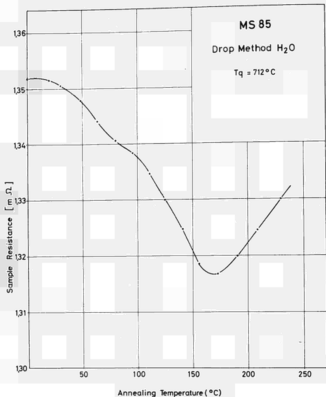
Fig. 8 : Change of the electrical resistance of a Ms - 85 sample quenched by the drop method from 712° C into water ( 18° C ) during isochronal ( 15' ) annealing.
