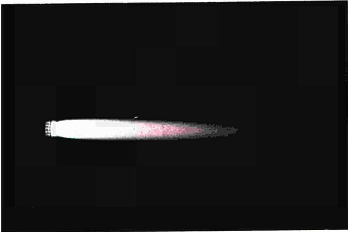
Fig. 4 : Appearance of the normal Air/C<sub>2</sub>H<sub>2</sub> flame
