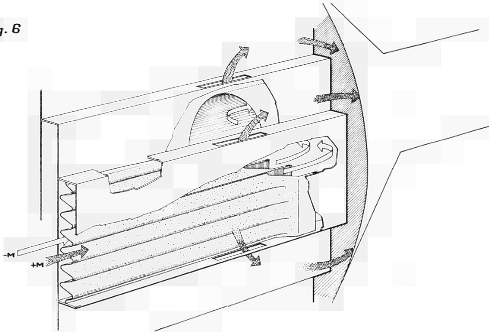
*Detail of the plate heat exchanger*
