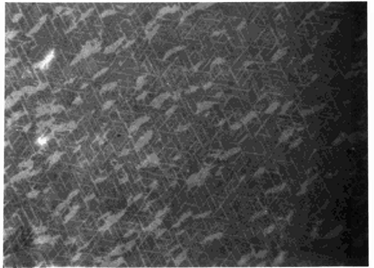
l) \text{U}_4\text{O}_9 bright regions, precipitations in the \{111\} plane, \text{O}/\text{U} = 2.056 ( \times 400 )
