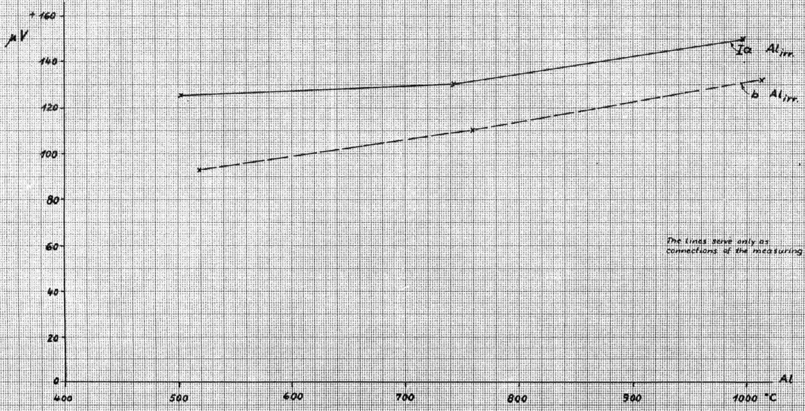
EMF of Alumel irradiated against Alumel unirradiated pair (curve b after annealing)
