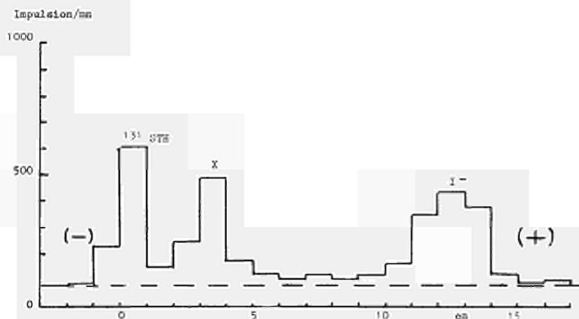
FIGURE 1. — Radioelectrophoretogram of iodination products of a human growth hormone preparation
