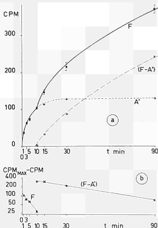
FIGURE 4. — <sup>125</sup>I-insulin binding ( $F$  in  $cpm/P^{2/3}$ ) in respect to dipping time (min). In the upper part of the graph are indicated the evolution of the rapid ( $A'$ ) and the slow ( $F-A'$ ) association processes. In the lower part of the graph are plotted the semilogarithmic lines representative of these inverse exponential processes. Given figures are the mean and S.E.M.
