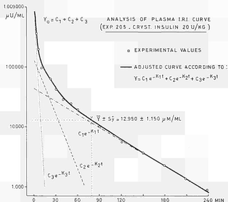
FIGURE 6. — Multiexponential analysis of a disappearance curve of unlabelled insulin after intravenous injection of crystalline insulin.
