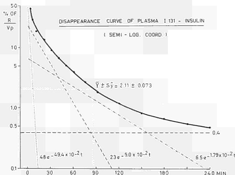
FIGURE 3. — Semi-logarithmic representation of a disappearance curve of plasma  $^{131}\text{I}$ -insulin (Figure 1). Results of the multiexponential analysis are indicated in the lower part of the graph.
