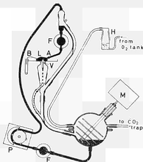
Diagram of the apparatus used for liver perfusion
