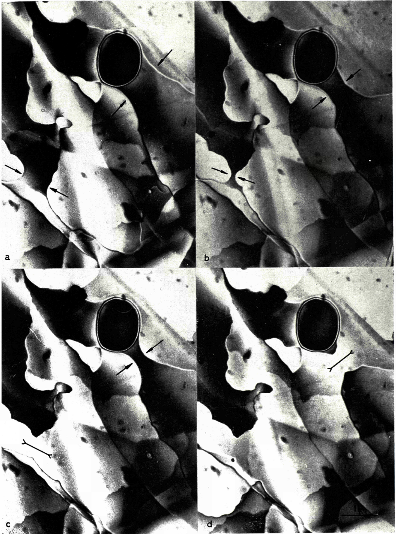
Fig. 3 — Peripheral part of a brominated graphite crystal showing regions exhibiting a mosaic of stacking fault contrast, boundary dislocations and the mechanism of the formation of typical configurations of concentric bromine loops one above the other in different planes.
