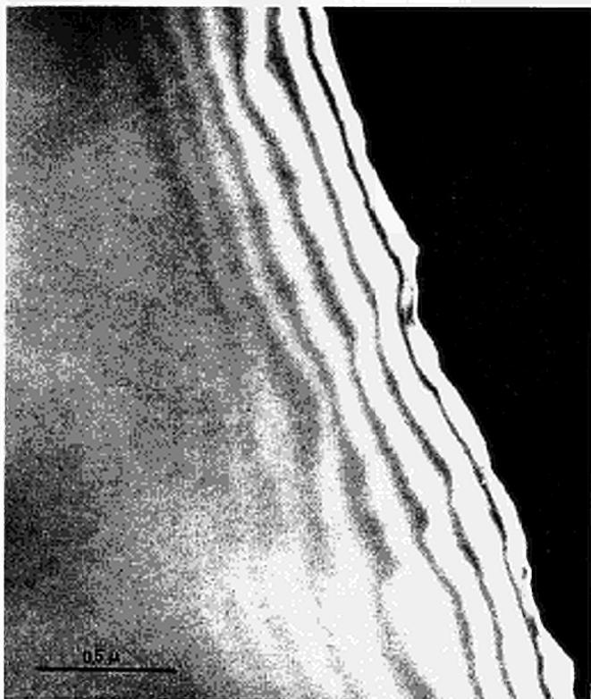
FIG. 1. Dark field picture of a crystal wedge. The diffraction vector operating is  $\vec{g}=[220]$ ,  $t_{220}=330$  Å. One can easily count seven extinction contours which correspond to more than 2000 Å thickness at the thick part of the wedge.
