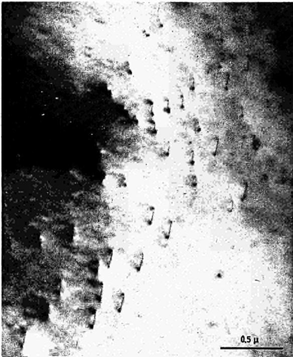
FIG. 6. Dislocations lying steeply inclined to the plane of the foil. Area near a crack which has been produced in a thick part of the specimen by manipulating the electron beam.
