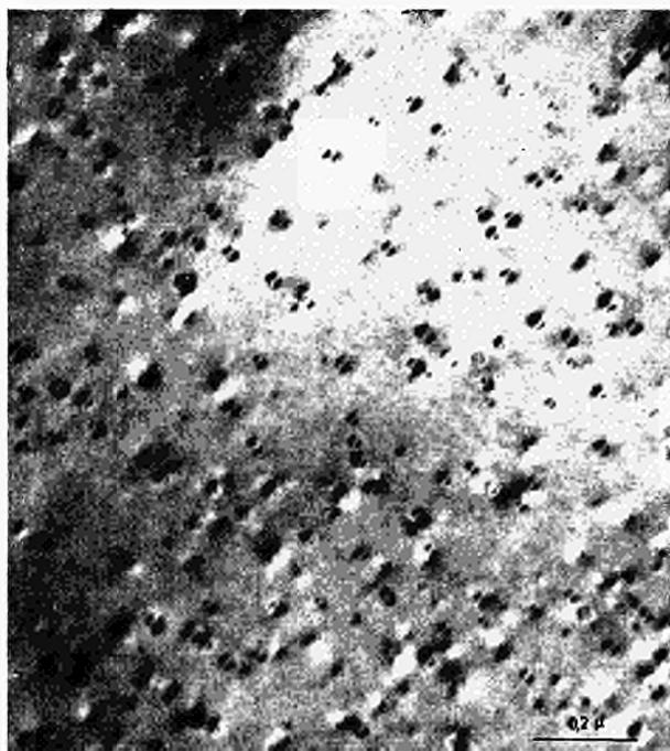
FIG. 2. Pattern of precipitates in a nonannealed crystal.
