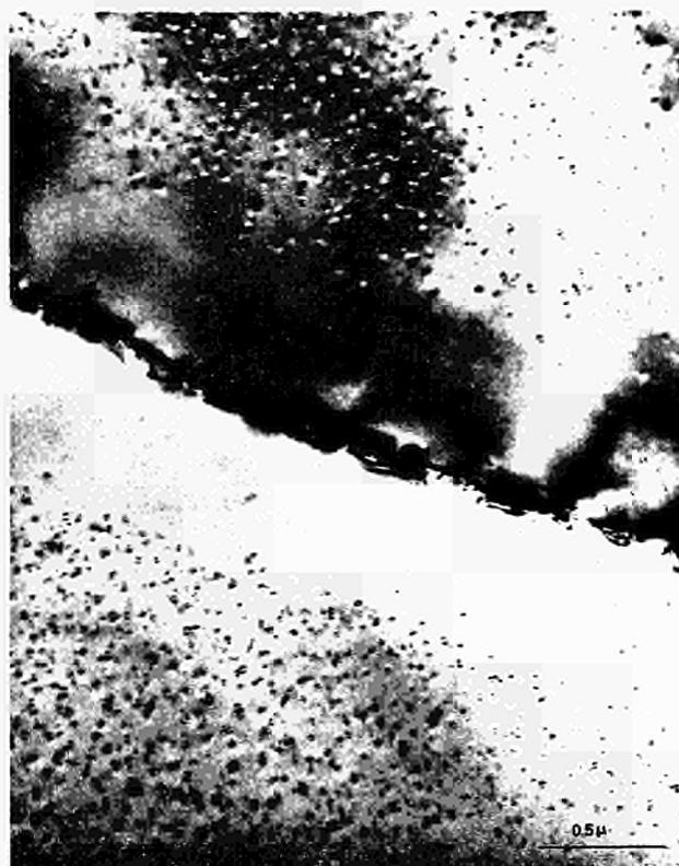
FIG. 3. Absence of precipitates near a small angle boundary decorated by bigger precipitations.
