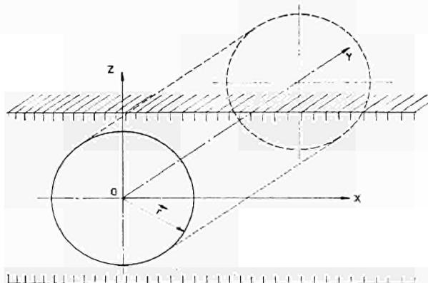
FIG. 17. The coordinate system for the displacement function of a fission track that lies parallel to the surface of the foil.
