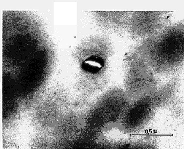
FIG. 5. Large single loop in crystal foil, irradiated up to  $10^{16}$  nvt (thermal).
