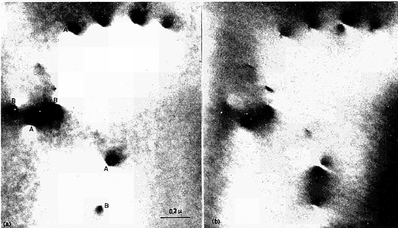
FIG. 8. Dislocations seen end-on in an area which had been thinned with the electron beam by evaporating part of the  $\text{UO}_2$ . (a) Bright field image. Dislocations denoted by A have opposite Burgers vectors with respect to those denoted by B. (b) Dark field image with  $g=[331]$  (two-beam case). Some of the dislocations show noncomplementary contrast in the dark field due to anomalous absorption.
