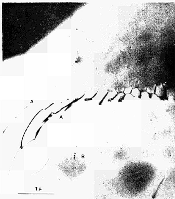
FIG. 13. Interaction between fission tracks and dislocations. At AA a fission fragment probably has cut through two dislocations of the small angle boundary. At B a track decorated by dots showing decreasing distances can be seen.
