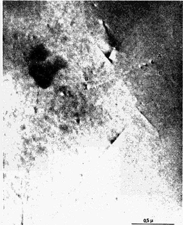
FIG. 11. Varying contrast of fission tracks due to different orientation of tracks with respect to diffraction vector  $g$ .  $g$  is parallel to the line of the scale indicator. The track denoted BB lies nearly parallel to  $g$  and, therefore, is almost out of contrast. Tracks roughly at right angles to  $g$  show strong contrast.
