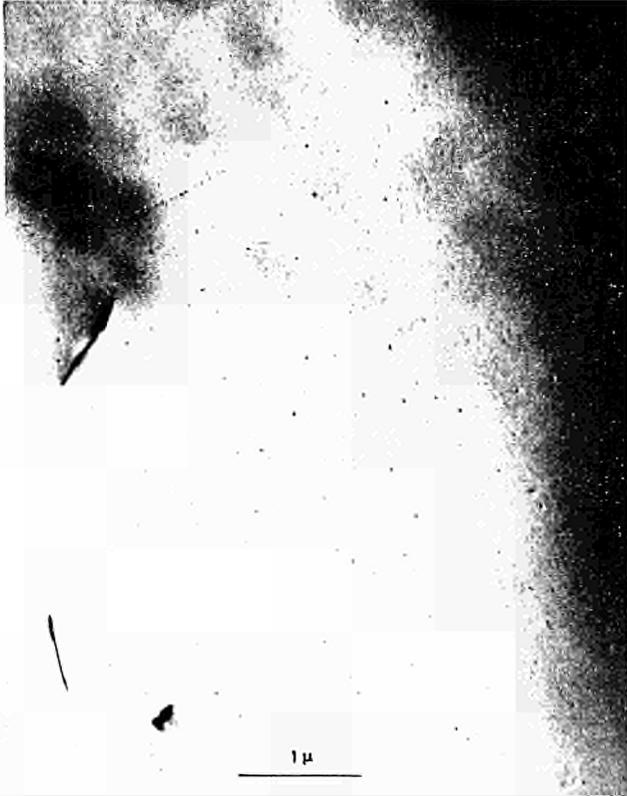
FIG. 10. Aspect of crystal foil 1000 Å thick after irradiation with nearly  $10^{15} \text{ nvt}$  (thermal). Nondecorated and decorated fission tracks, black dots, and short segments of dislocations are visible.
