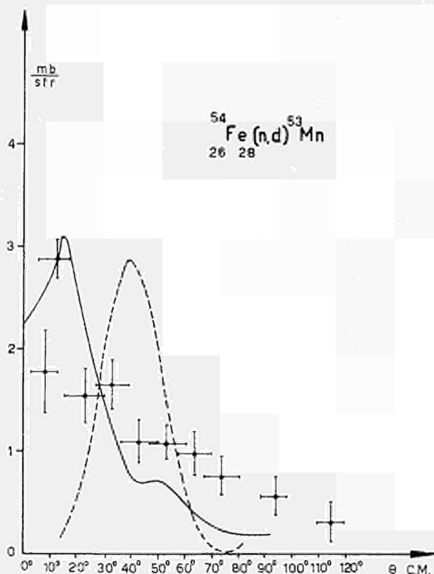
Fig. 2. Angular distributions of deuterons of maximum energy from the  $Fe^{54}(n, d)Mn^{53}$  reaction. Points are experimental results. Bars on each point show the statistical errors. The dotted curve is calculated by Satchler using a distorted wave-Born approximation and assuming transferred angular momentum  $l = 3$ . The curve drawn in full is obtained taking 68% of  $l = 1$  transition plus 32% of  $l = 3$ .
