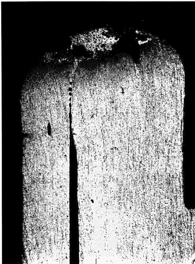
Fig. 4 - Undegassed S.A.P. after electron beam welding - Otto Fuchs material. ( \times 25 )
