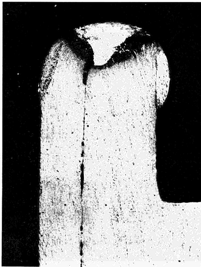
Fig. 14 - End-plug type a - welding of S.A.P. Montecatini 895 degassed 24 hrs at 625^{\circ}\text{C} . ( \times 25 )
