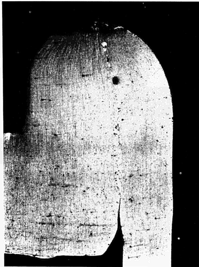
Fig. 10 - End-plug type a - welding of S.A.P. Montecatini 960 undegassed. ( \times 25 )
