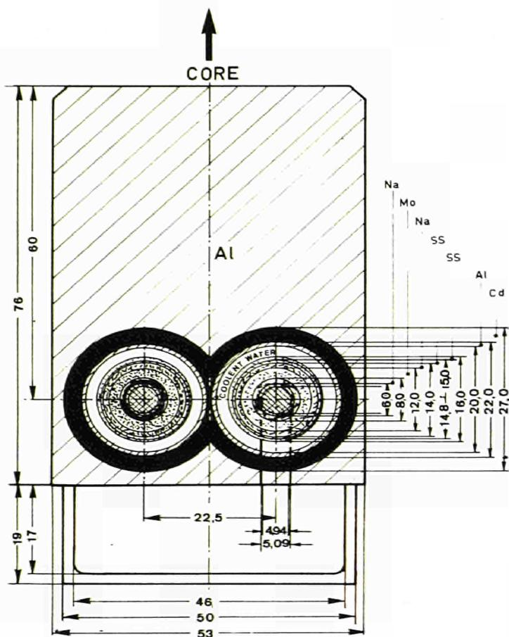
Fig. 2.50 LMBFR fuel testing. PSF capsule for power ramping of long pre-irradiated fuel pins. Horizontal section.
