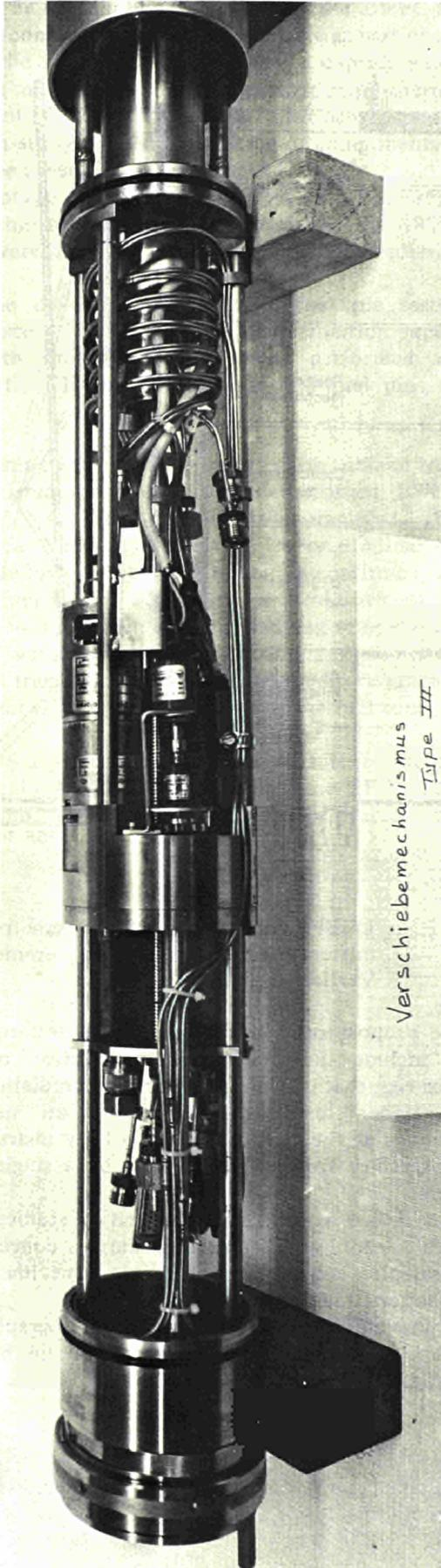
Fig. 2.49 Modified Trio Rig Head with Vertical Displacement Unit (VDU) and Central Instrument Lead Outlet.
