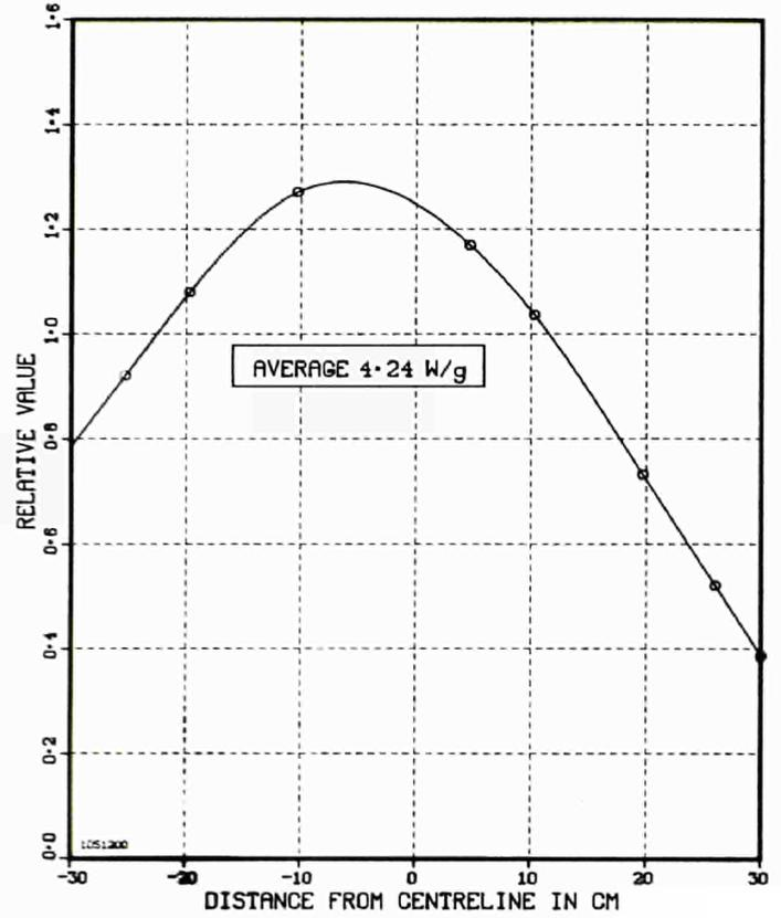
Fig. 2.19 Nuclear heating in graphite. Small samples in position F2.
