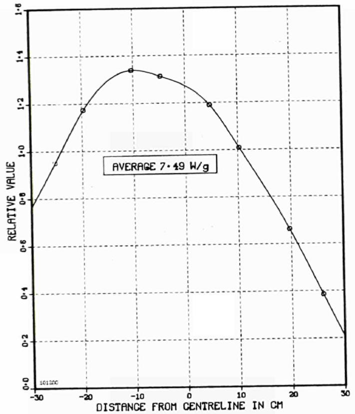
Fig. 2.16 Nuclear heating in graphite. Small samples in position C7.
