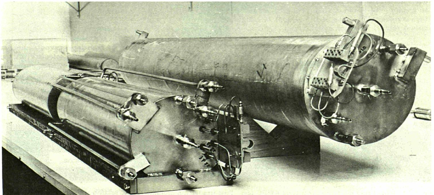
Fig. 2.55 Sweep loops. Filter units after assembly.
