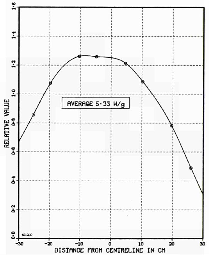
Fig. 2.17 Nuclear heating in graphite. Small samples in position G3.
