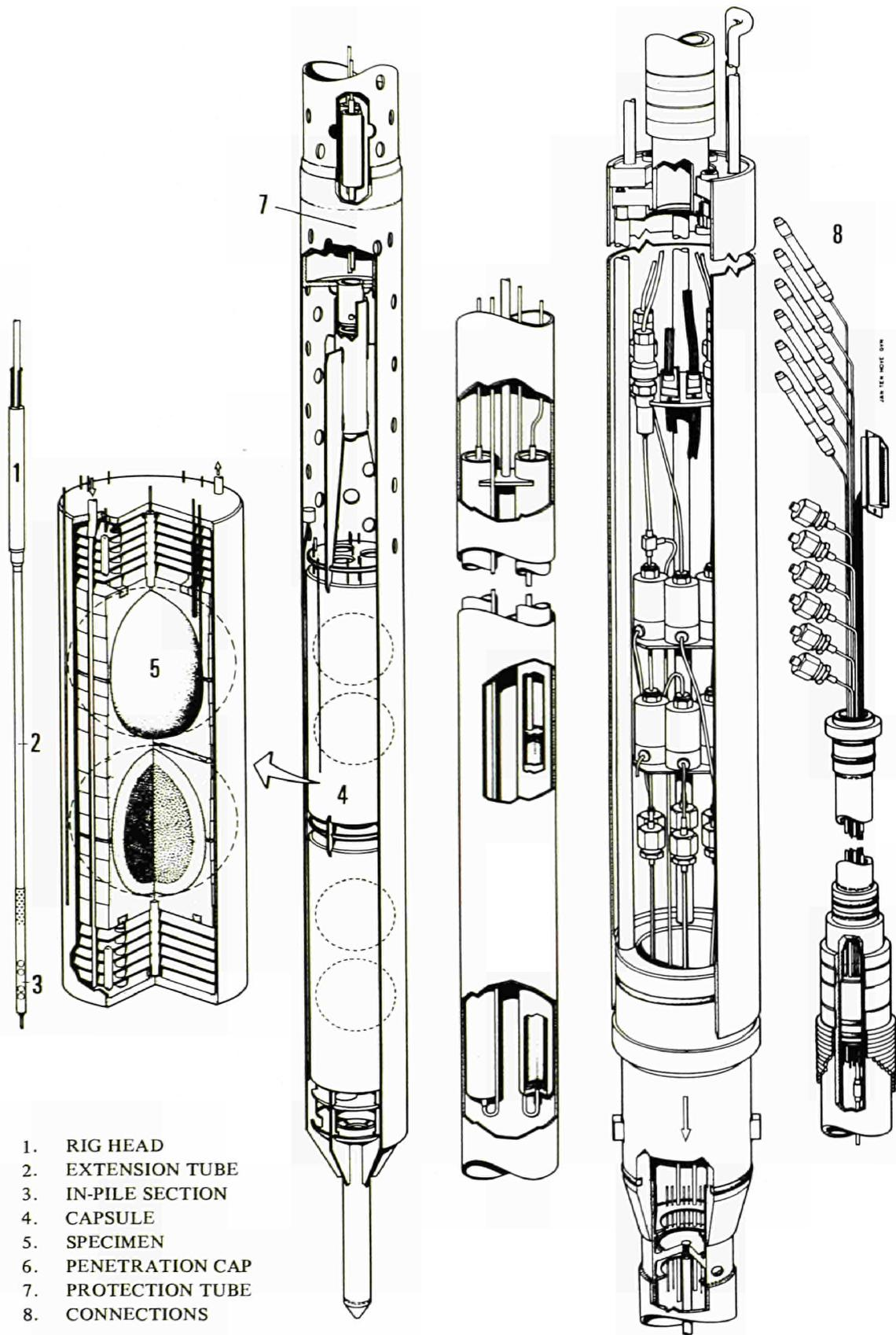
Fig. 2.28 Irradiation device for special HTR fuel element testing.
