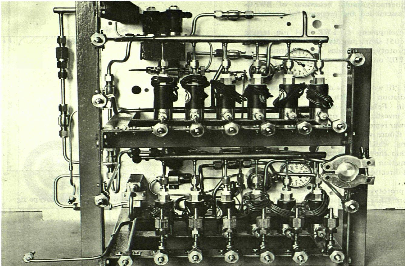
Fig. 2.54 Sweep loops. Katharometer panel during assembly.
