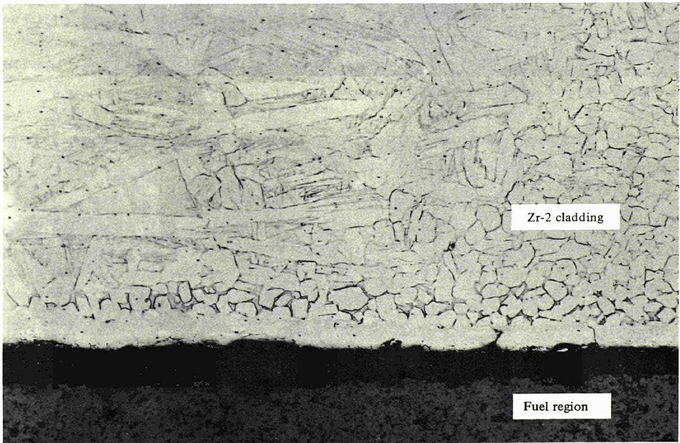
Fig. 2.53 Failed fuel pin from prototype BWFC test. Post-irradiation metallographic section showing transition zone in clad structure. Magn. x 250.
