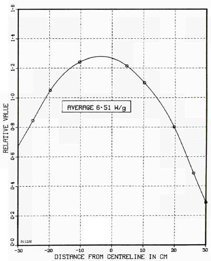
Fig. 2.18 Nuclear heating in graphite. Small samples in position G5.
