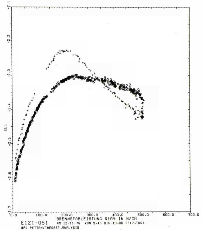
Fig. 2.52 Elongation measurement on prototype rig BWFC-RL.
