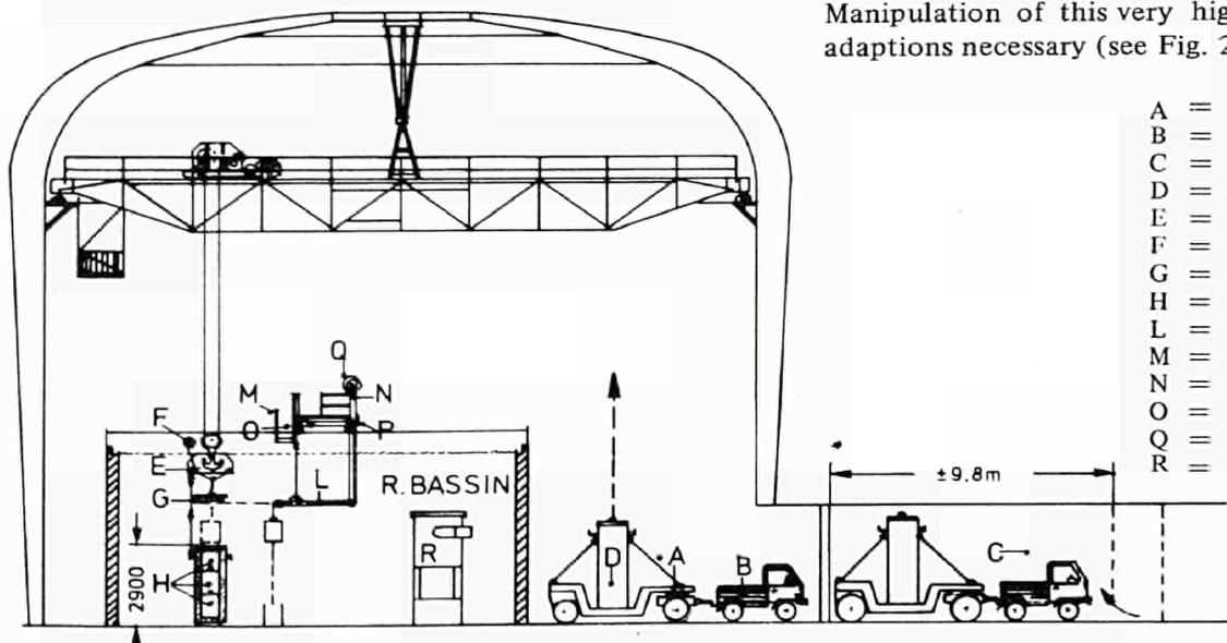
Fig. 2.12 New type transport container. Handling scheme.
