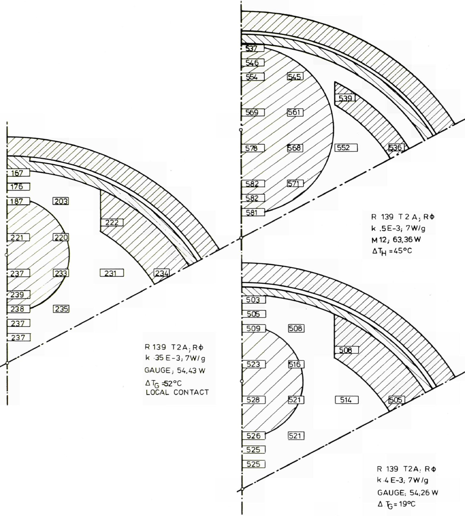
Fig. 2.30 R139-2A, calculated temperature patterns for head section, gauge section and local contact.
