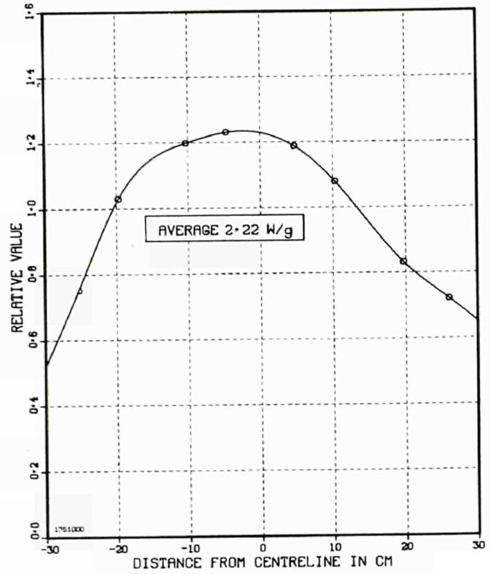
Fig. 2.15 Nuclear heating in graphite. Small samples in position H2.
