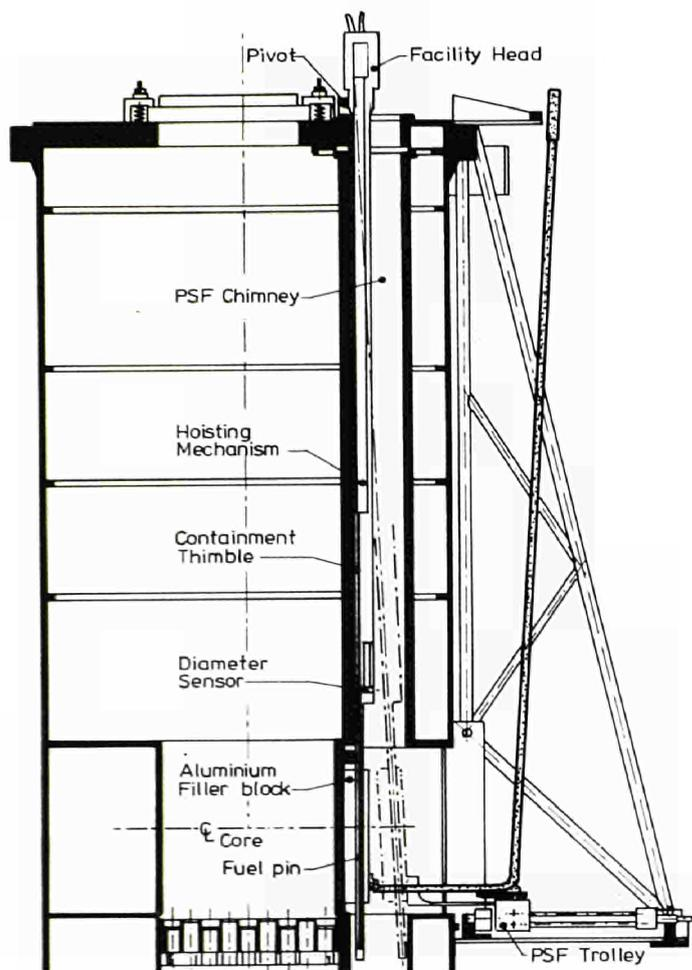
Fig. 2.51 LMBFR fuel testing. PSF capsule for intermittent fuel pin diameter measurement. Vertical section.
