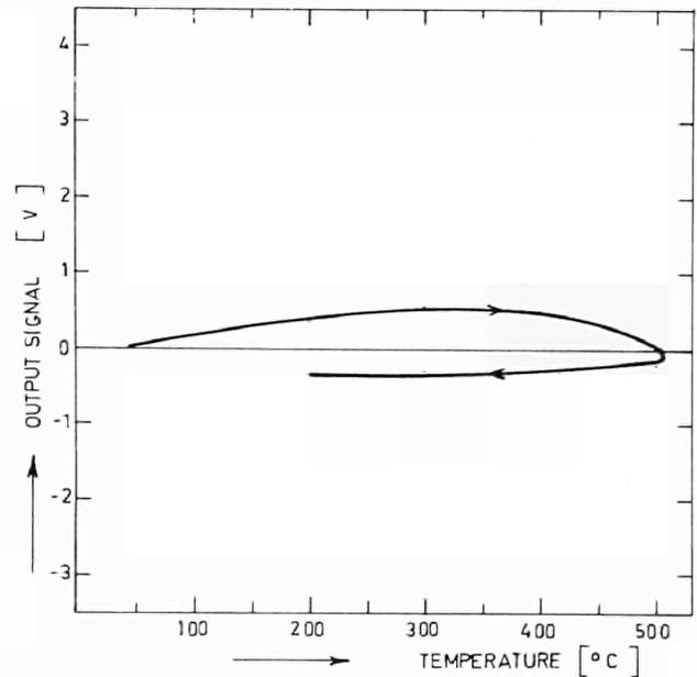
Fig. 2.65 Output signal of the pressure transducer with two Ailtech Type SG-425 strain gages. The sensitivity of the measuring system is 10 times higher than that used in Fig. 2.62. In this case RTC1 = 12.5Ω and RTC2 = 15.0Ω.
