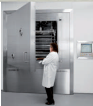
The processing hall contains a new freeze dryer with a 100 kg ice condenser capacity.
