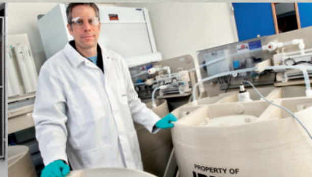
The building contains a new laboratory for producing water reference materials, consisting of 4 x 500 litre drums which can be made into one volume of 2000 litre thanks to the inert pumps that re-circulate water in the system.
