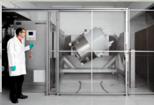
This large-scale mixer in the processing hall can mix powders up to 550 L or 400 kg during reference material preparation.
