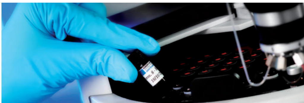
Liquid chromatography – time of flight mass spectrometry is used for metabolomics and food authentication studies.
