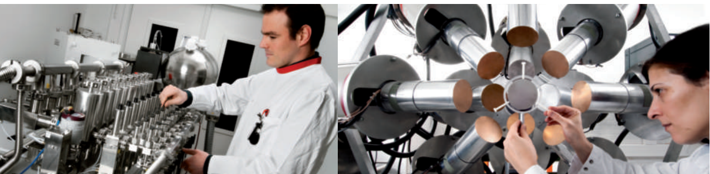
(left): New mass spectrometer for certification of reference materials and nuclear safeguards measurements.
