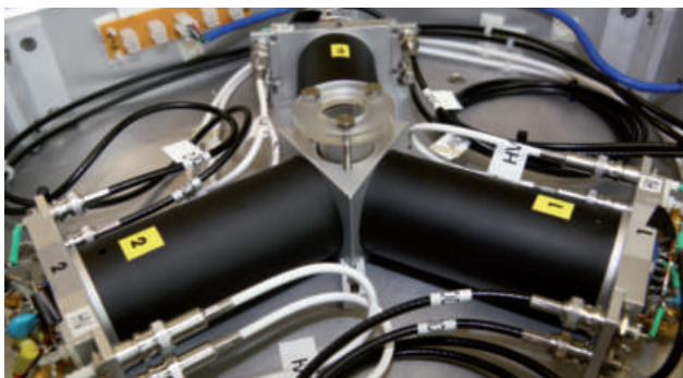
The triple-to-double coincidence ratio (TDCR) liquid scintillation spectrometer.
