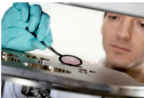
Preparation and characterisation of thin film nuclear targets by vacuum evaporation.
