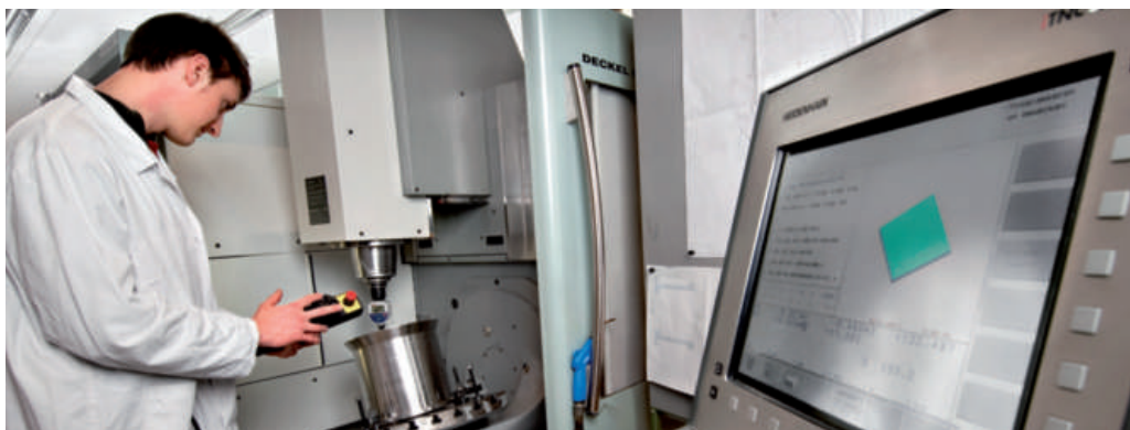
Checking the reference points before operating a milling machine in the workshop.
