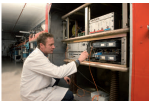
Checking the electronics settings in GELINA's injector pulsing system. During operation, these electronics are working on a hot deck at 80,000 volts above earth potential.
