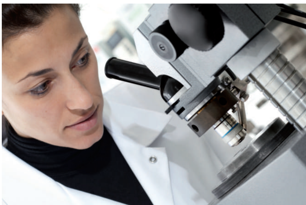
Optical distance measuring device for \alpha -particle counting at a defined solid angle. This is a primary standardisation technique for radioactivity and the determination of nuclear decay data.
