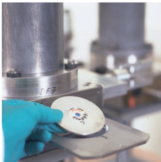
Insertion of a thin, vacuum evaporated source into an \alpha -particle spectrometer.
