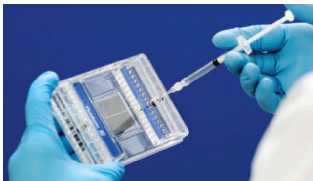
Digital polymerase chain reaction (PCR) for the quantification of a DNA copy number ratio.
