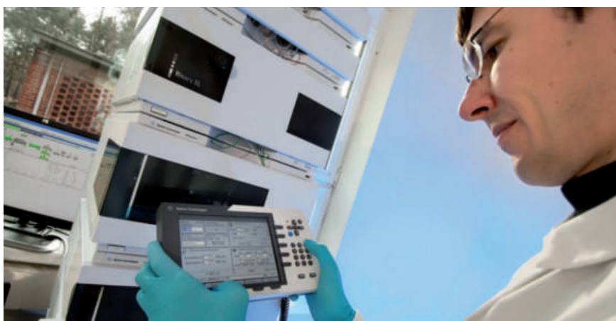
Verification of instrument settings for mycotoxin analysis using high performance liquid chromatography (HPLC).
