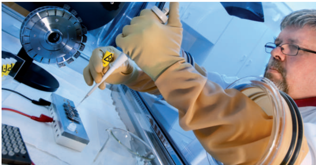
Loading of a solution of certified plutonium isotope reference material for mass spectrometric analysis.
