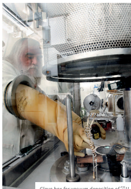
Glove box for vacuum deposition of ^{235}\text{U} .
