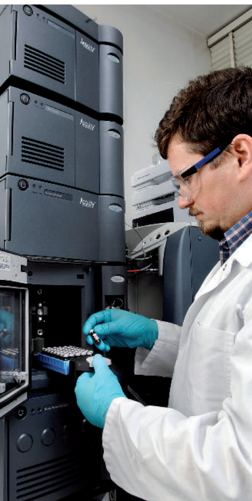
Ultra performance liquid chromatography: loading the autosampler tray.
