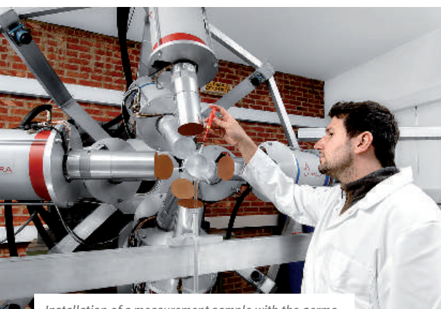
Installation of a measurement sample with the germanium array for inelastic neutron scattering (GAINS).
