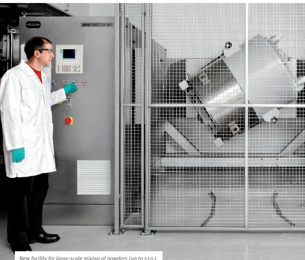
New facility for large-scale mixing of powders (up to 550 L or 400 kg) during reference material preparation.
