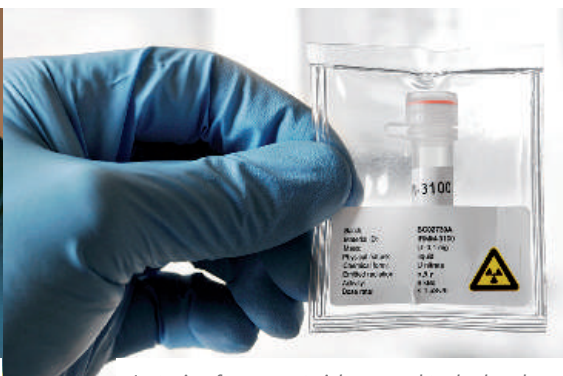
Isotopic reference materials are used to check and account for irradiated nuclear fuel.
