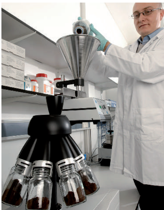
Sample divider for homogenous distribution of material.
