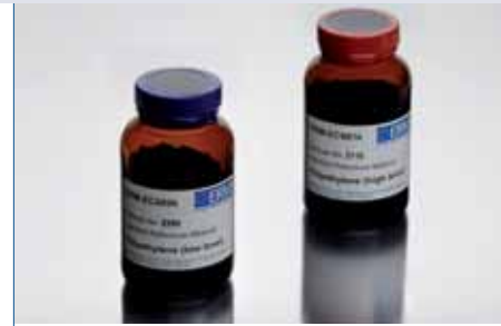
ERM-EC680k and ERM-EC681k are low density polyethylene granulates that can be used for the quality assurance of measurements related to the implementation of the RoHS Directive.
