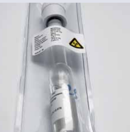
IRMM-086 is a highly enriched ^{239}\text{Pu} spike certified for plutonium amount content and isotopic composition. This isotopic reference material is applied for the quality control of measurements in the nuclear fuel cycle.
