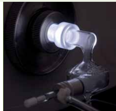
Inductively coupled plasma mass spectrometry (ICP-MS) is commonly used to analyse contents of metals in food and feed samples.
