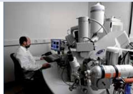
Scanning electron microscopy is used for the characterisation of candidate reference materials.
