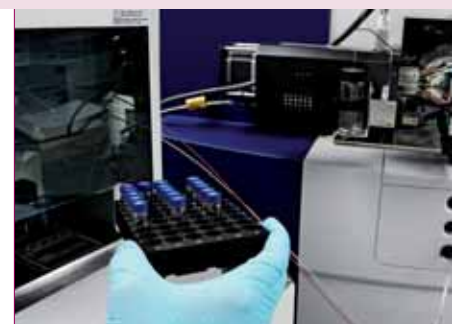
Proteins in complex foodstuffs are analysed with a quadrupole – time-of-flight mass spectrometer.
