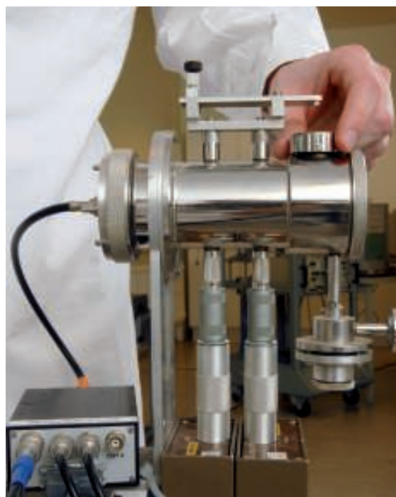
The recoil proton telescope at JRC-IRMM is used for neutron fluence measurements
