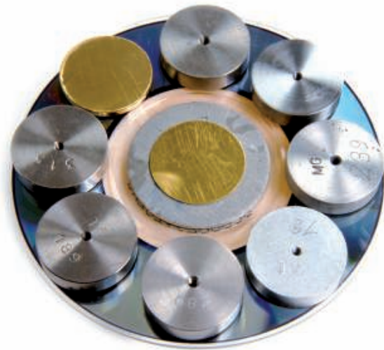
A passive detector used for neutron dosimetry is tested at JRC-IRMM
