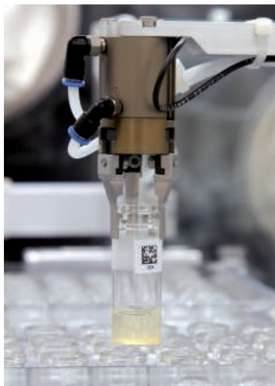
An automated system for dispensing and ampouling of large size dried spikes was installed at JRC-IRMM in 2006
