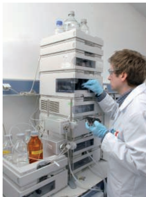
Analysis of PAHs by solid phase extraction high performance liquid chromatography
