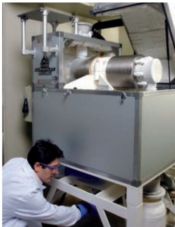
Some candidate reference materials are milled at liquid nitrogen temperature
