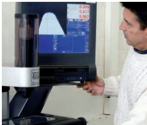
Measuring Charpy specimens
