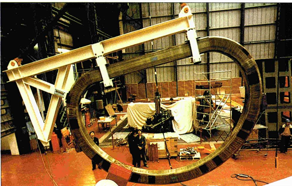
A completed toroidal field coil ready for assembly
