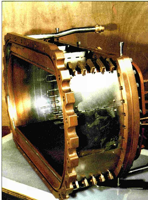
*Neutral injector box being prepared for testing*
