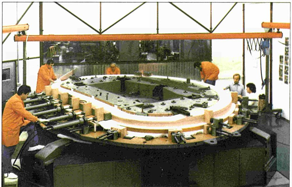
*Winding of the copper conductor into the coil's D-shape*
