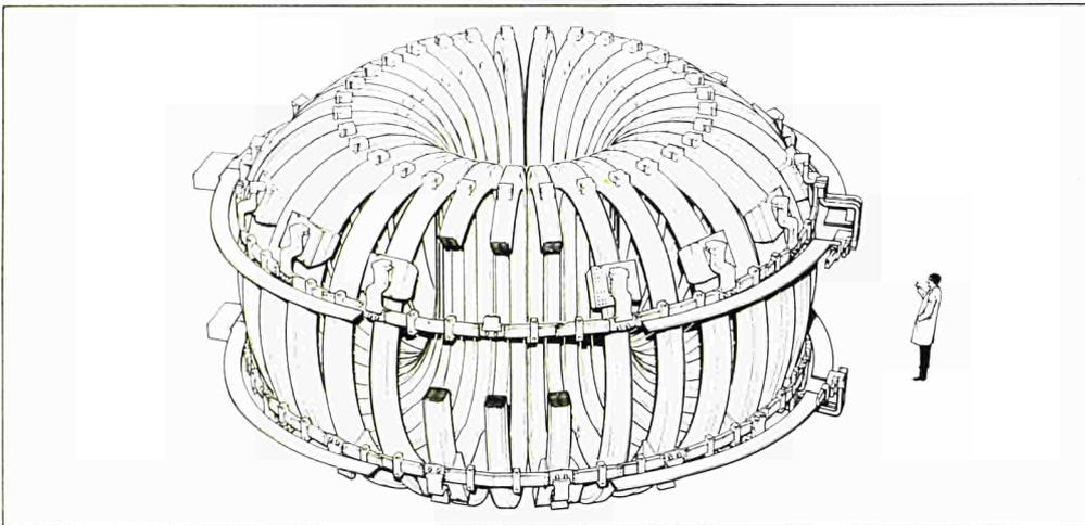
The toroidal field coil system
