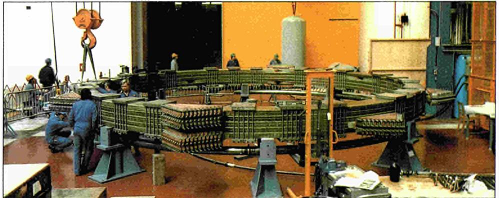
A completed outer coil with water manifolds and electrical bus bars
