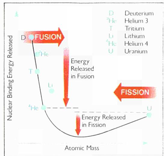
Illustration of the Energy which can be released by Nuclear Reactions
