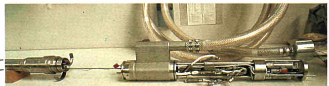
STANDARD IRRADIATION FACILITIES LOWER PORTION AND HEAD OF A RELOADABLE IN-CORE IRRADIATION CAPSULE
