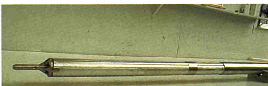
STANDARD IRRADIATION FACILITIES LOWER PORTION AND HEAD OF A RELOADABLE IN-CORE IRRADIATION CAPSULE
