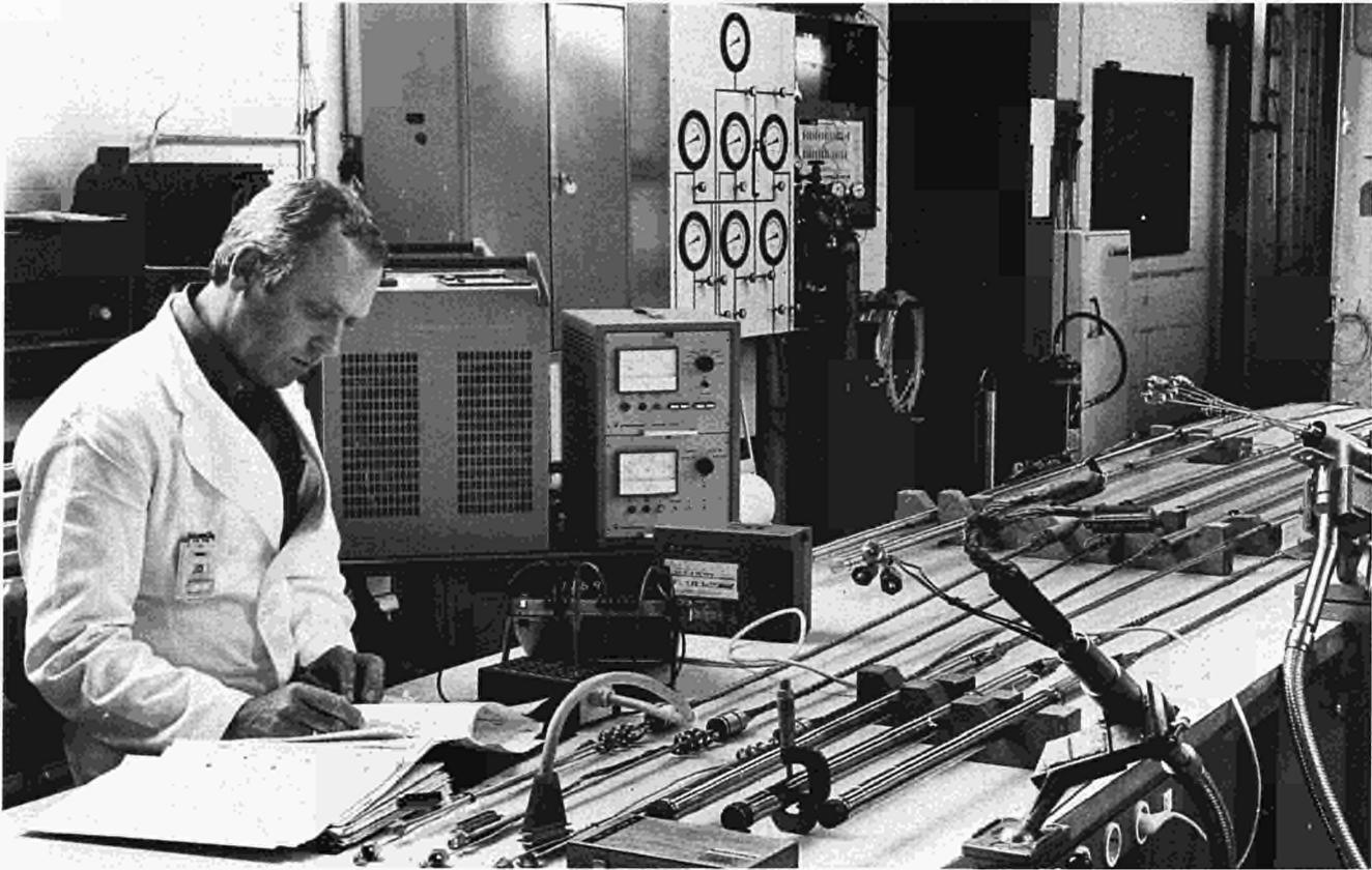
Fig. 71 Testing and commissioning of HFR irradiation devices.
