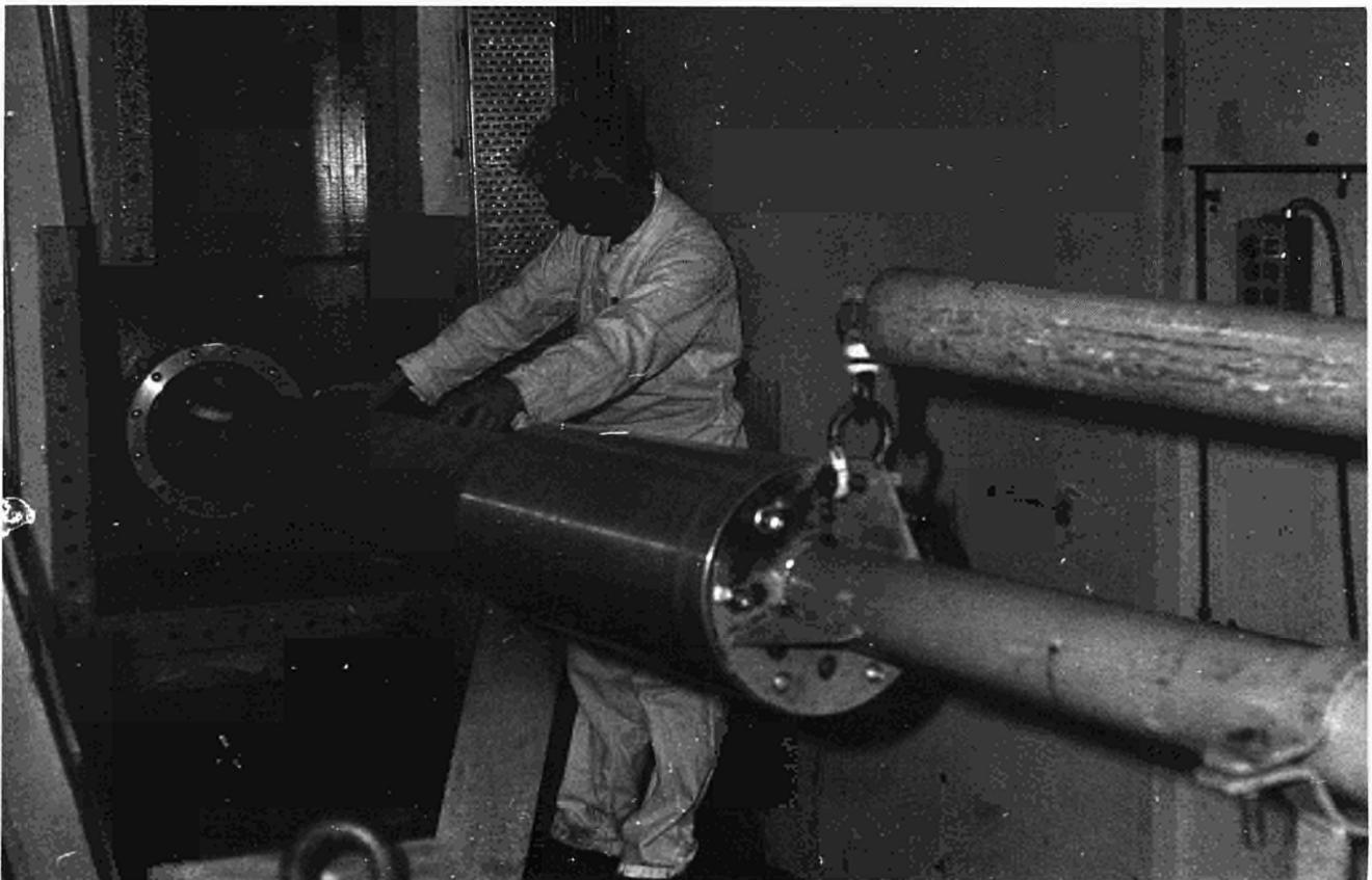
Fig. 78 Dry neutron radiography camera. Placing of the in-pile collimator in beam tube HB-8.
