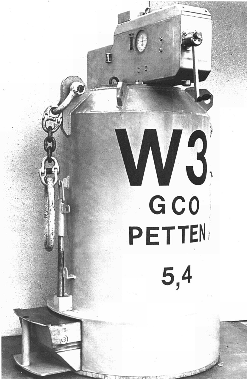
Fig. 66 New ("W3") shielded container for on-site transports.
