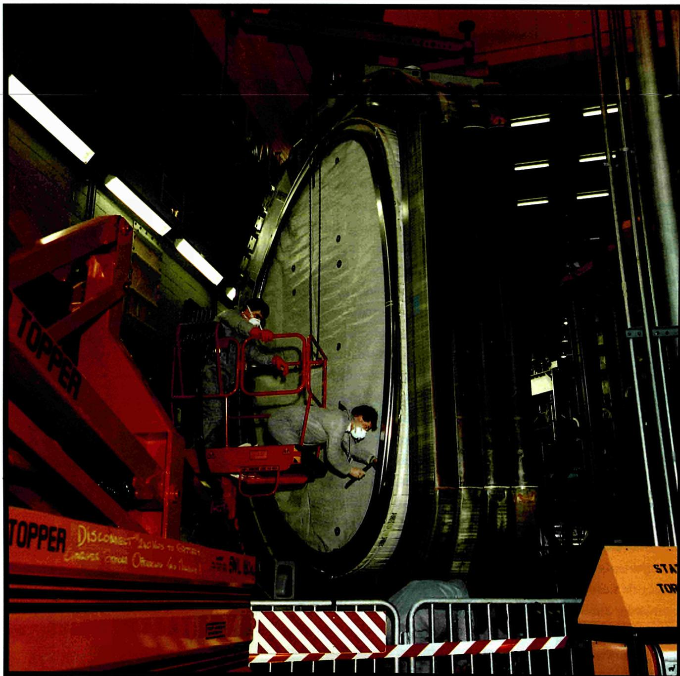
Fig.5: An octant being removed from the torus.
