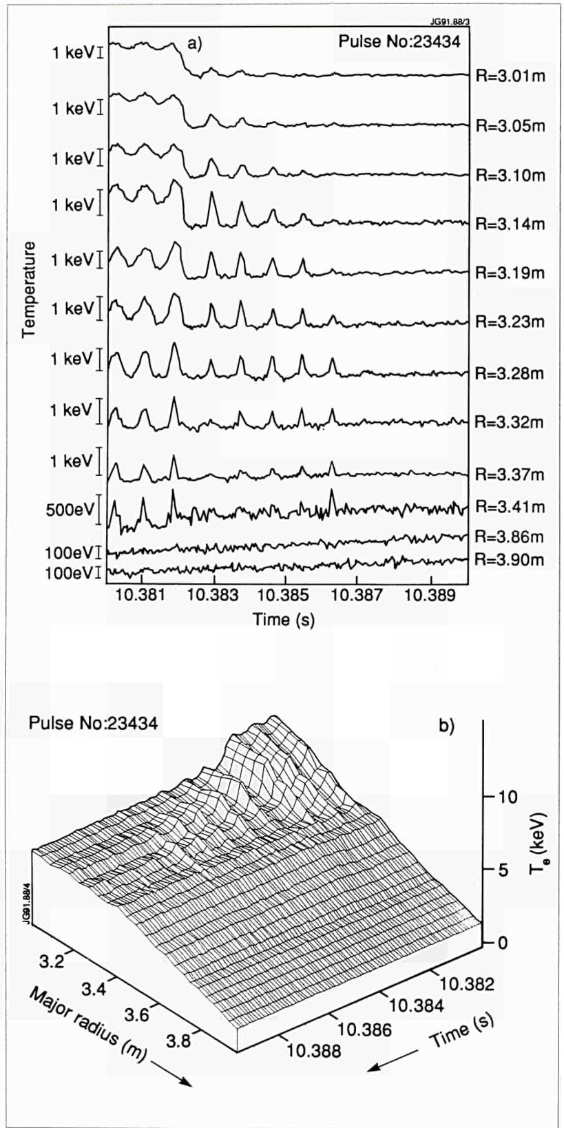
Fig.14: (a) the time evolution of the electron temperature around a sawtooth collapse, at a number of fixed radii. The signals shown are a subset of the 44 channels measured by the heterodyne radiometer. The existence of a localized MHD mode which persists through the sawtooth collapse is clearly visible; (b) data from 25 radiometer channels spanning the outer half of the plasma have been used to obtain the time evolution of the temperature profile in the same time range as part (a).
