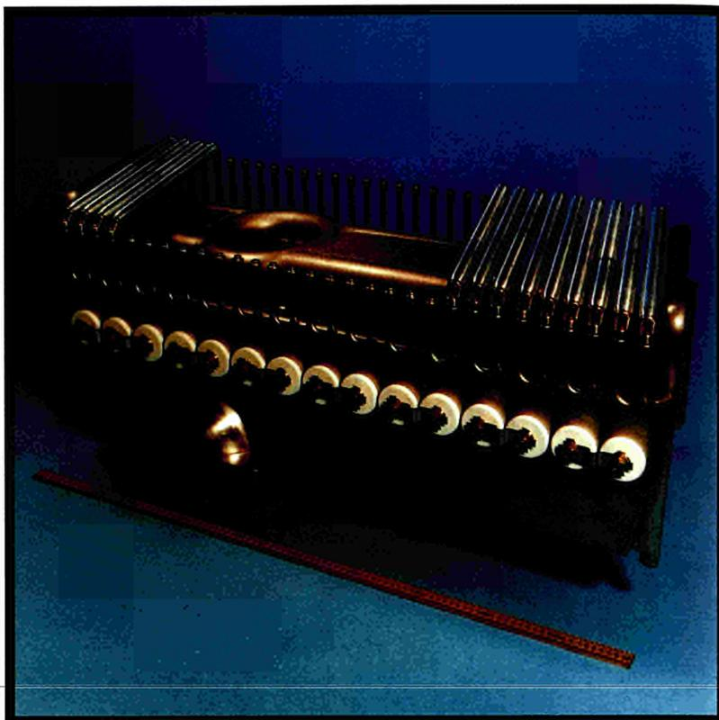
*Fig.50: The full scale model of one quadrant of the A2 antenna to be used for high power RF tests.*
