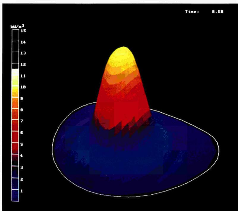
Fig.17: Typical output from the real-time tomography display taken during a plasma discharge.
