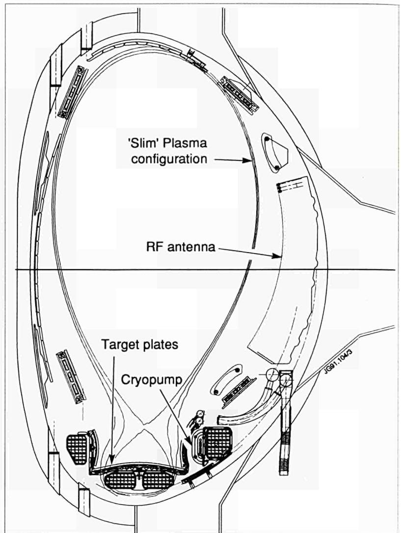
Fig.48: Configuration with so-called 'slim' plasma.
