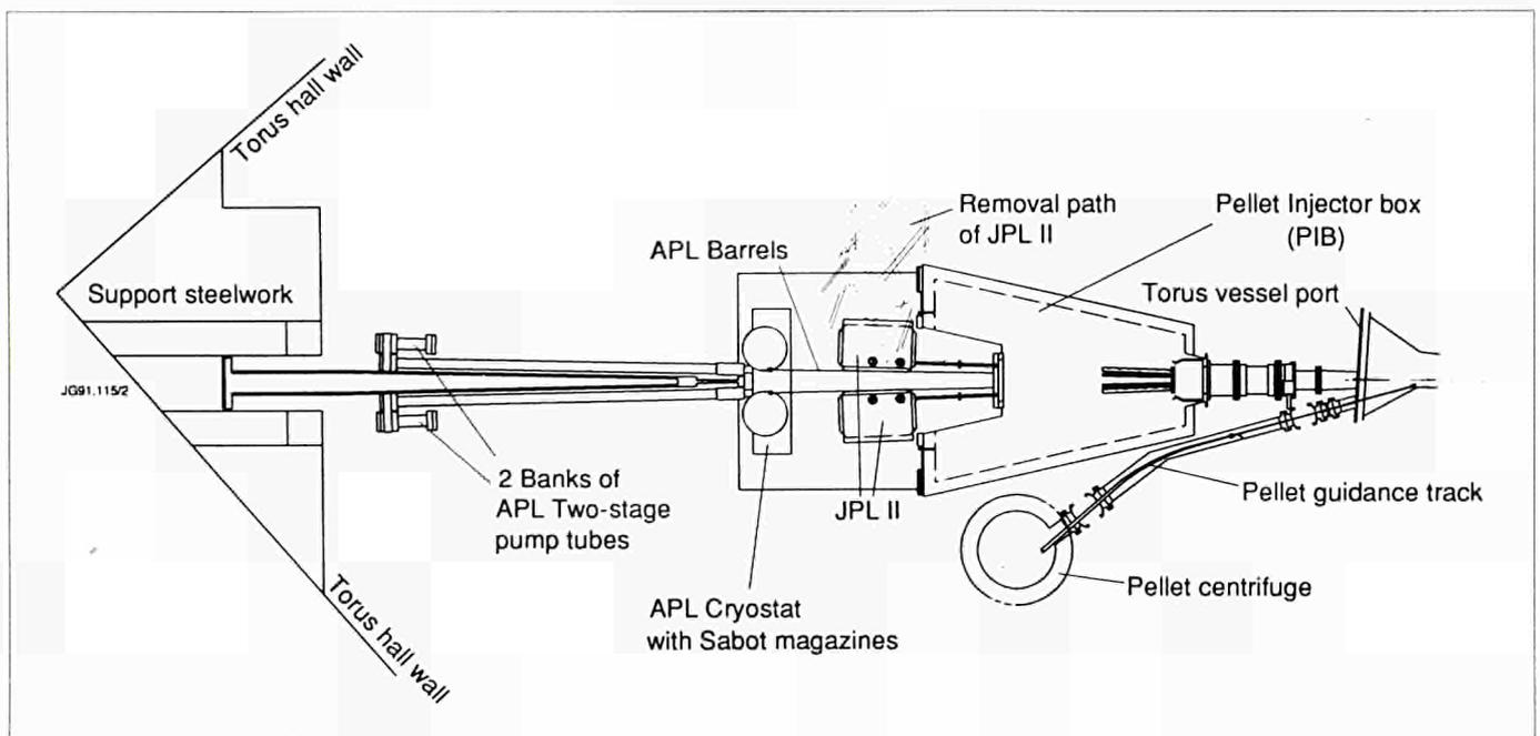
Fig.25: Conceptual view of future JET Pellet Injection (plan view).
