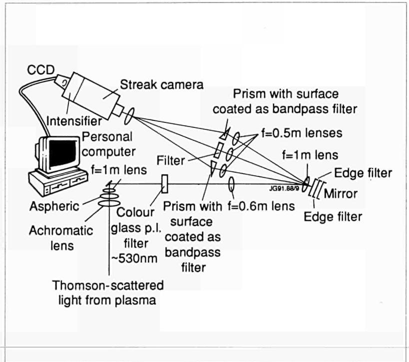
Fig.16: Schematic of the high resolution LIDAR Thomson scattering system under construction for edge measurements.
