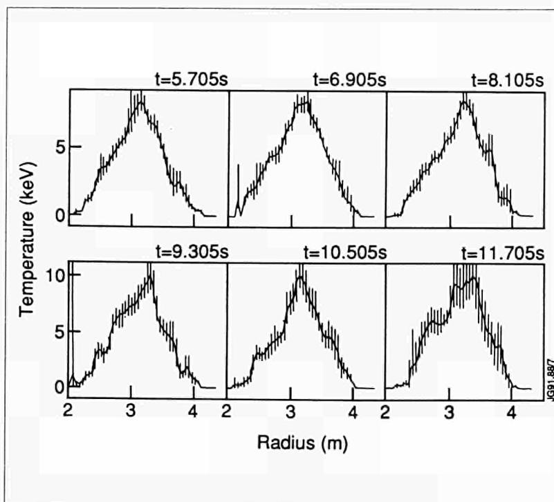
Fig. 15: The electron temperature profile measured by LIDAR Thomson scattering in the presence of severe stray light.
