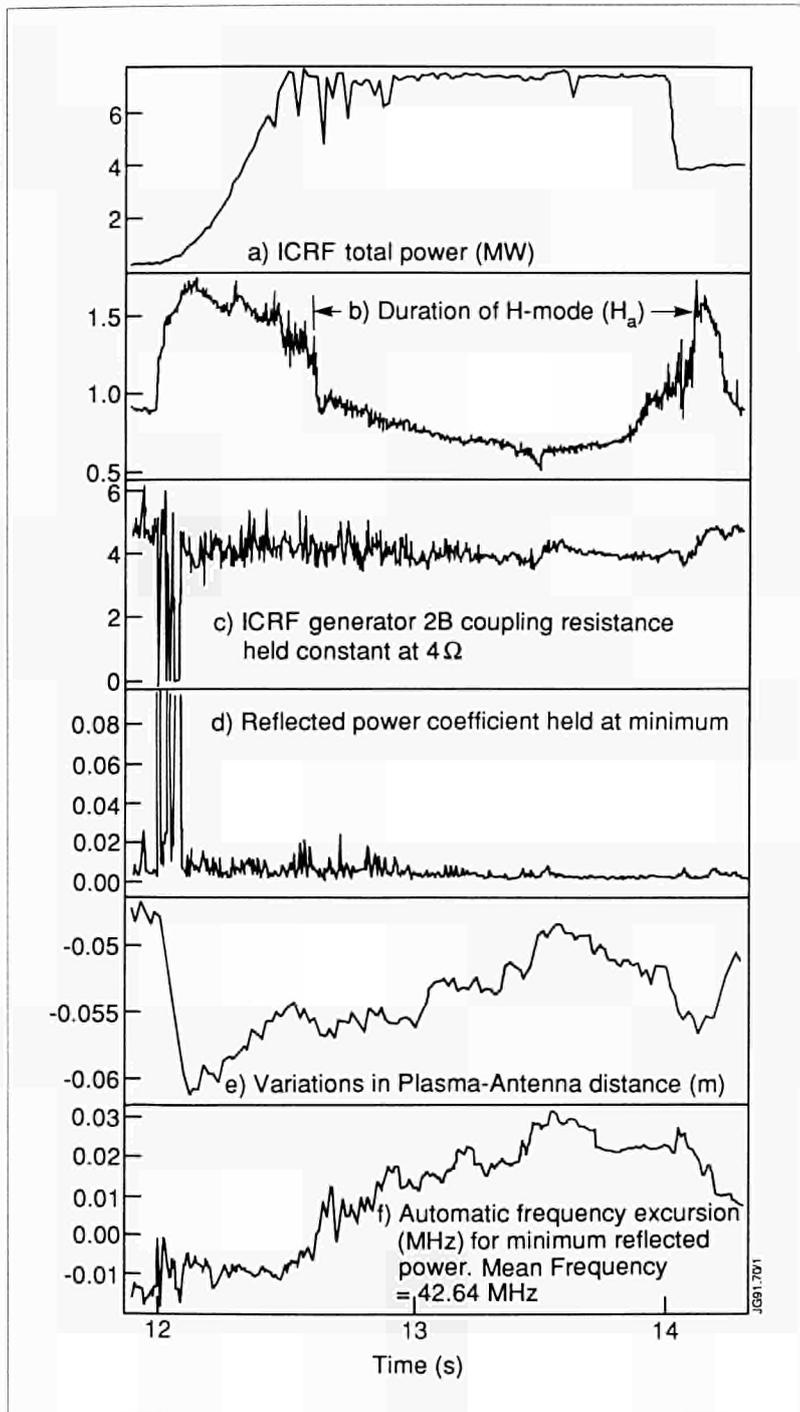
**Fig.10: Antennae coupling resistive control of plasma position during H-mode transitions in Pulse No:21906. During the RF Power pulse (a), which contains an 'H' mode (b), the coupling resistance at the antenna (c) is held constant, and the reflected power kept at a minimum (d) by the automatic control of the plasma position (e) and incremental frequency (f).**
