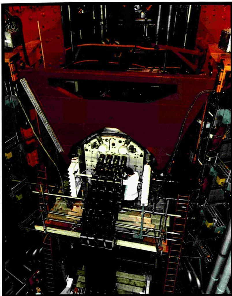
*Fig.11: An external view of the Lower Hybrid Current Drive Launcher on JET. Its vessel is supported by the large red frame. The prototype has 24 waveguides connected to the RF vacuum windows at the point of entry to the vessel.*
