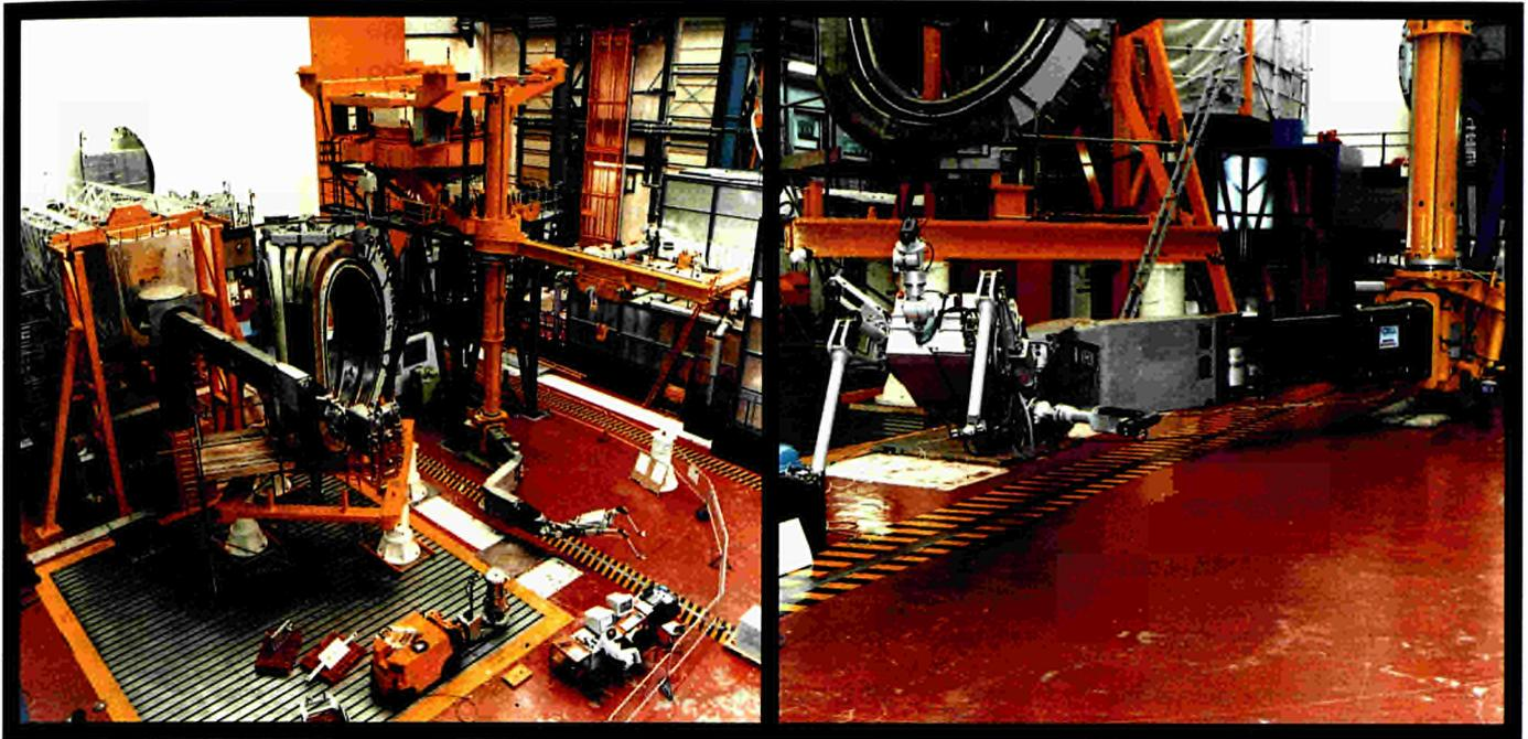
Fig.21: (a) the TARM installed on stillage in the Assembly Hall, shown with Mascot approaching a turbopump on a low level transporter for remote handling trials; (b) both TARM and Boom can reach the inside of the spare Octant for in-vessel tests.
