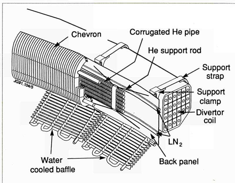
Fig.51: Divertor cryopump
