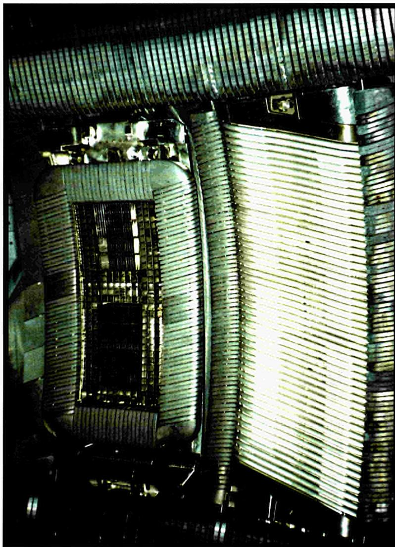
*Fig.9: View of the LHCD launcher in the torus (on the right), adjacent to one of the existing eight ICRF antennae (on the left). The upper and lower prototype launchers together with the carbon side protection tiles (similar to ICRF) can clearly be seen. The ICRF antenna conductors are just visible through the beryllium bars of the new open screen.*
