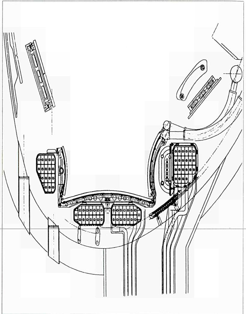
Fig.46: Details of four divertor coil arrangement.
