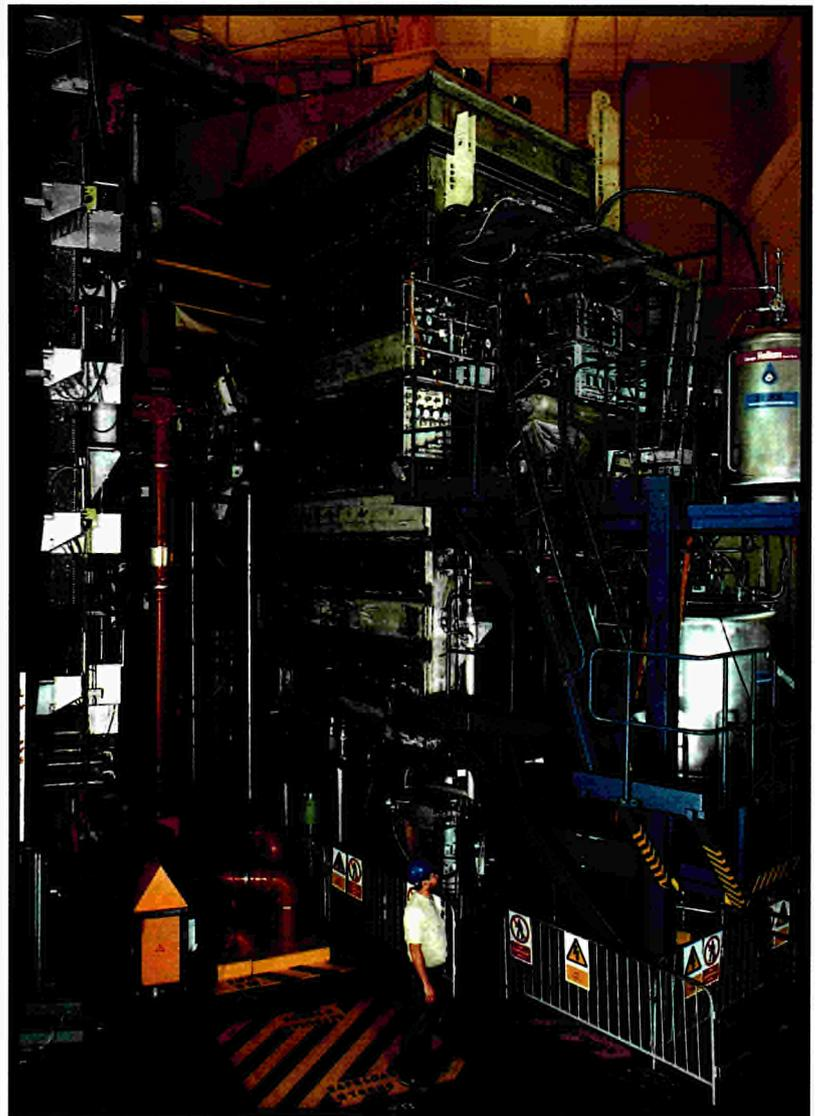
Fig.12: The multi-pellet injector on JET.
