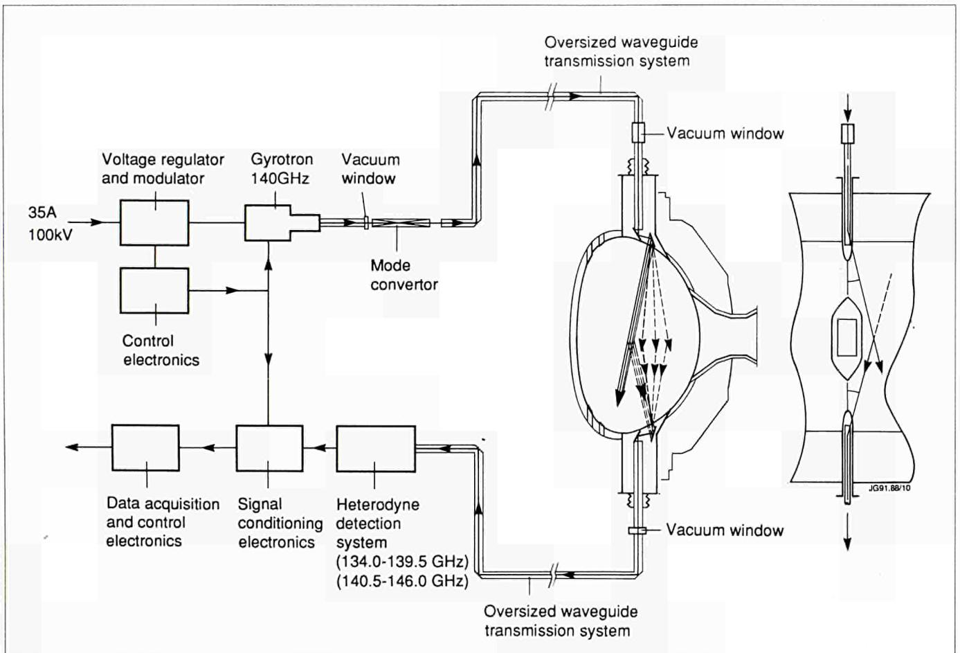
Fig.20: Schematic of collective scattering system for measuring spatial and velocity distributions of fast ions including alpha-particles.
