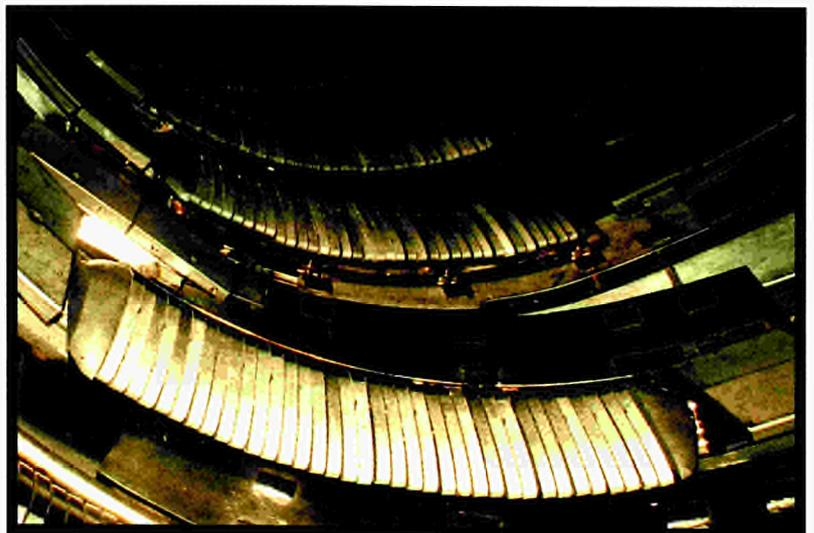
*Fig.6: Discrete beryllium X-point target plates at the bottom of the vessel.*
