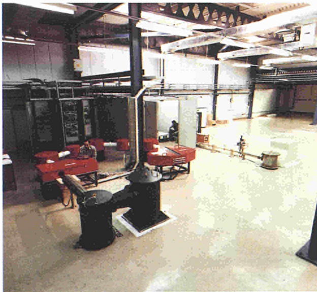
Fig. 38 The diagnostic roof laboratory showing the laser input and light collection system of the Thomson scattering diagnostic.
