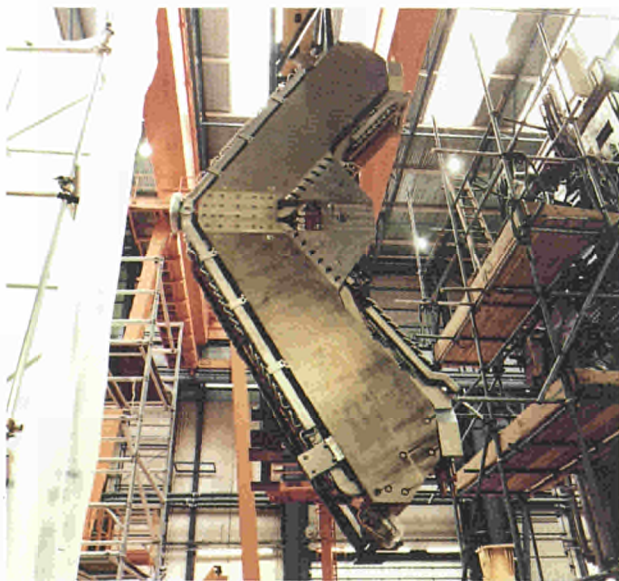
Fig. 21 Deflection magnet after installation of the internal liners and the dumps for fractional energy beams.
