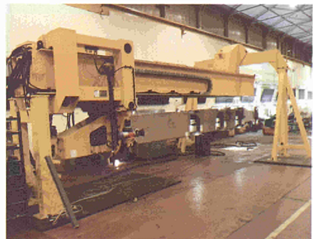
Fig.32 The articulated boom, capable of carrying a one-tonne load inside the vacuum vessel. Seen at the manufacturer's works.
