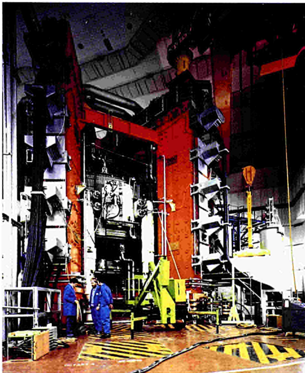
Fig.34 The provisional soft X-ray diode array at octant 4. To the right, at octant 5, the concrete tower of the Thomson scattering system.
