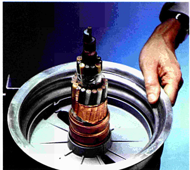
Fig.14 A section of a SF 6 -insulated high voltage transmission line for the supply of power to the neutral injectors.
