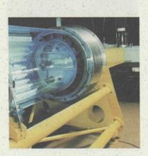
480-litre reaction chamber for simulating atmospheric photochemistry.
