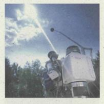
Precision solar energy measurements with a cavity radiometer.
