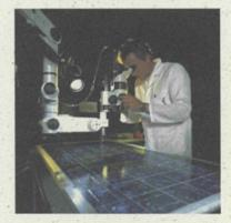
Inspection of PV Modules after 20-year lifetime simulation.
