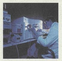
The discovery, at the Environment Institute in 1998, of a new class of chemical compounds has significantly improved our understanding of smog formation. M. Duane is preparing the HPLC-MS<sup>n</sup> for smog analysis.
