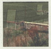
Static rooms used to measure methane flows in the Vercelli experimental site (collaboration with University of Edinburgh).
