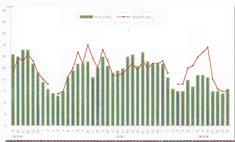
Fig. 73 - Comparison of hourly \text{NO}_2 concentrations at the JRC and the station shown in Fig. 72.
