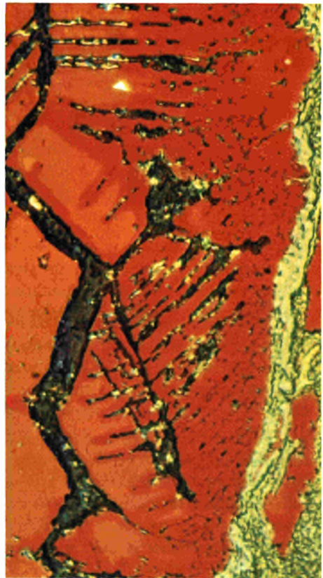
Micrographs of samples of corroded steel cladding which illustrate the use of interference films to enhance phase differentiation
