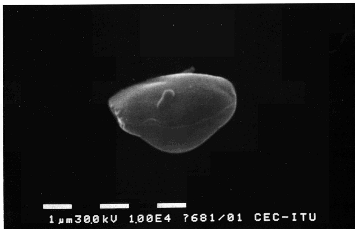
Fig. 7.2 Particle ablated from \text{UO}_2 pellet
