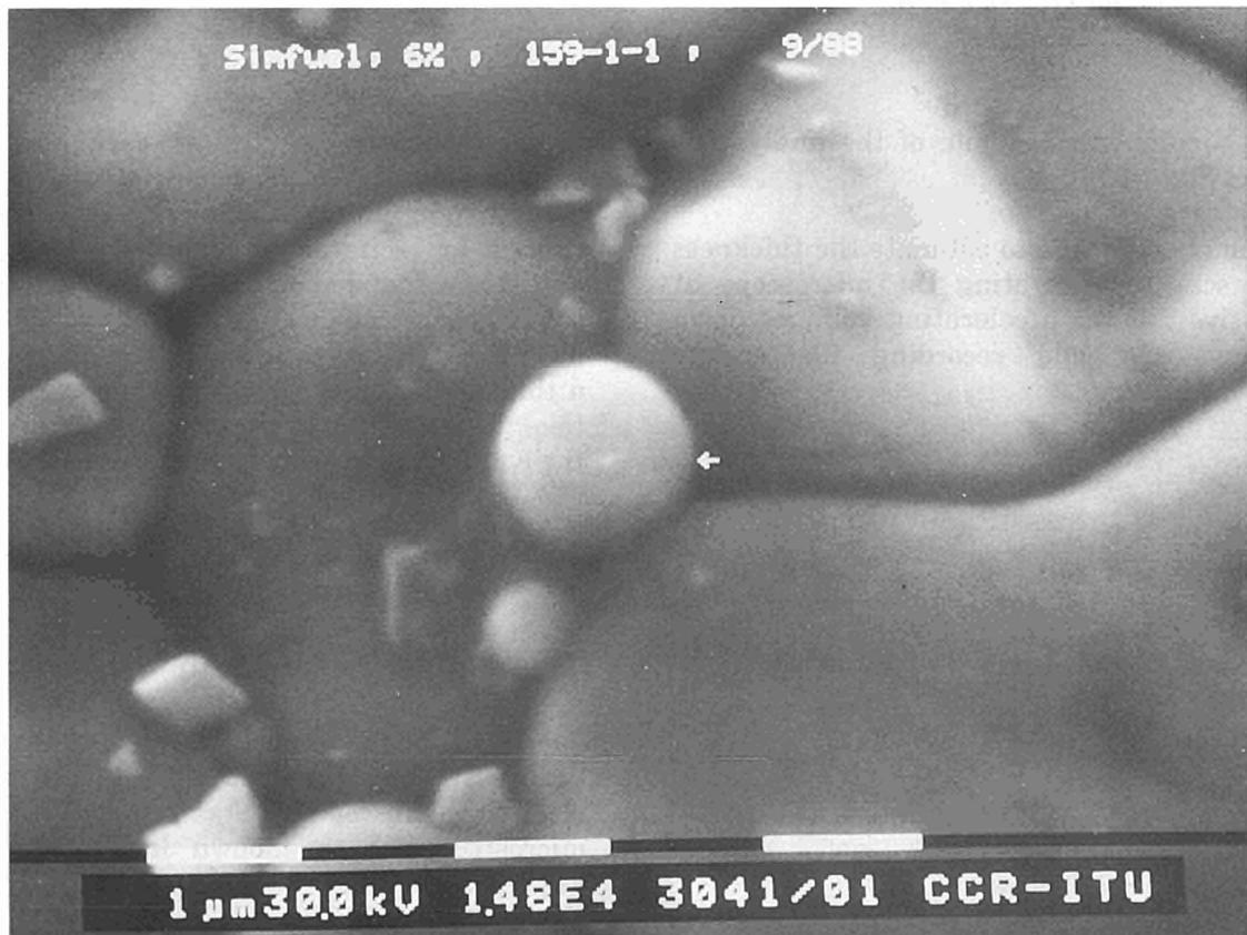
Fig. 1.20 High magnification micrograph of part of the same area showing the spherical Mo/Ru precipitates.
