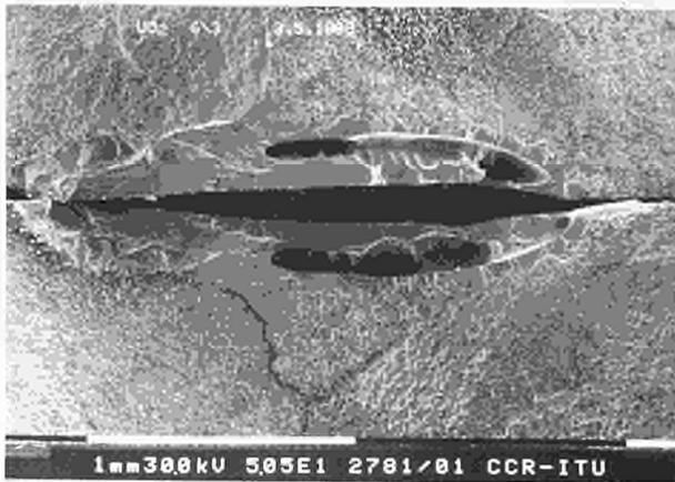
Fig. 4.7 SEM Photograph of the cleaving surfaces along the radial crack, sample of Figs. 4.2-4.4. The crevasses are caused by the 11% reduction in volume on solidification.
