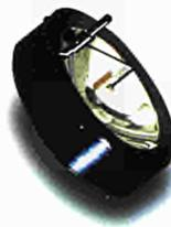
New developments were conducted on the Syclop detector (heat flux sensor based detector) in order to trigger a digital camera when an intrusion is monitored. The first prototypes gave very good results.
