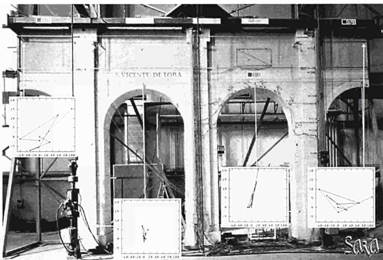
Figure 2.9: Photogrammetry used to monitor a model of the Portuguese Monastery São Vicente de Fora during PSD testing: During the seismic experiment the actuator connected to the upper right part of the building pushes and pulls the building until structural damage occurs.
