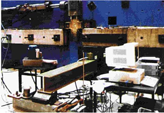
Figure 2.12: Determination of vibrational shapes in flat composite plates using embedded optical sensor networks. Peaks in the frequency spectra of embedded sensors, as shown for one such sensor in the data curve, allow interpretation of how the plates vibrate under given loads. The data can be verified by measurements of Pulsed Electronic Speckle Pattern Interferometry.
