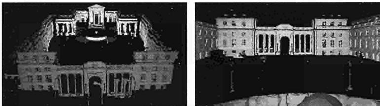
Figure 1.20: 3D Reconstruction of the "Cour d'Honneur" of the French National Assembly – the figure shows two snapshots of the final 3D reconstructed model. The model is textured with the infrared laser reflectance data. The internal courtyard is about 80 m per 50 m.
