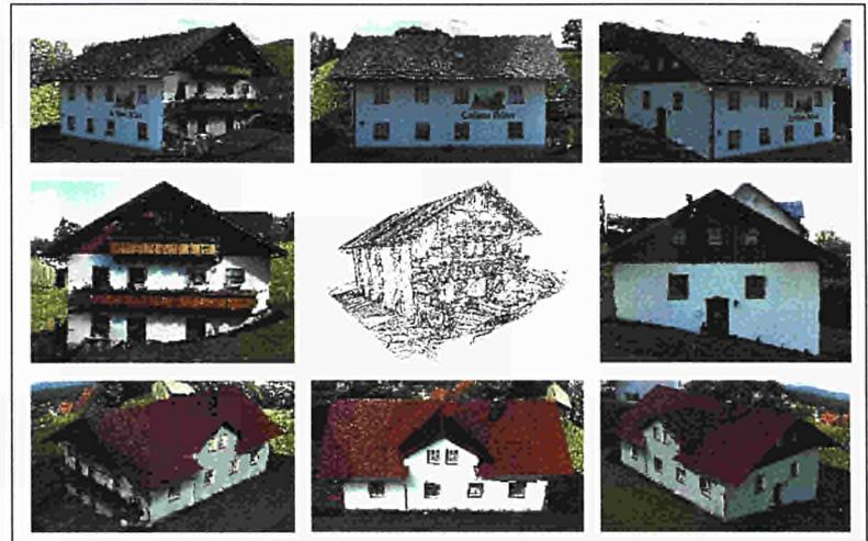
Figure 1.22: 3D Reconstruction of a Bavarian farmhouse - several snapshots of the 3D reconstructed model.
