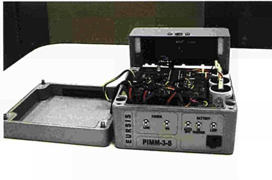
Figure 3.2: A prototype pressure instrument module was designed for accurate in-field measurement of liquid mass and volume in tanks (PIMM).
